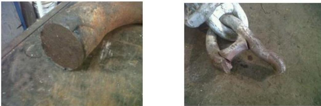
Fig. 1 The Anchor Chain Failure of Gryphon Alpha FPSO (Finucane 2012)
