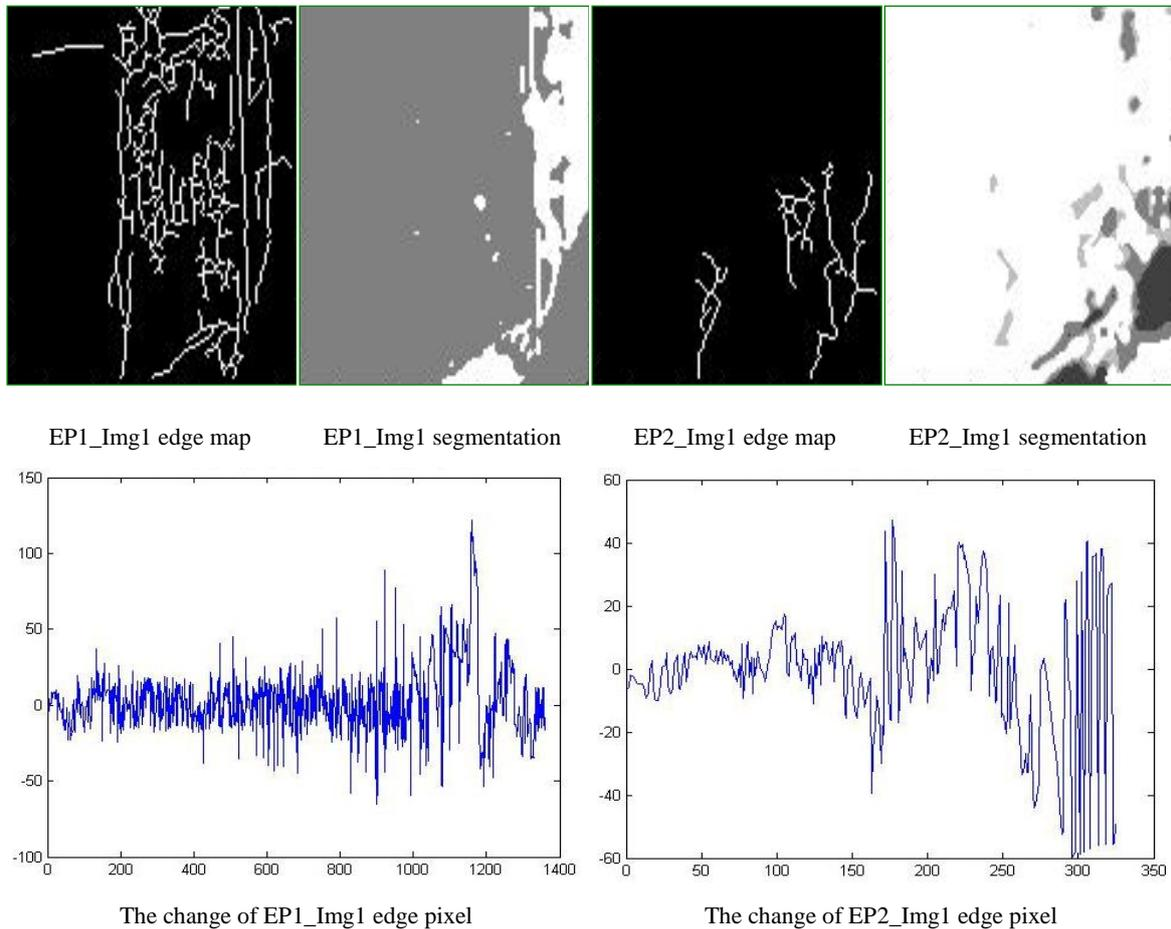
Fig. 11 The region segmentation analysis of underwater image by the EP model
