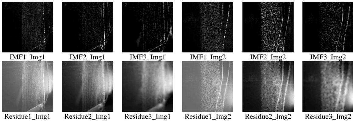
Fig. 4 Test image 1 and test image 2 are decomposed into three IMFs and three Residues
