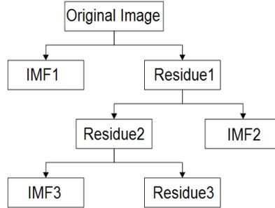
Fig. 3 Decomposition diagram of BEMD
