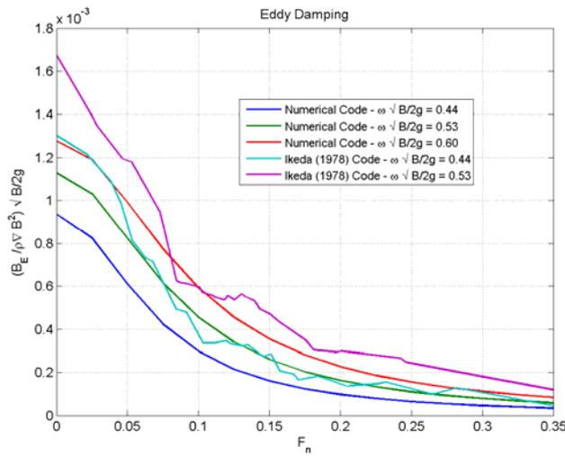
Fig. 9 Forward Speed Eddy Damping for Series 60 Hull
