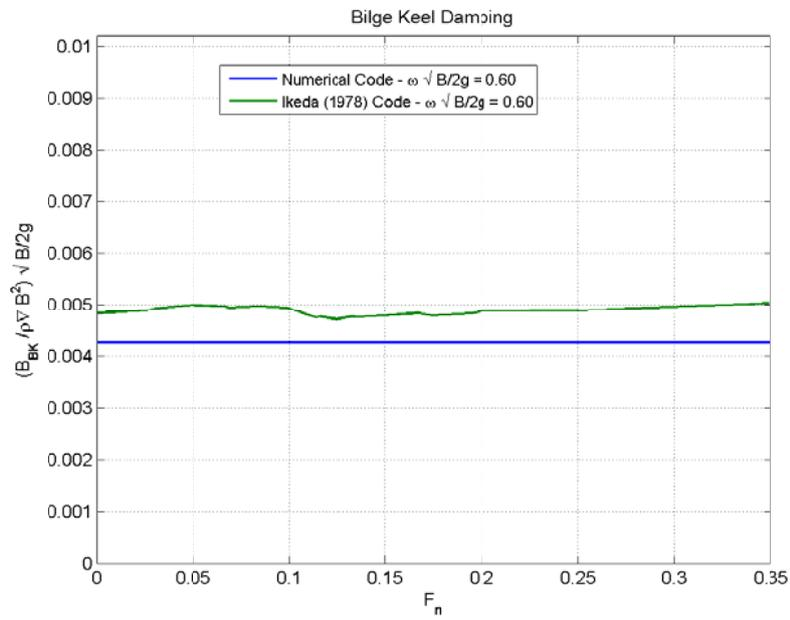
Fig. 11 Bilge Keel Damping for Series 60 Hull in Forward Speed
