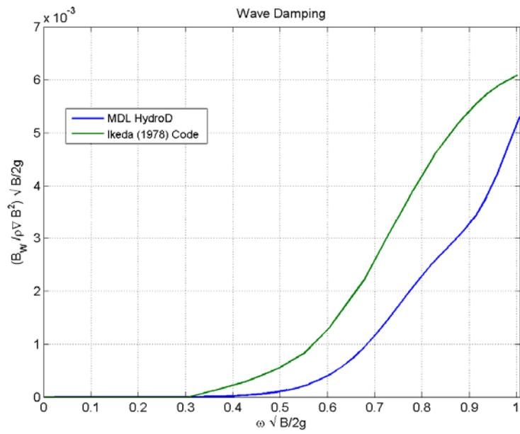
Fig. 3 Zero Speed Wave Damping for Series 60 Hull
