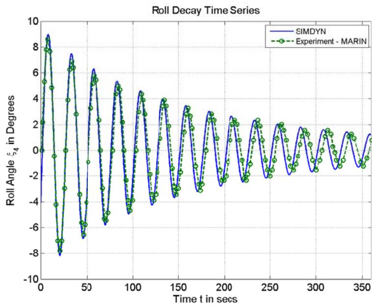
Fig. 12 Roll Decay Time Series for APL China
