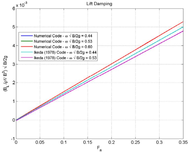
Fig. 7 Lift Damping for Series 60 Hull
