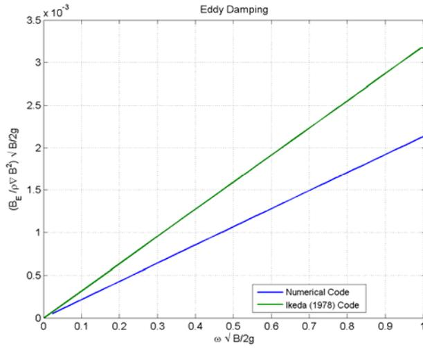
Fig. 8 Zero Speed Eddy Damping for Series 60 Hull
