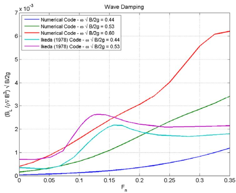
Fig. 4 Forward Speed Wave Damping
