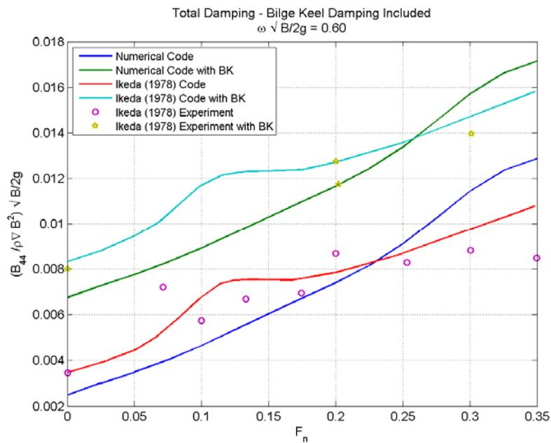
Fig. 2 Forward Speed Total Roll Damping for Series 60 Hull
