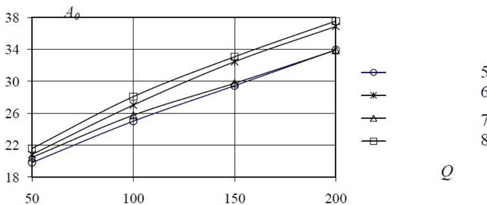
Fig. 2 Variation of cross-sectional area  $A_0$  with load  $Q$
