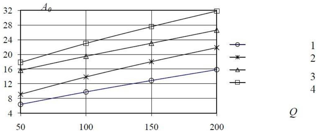
Fig. 1 Variation of cross-sectional area  $A_0$  with load  $Q$
