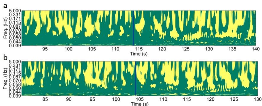
Fig. 12 Angle of cross wavelet transform with crest period 0.791s (a) and 0.632s (b)
