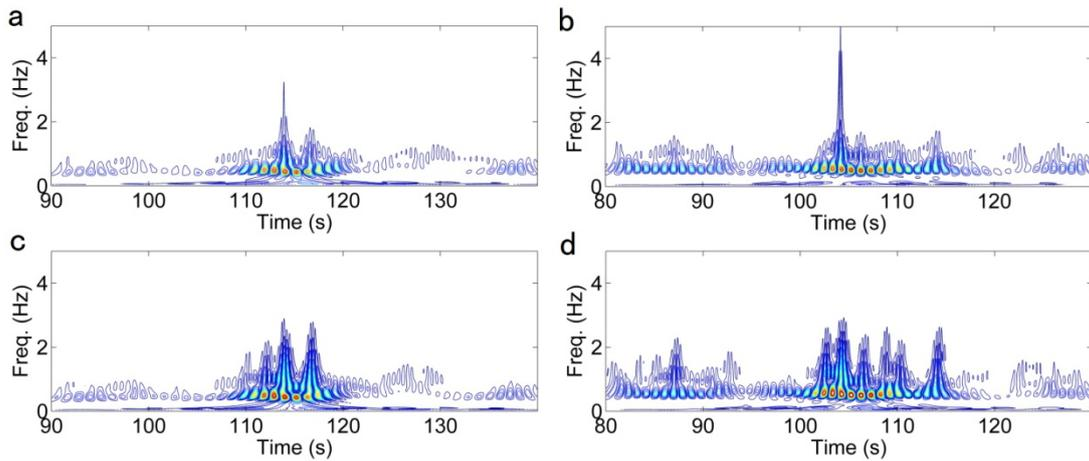
Fig. 10 Wavelet spectra of undisturbed waves (a, b) and wave run-ups (c, d). ((a, c) crest period 0.791s; (b, d) crest period 0.632s)
