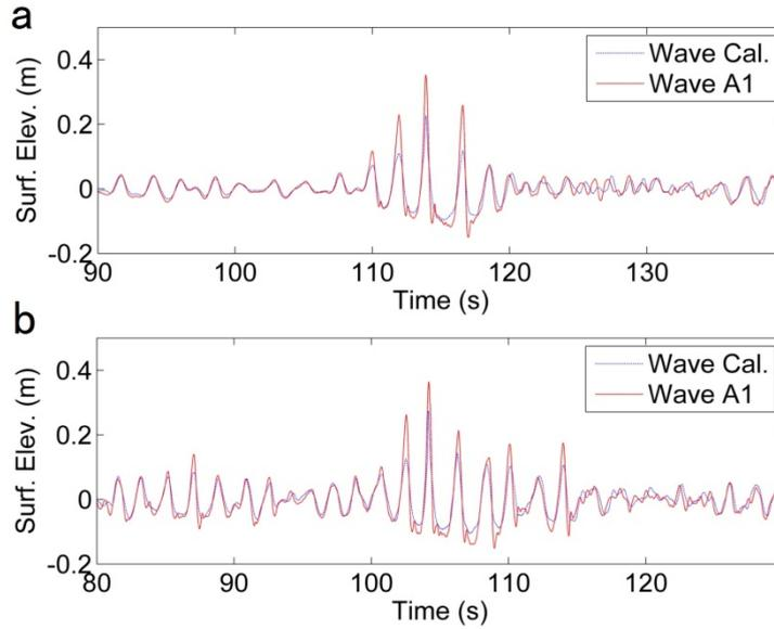
Fig. 8 Calibrated focused waves and wave run-ups at A1 of crest period 0.791s (a) and 0.632s (b)
