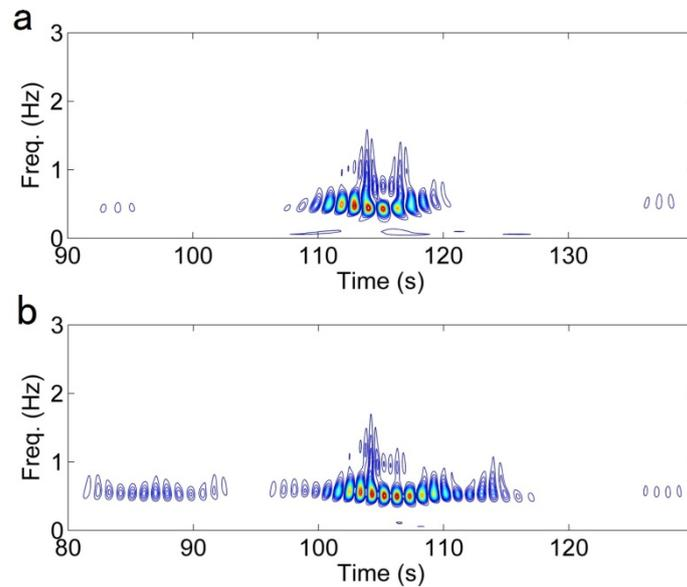
Fig. 11 Cross wavelet spectra with crest period 0.791s (a) and 0.632s (b)
