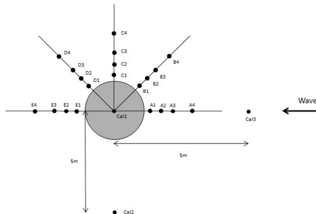
Fig. 2 Locations of wave gauges
