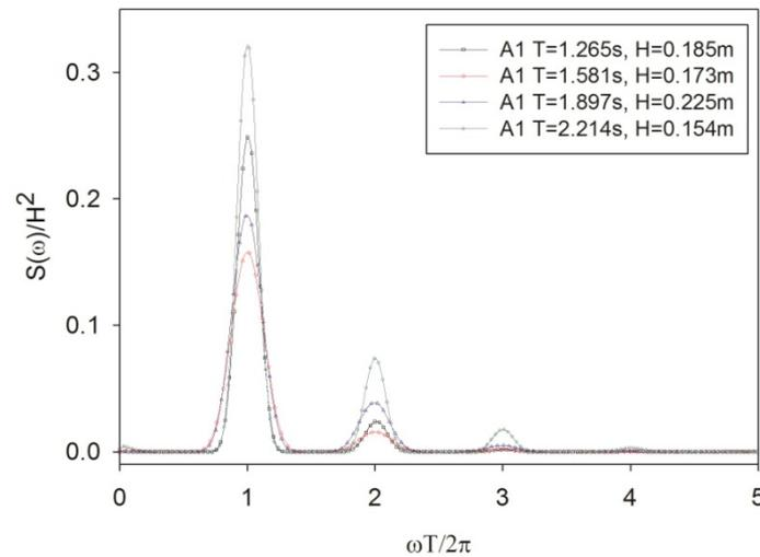
Fig. 6 Normalized spectra of wave run-up at location A1
