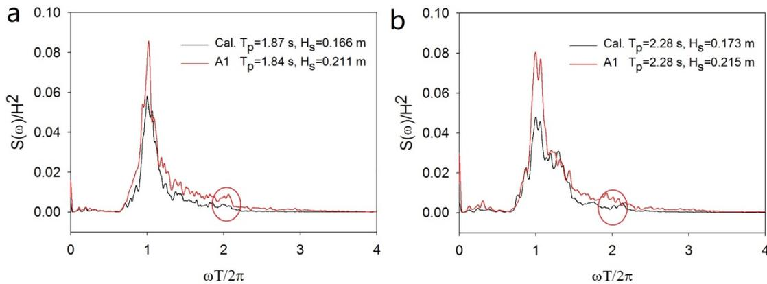
Fig. 7 Normalized spectra of undisturbed waves and wave run-ups
