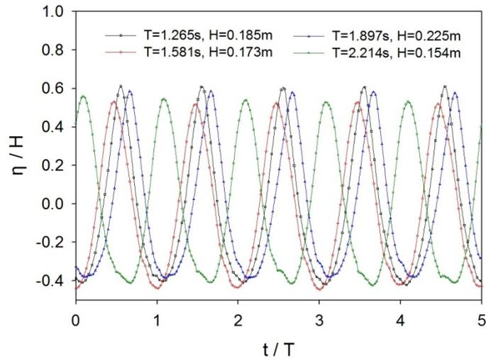
Fig. 4 Normalized time series of undisturbed incident waves
