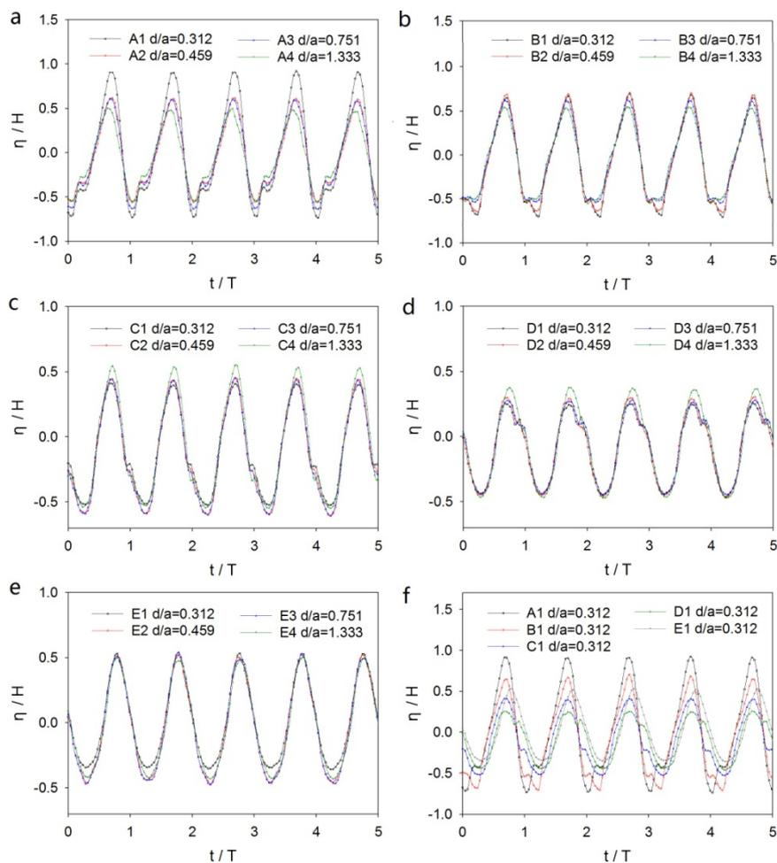
Fig. 3 Normalized wave elevations around the cylinder ( $T=1.265$  s,  $H=0.185$  m)
