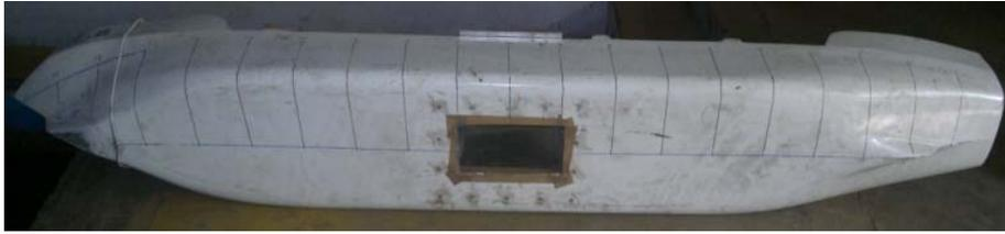
Fig. 4 Bottom view of ship model with moonpool
