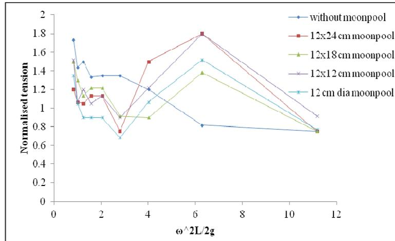
Fig. 13 Mooring line normalized tension for head on side
