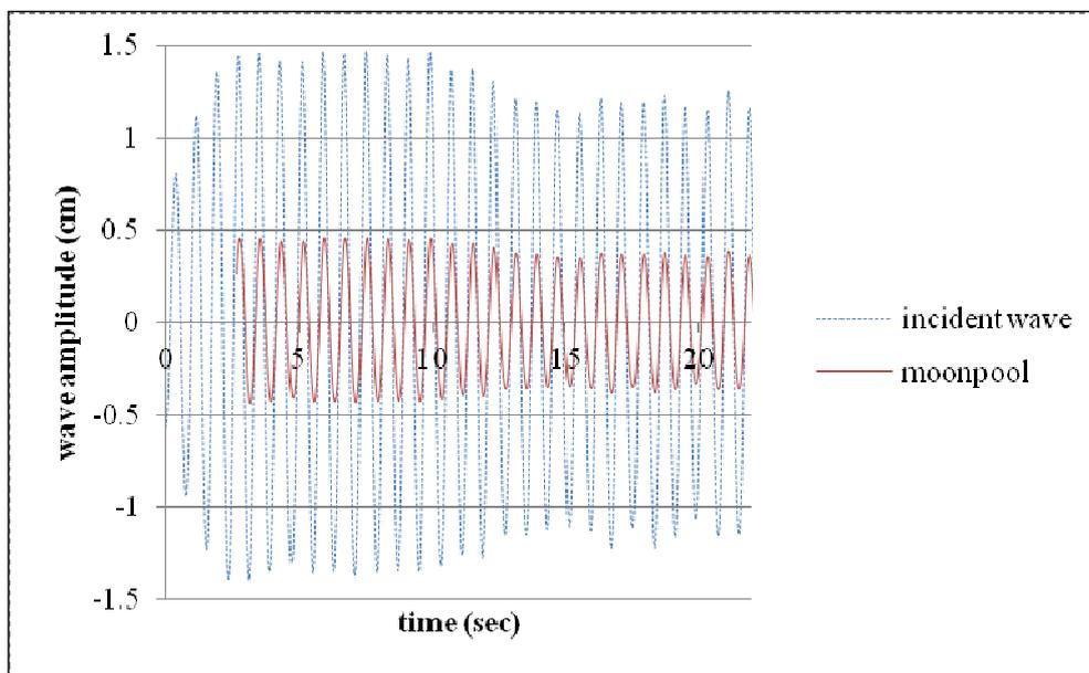
Fig. 9 Incident wave and moonpool water column oscillation for 3cm wave height
