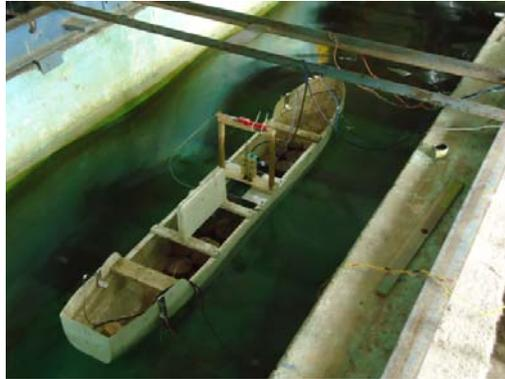
Fig. 6 Experimental setup in wave flume
