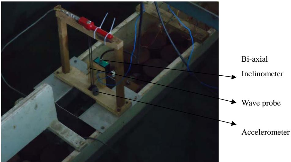
Fig. 7 Ship model with instruments for measurement
