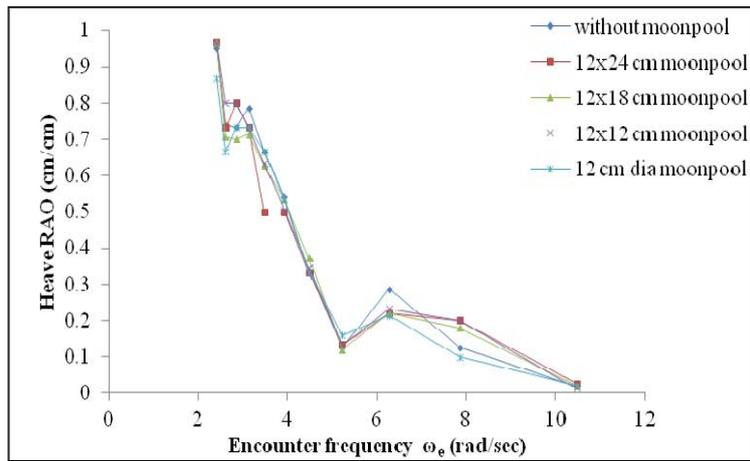
Fig. 10 Heave RAO for different shapes of the moonpool for 3 cm wave height
