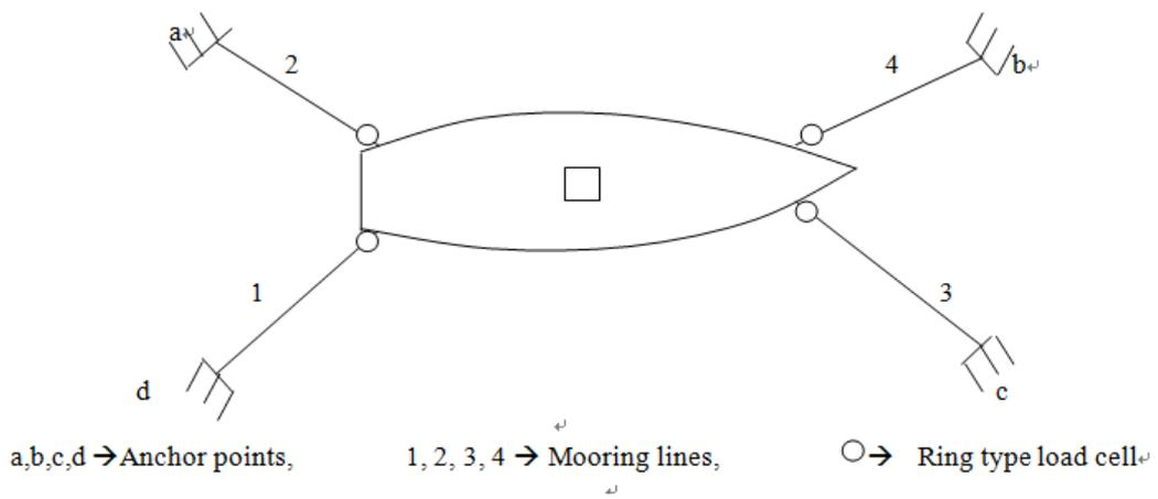
Fig. 5 (a) Plan view of model in the experimental setup
