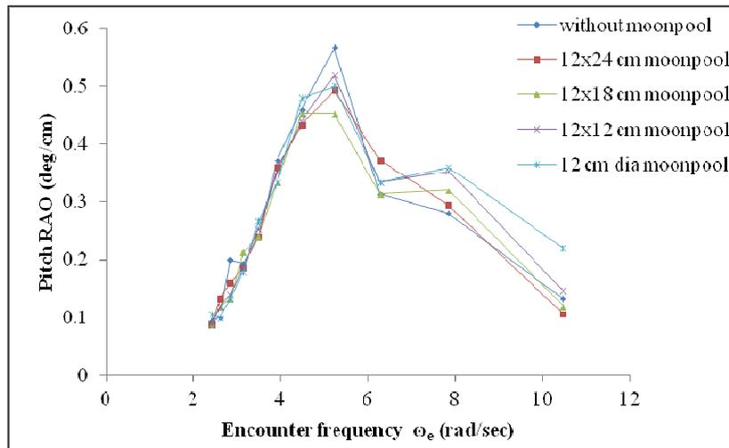
Fig. 12 Pitch RAO with different moonpool shapes for 3cm wave height
