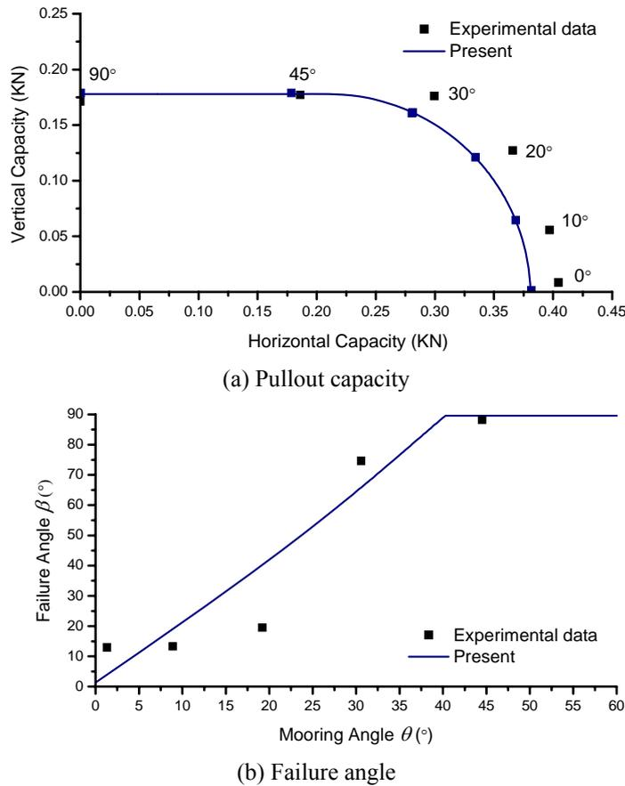
Fig. 5 Comparison with model tests
