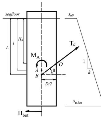
Fig. 6 Analytical method for predicting the optimal attachment point
