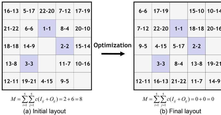
Fig. 17 Block layout of the block stock yard of 5 × 5 before and after optimization using the proposed method
