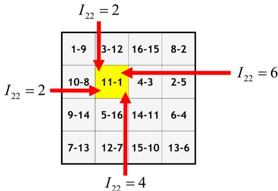
Fig. 9 Example of calculating the relocation cost for inserting ‘11-1’ block in the block stockyard
