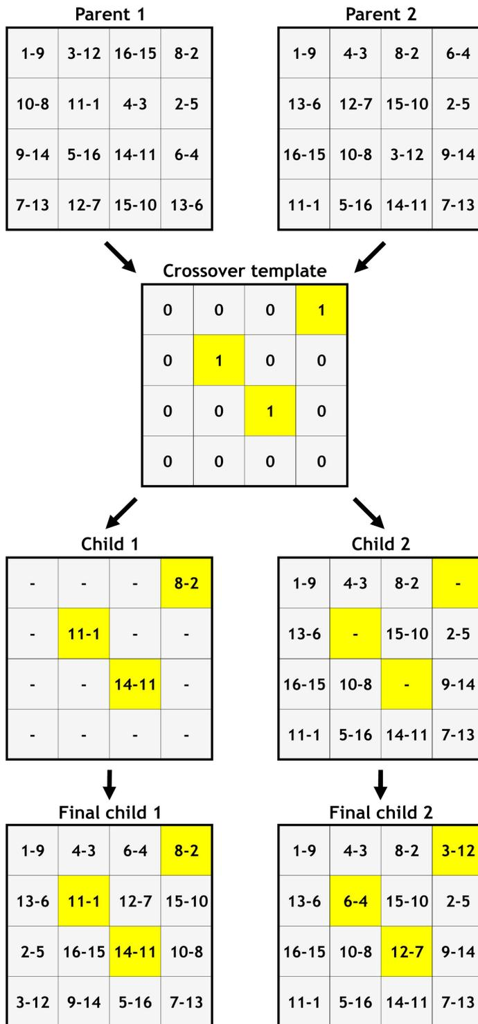
Fig. 13 Example of the uniform order-based crossover operation
