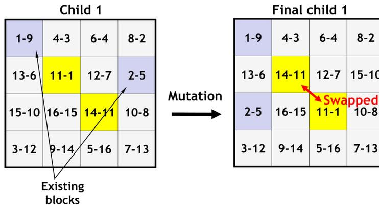
Fig. 15 Example of the mutation operation
