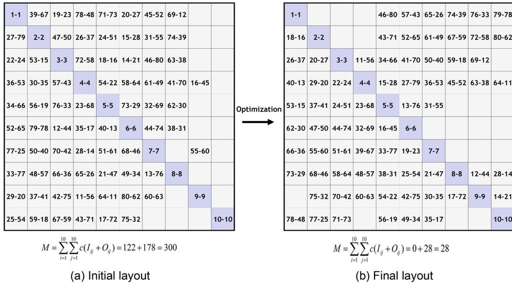
Fig. 18 Block layout of the block stock yard of 10 × 10 before and after optimization using the proposed method
