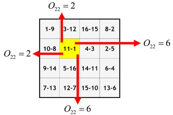
Fig. 10 Example of calculating the relocation cost for releasing the ‘11-1’ block from the block stockyard
