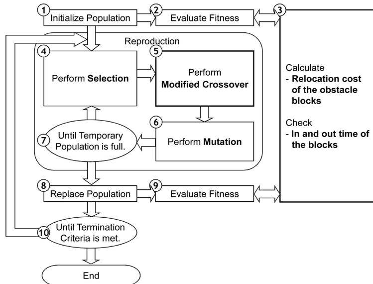
Fig. 7 Scheme of the proposed method for the block layout
