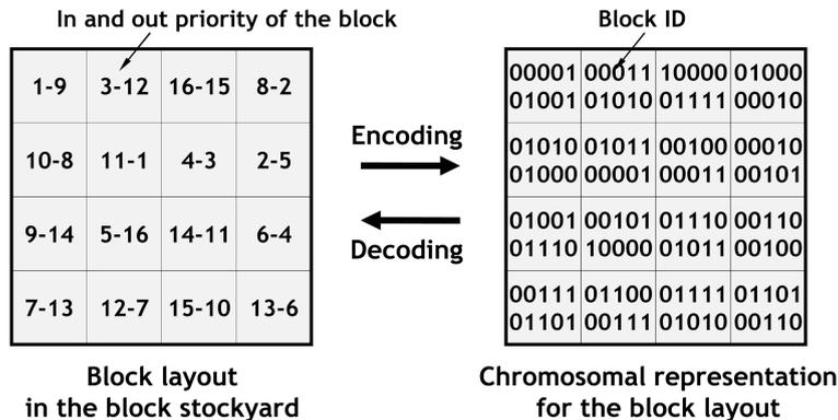
Fig. 8 Example of the block layout and the corresponding representation of the chromosome
