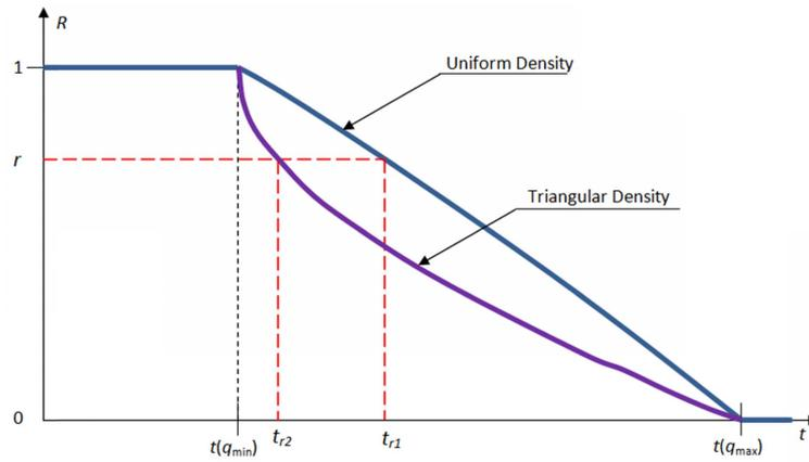
Fig. 5 Reliability of the structure versus time
