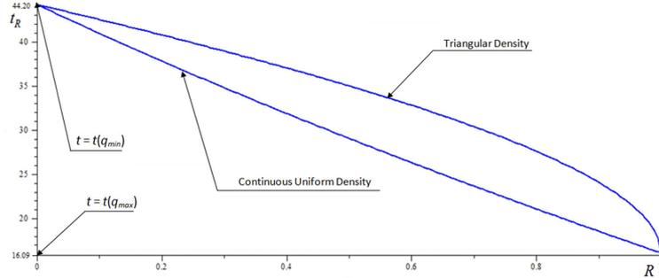
Fig. 4 Variation of time instant  $t$  as a function of reliability  $R$  in the range  $q_{min} \leq q \leq q_{max}$
