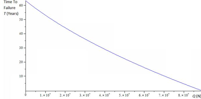
Fig. 1 Durability of the bar in years versus load  $Q$
