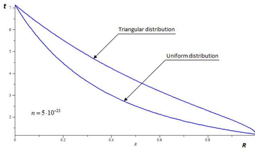
Fig. 9 Variation of time instant  $t$  as a function of reliability  $R$  in the range  $q_{min} \leq q \leq q_{max}$  for  $n = 5 \cdot 10^{-25}$
