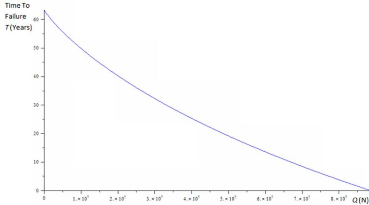
Fig. 13 Durability of the bar in years versus load  $Q$
