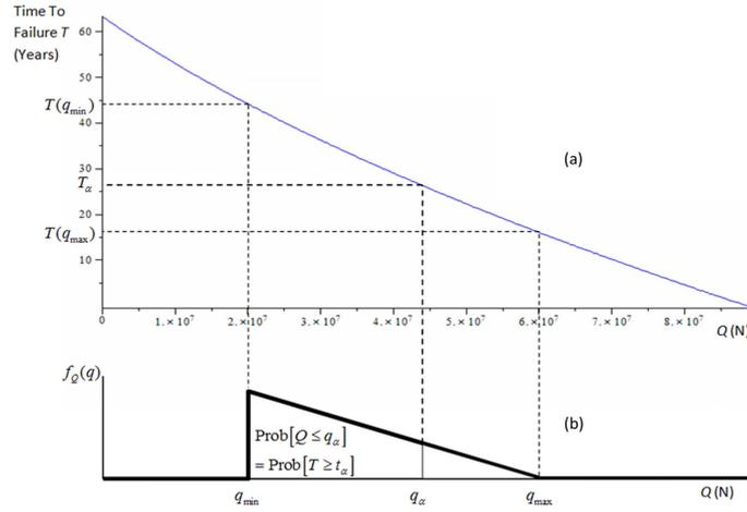
Fig. 3 (a) Time to failure  $T$  versus load  $Q$  and (b) probability density function of  $Q$
