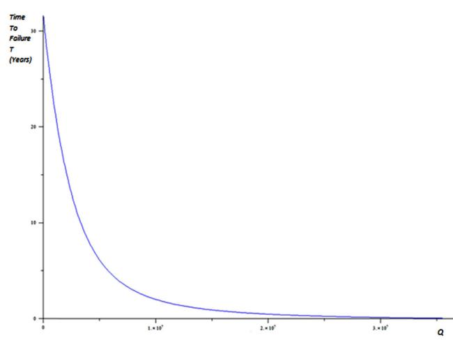
Fig. 6 Time to failure  $T$  versus load  $Q$
