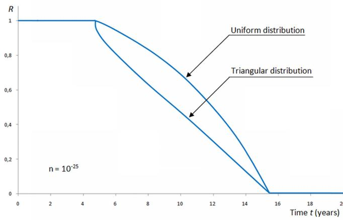
Fig. 11 Reliability of the structure versus time for  $n = 5 \cdot 10^{-25}$
