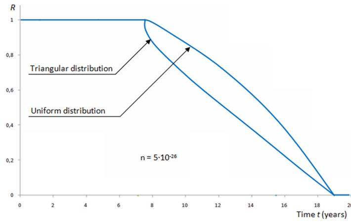
Fig. 10 Reliability of the structure versus time for  $n = 5 \cdot 10^{-26}$
