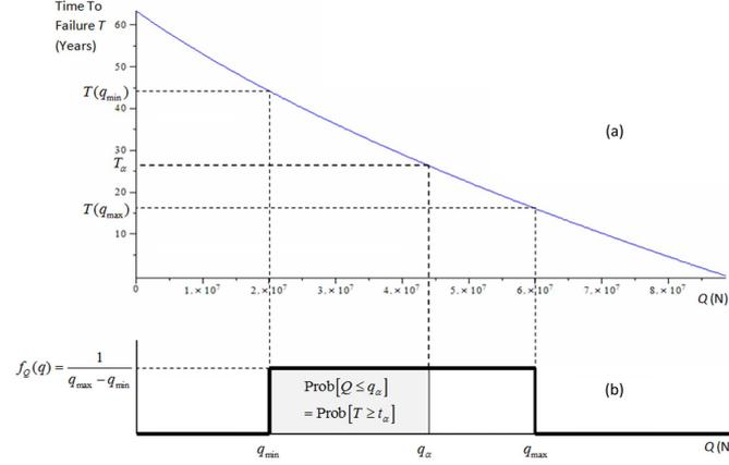
Fig. 2 (a) Time to failure  $t$  versus load  $Q$  and (b) probability density function of  $Q$
