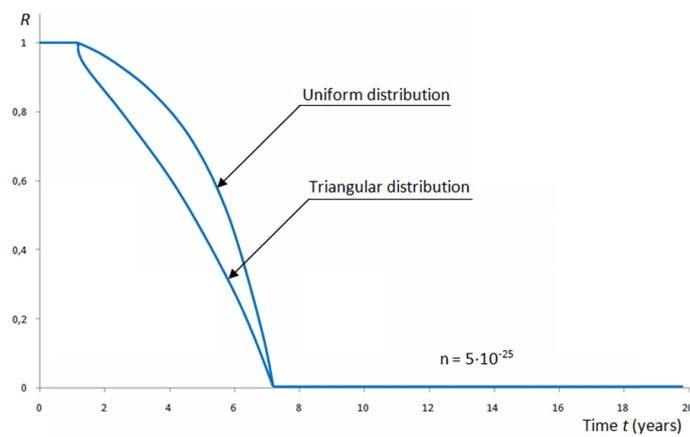
Fig. 12 Reliability of the structure versus time for  $n = 5 \cdot 10^{-25}$
