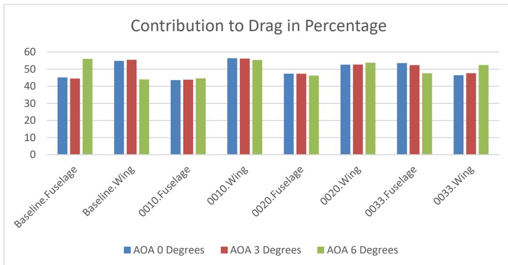
Fig. 14 Contribution of fuselage and wing to the drag of the glider (in percentage)
