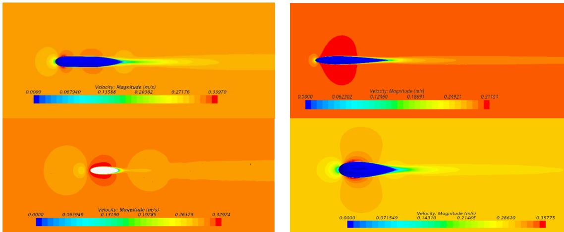
Fig. 19 Velocity scalars for the four gliders at velocity 0.3 m/s and  $\alpha=0^\circ$
