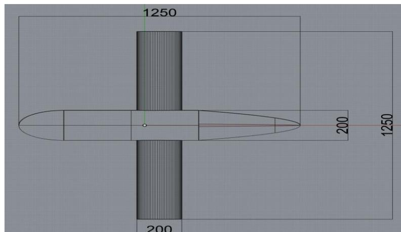
Fig. 7 Candidate baseline underwater glider CAD model. The dimensions of the glider are shown in mm
