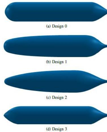
Fig. 4 Hull forms for AUGs evaluated for drag performance (Lidtke *et al.* 2016)
