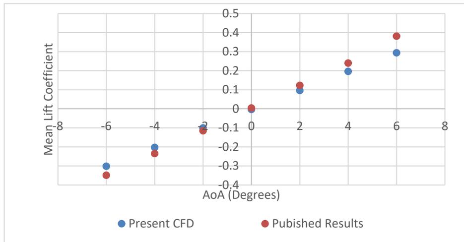
Fig. 6 Mean Lift Coefficient Results for Validation (Published results refer to the experimental results of Arima *et al.* (2008))
