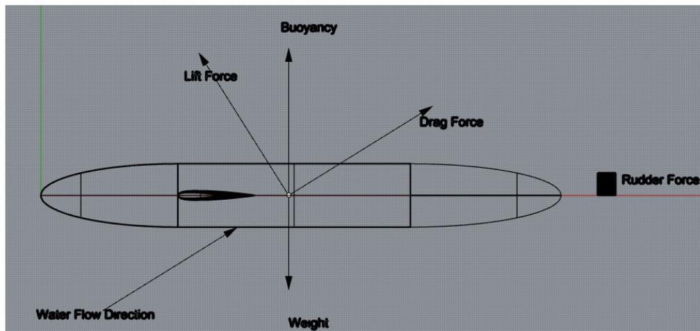
Fig. 2 Forces on the Underwater Glider
