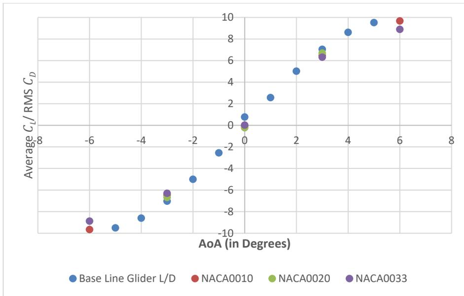
Fig. 18 Mean L/D vs Angle of attack for all four gliders
