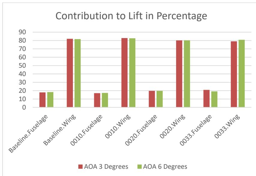
Fig. 15 Contribution of fuselage and wing to the lift of the glider (in percentage)
