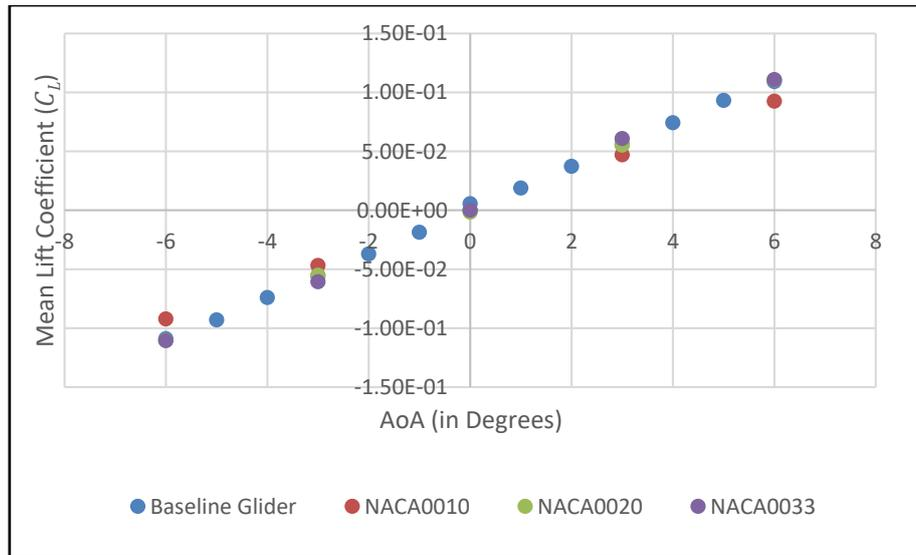
Fig. 17 Mean Lift Coefficient vs Angle of Attack for all four gliders
