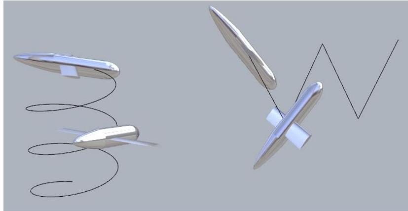
Fig. 1 Glider characteristic maneuver. Turning path in the left and “Sawtooth” motion on right
