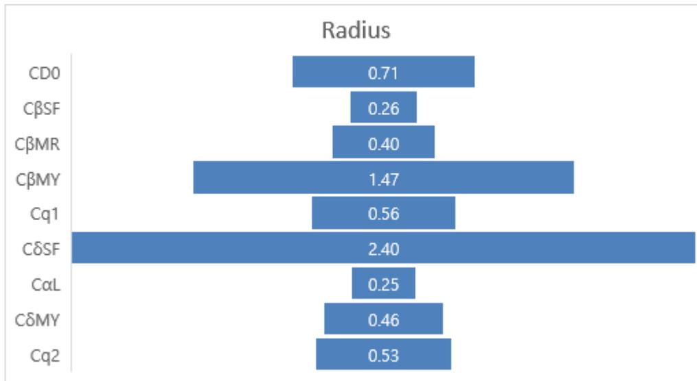
Fig. 5 Sensitivity of the Radius of the Spiral path on the viscous HDCs (Rayaprolu and Vijayakumar 2021)
