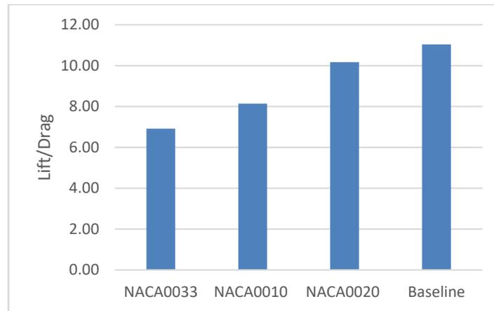
Fig. 13 Comparison of Lift/Drag ratio for all the four gliders
