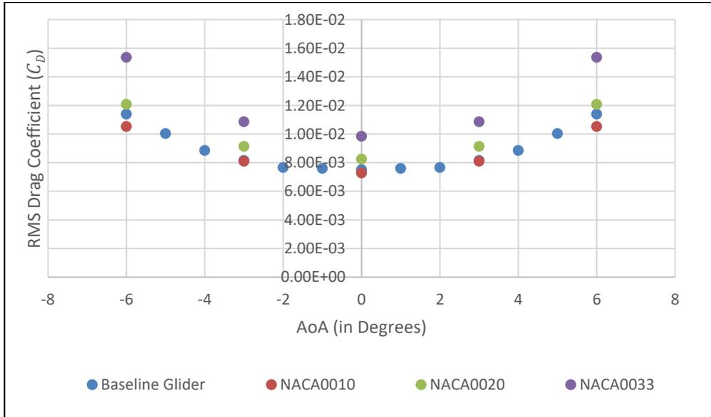
Fig. 16 RMS Drag coefficient vs Angle of attack for all the four gliders
