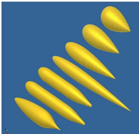
Fig. 3 Standard AUV Bodies. left to right Laminar Flow Body, Autosub 1 to 3, Autosub 6000, NACA 0010, NACA 0020, NACA 0033, NACA 0050 (Stevenson *et al.* 2007)
