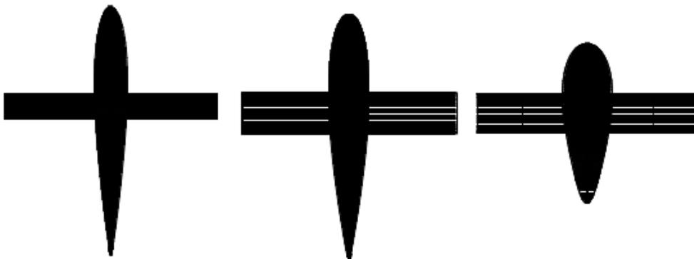
Fig. 8 Body of Revolution generated considering 2D sections of NACA0010, NACA0020 and NACA0033 (Left to Right)
