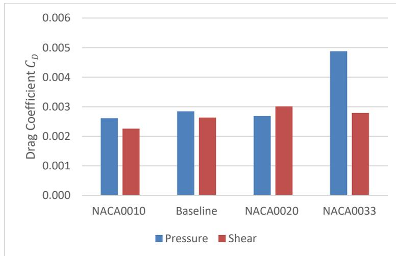
Fig. 11 Comparison of Drag Force Coefficient ( $C_D$ ) for all the four gliders
