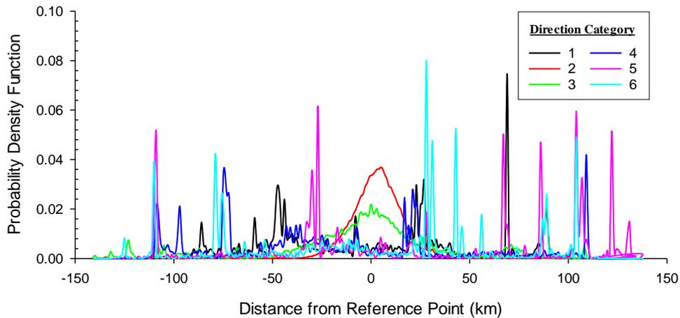
Fig. 4 PDF of ship distribution for each direction category as described in Fig. 3, for five years from June 2016 until May 2021
