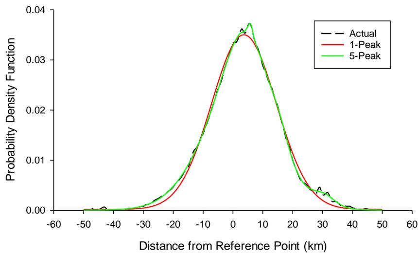
Fig. 8 Comparison of 1-peak and 5-peak Gaussian distribution against actual distribution
