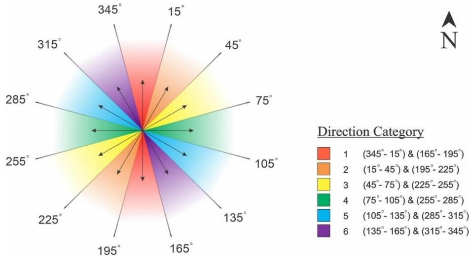
Fig. 1 Illustration of six direction category of ship traffic. The angles is measured from zero degree as true north
