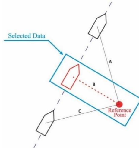
Fig. 2 Illustration of AIS data filter against its relative distance
