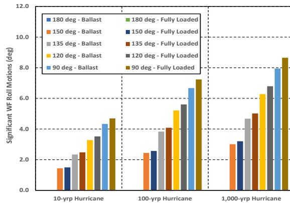
Fig. 27 Significant WF roll motions of the eco-FPSO in 10-yrp, 100-yrp and 1,000-yrp hurricanes
