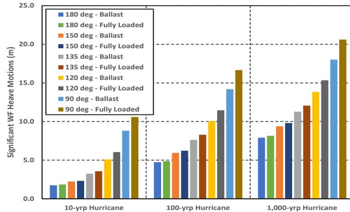
Fig. 22 Significant WF heave motions of the SS-FPSO in 10-yrp, 100-yrp and 1,000-yrp hurricanes
