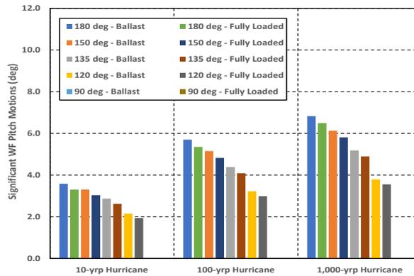
Fig. 31 Significant WF pitch motions of the eco-FPSO in 10-yrp, 100-yrp and 1,000-yrp hurricanes
