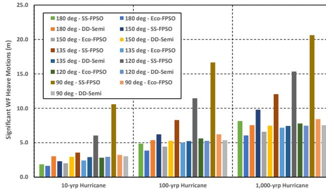
Fig. 25 Significant WF heave motions of the SS-FPSO, the eco-FPSO and the DD-Semi in 10-yrp, 100-yrp and 1,000-yrp hurricanes
