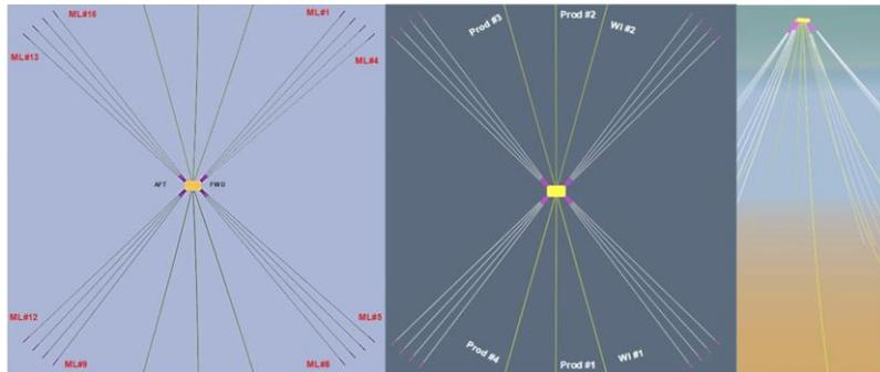
Fig. 5 Field layout – moorings and risers: left, top view of moorings; middle, top view of risers; right, elevation view of moorings and risers
