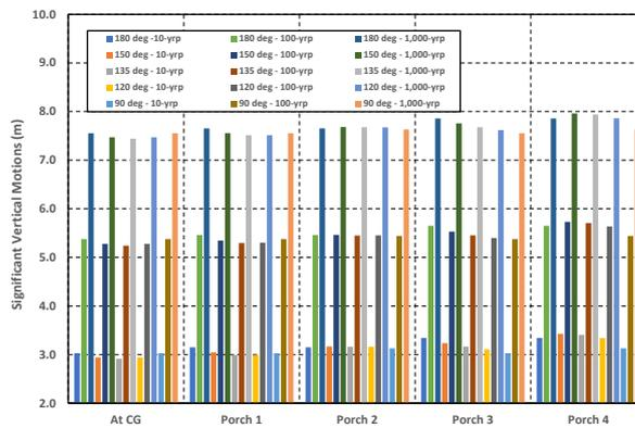
Fig. 34 Extreme WF PVDs and platform heave motions in 10-yrp,100-yrp and 1,000-yrp hurricanes
