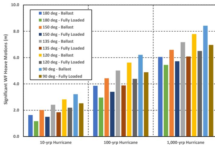
Fig. 23 Significant WF heave motions of the eco-FPSO in 10-yrp, 100-yrp and 1,000-yrp hurricanes
