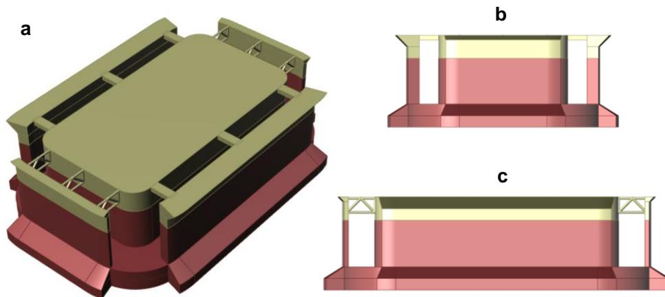
Fig. 3 Eco-FPSO hull configuration only: (a) a perspective view of hull and (b) elevation view – looking FWD-AFT; elevation view – looking port-starboard
