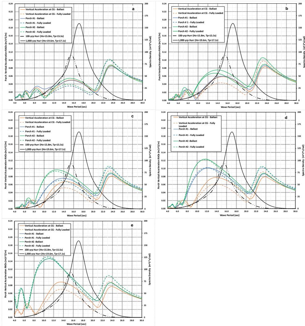
Fig. 18 Comparisons of the PVA RAOs of the eco-FPSO: (a) 180 deg, (b) 150 deg, (c) 135 deg, (d) 120 deg and (e) 90 deg headings
