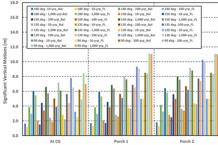
Fig. 37 Extreme WF PVDs and heave motions of the eco-FPSO in 10-yrp,100-yrp and 1,000-yrp hurricanes
