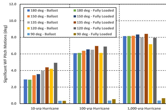
Fig. 30 Significant WF pitch motions of the SS-FPSO in 10-yrp, 100-yrp and 1,000-yrp hurricanes
