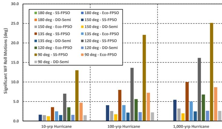
Fig. 29 Significant WF roll motions of the SS-FPSO, the eco-FPSO and the DD-Semi in 10-yrp, 100-yrp and 1,000-yrp hurricanes
