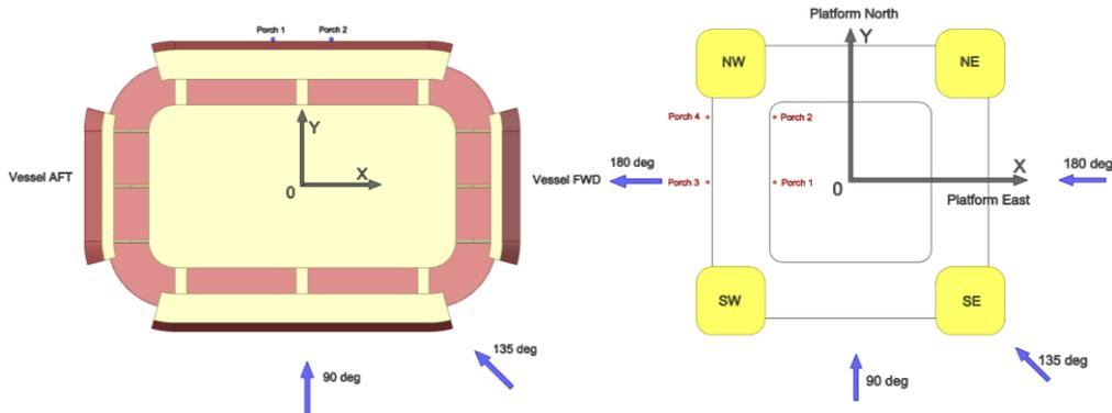
Fig. 12 Locations of SCR porches: left, porches 1 and 2 for the eco-FPSO; right, porches 1 and 2 located at inside of west pontoon; porches 3 and 4 located at outside of west pontoon for the DD-Semi
