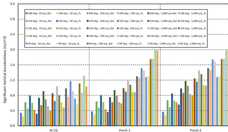
Fig. 39 Extreme WF PVAs and vessel heave accelerations of the eco-FPSO in 10-yrp,100-yrp and 1,000-yrp hurricanes
