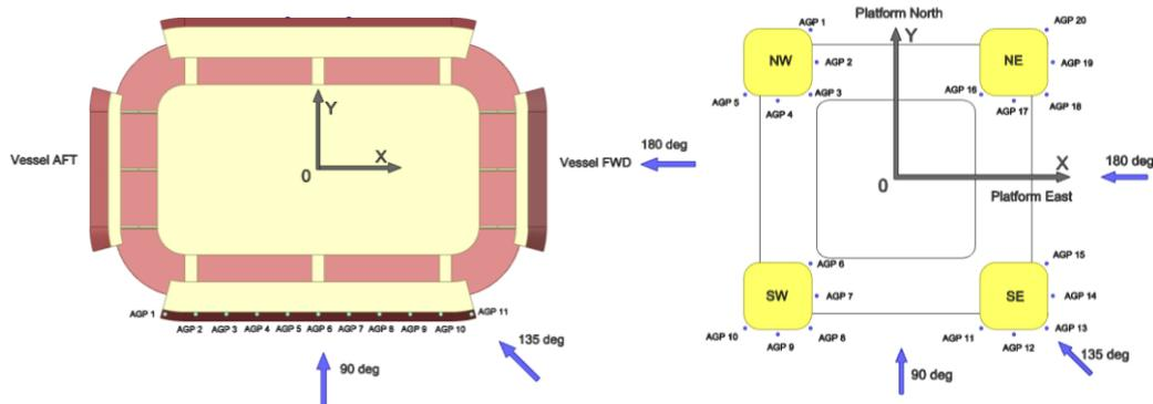
Fig. 10 Points of wave probes for airgaps: left, for the eco-FPSO; right, for the DD-Semi
