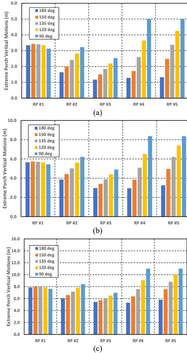
Fig. 40 (a) Extreme WF PVDs in 10-yrp Hurricane, (b) Extreme WF PVDs in 100-yrp Hurricane and (c) Extreme WF PVDs in 1,000-yrp hurricane
