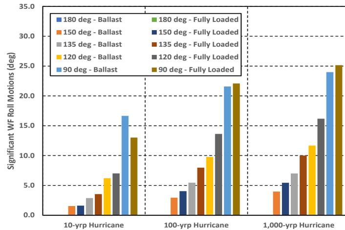
Fig. 26 Significant WF roll motions of the SS-FPSO in 10-yrp, 100-yrp and 1,000-yrp hurricanes
