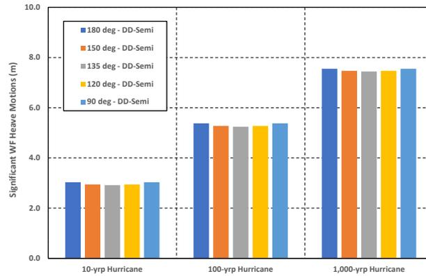
Fig. 24 Significant WF heave motions of the DD-Semi in 10-yrp, 100-yrp and 1,000-yrp hurricanes
