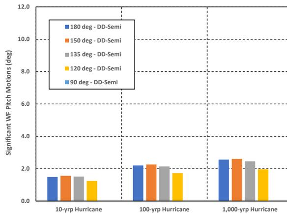
Fig. 32 Significant WF pitch motions of the DD-Semi in 10-yrp, 100-yrp and 1,000-yrp hurricanes
