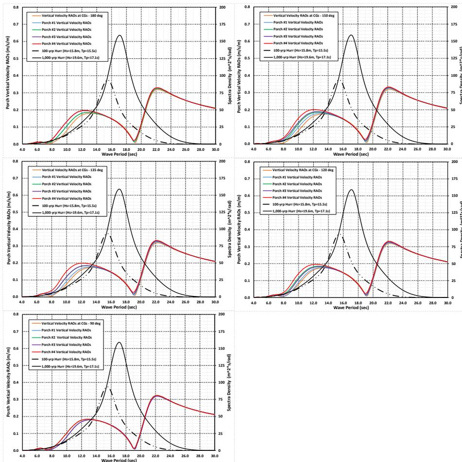
Fig. 14 Comparisons of PVV RAOs of the DD-Semi
