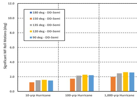
Fig. 28 Significant WF roll motions of the DD-Semi in 10-yrp, 100-yrp and 1,000-yrp hurricanes
