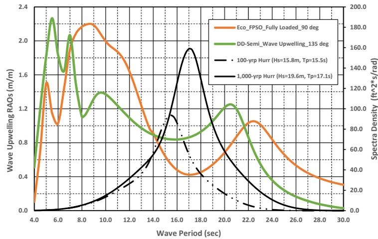
Fig. 11 Comparison of wave upwelling RAOs, eco-FPSO vs DD-Semi
