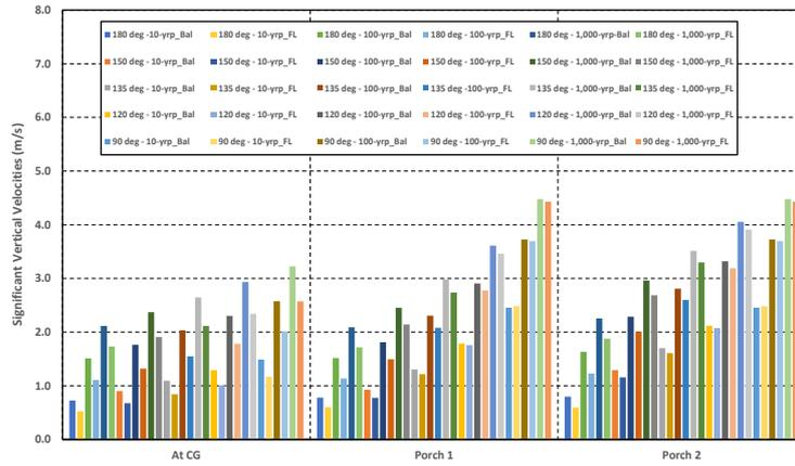
Fig. 38 Extreme WF PVVs and vessel heave velocities of the eco-FPSO in 10-yrp,100-yrp and 1,000-yrp hurricanes
