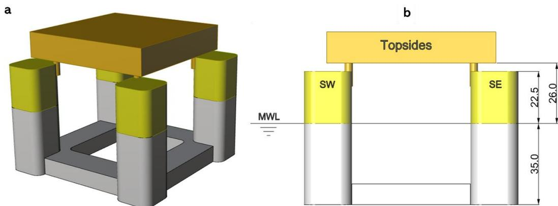
Fig. 4 A DD-Semi platform: (a) a perspective view and (b) elevation view
