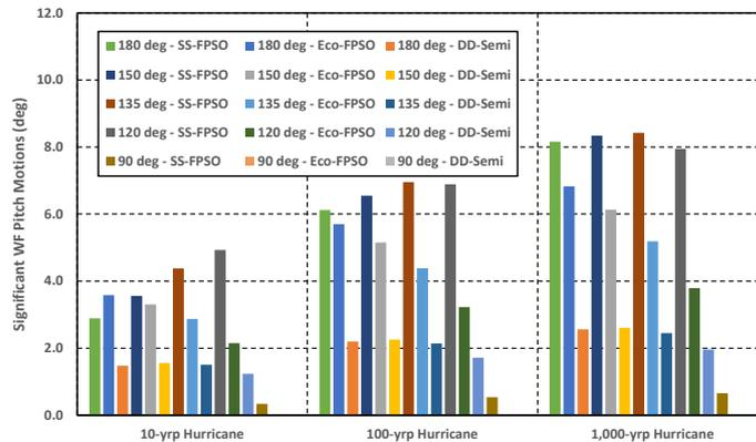
Fig. 33 Significant WF pitch motions of the SS-FPSO, the eco-FPSO and the DD-Semi in 10-yrp, 100-yrp and 1,000-yrp hurricanes
