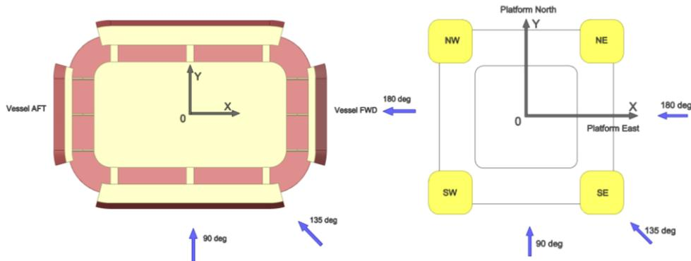
Fig. 6 Heading and coordinate system definitions: left, eco-FPSO; right, DD-Semi platform
