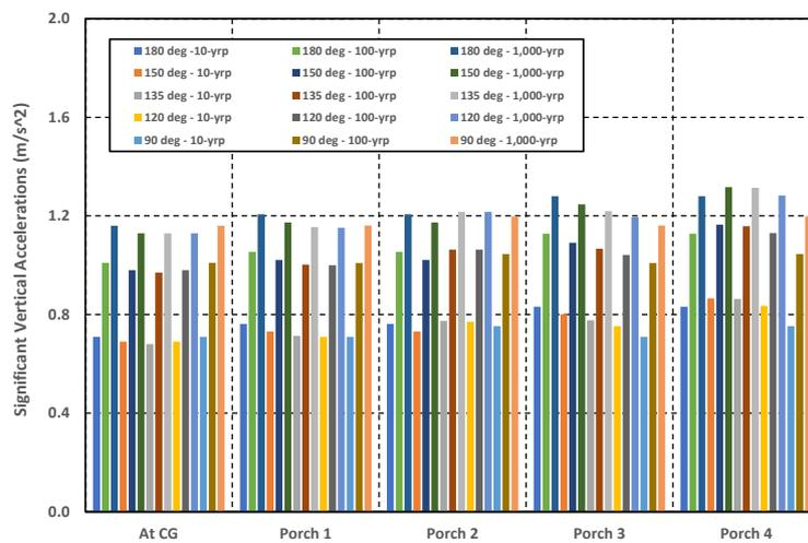
Fig. 36 Extreme WF PVAs and platform heave accelerations in 10-yrp,100-yrp and 1,000-yrp hurricanes
