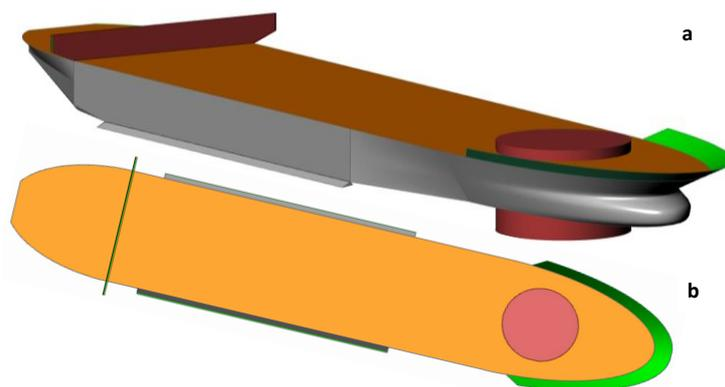
Fig. 2 SS-FPSO hull configuration only: (a) a perspective view of hull and (b) top view
