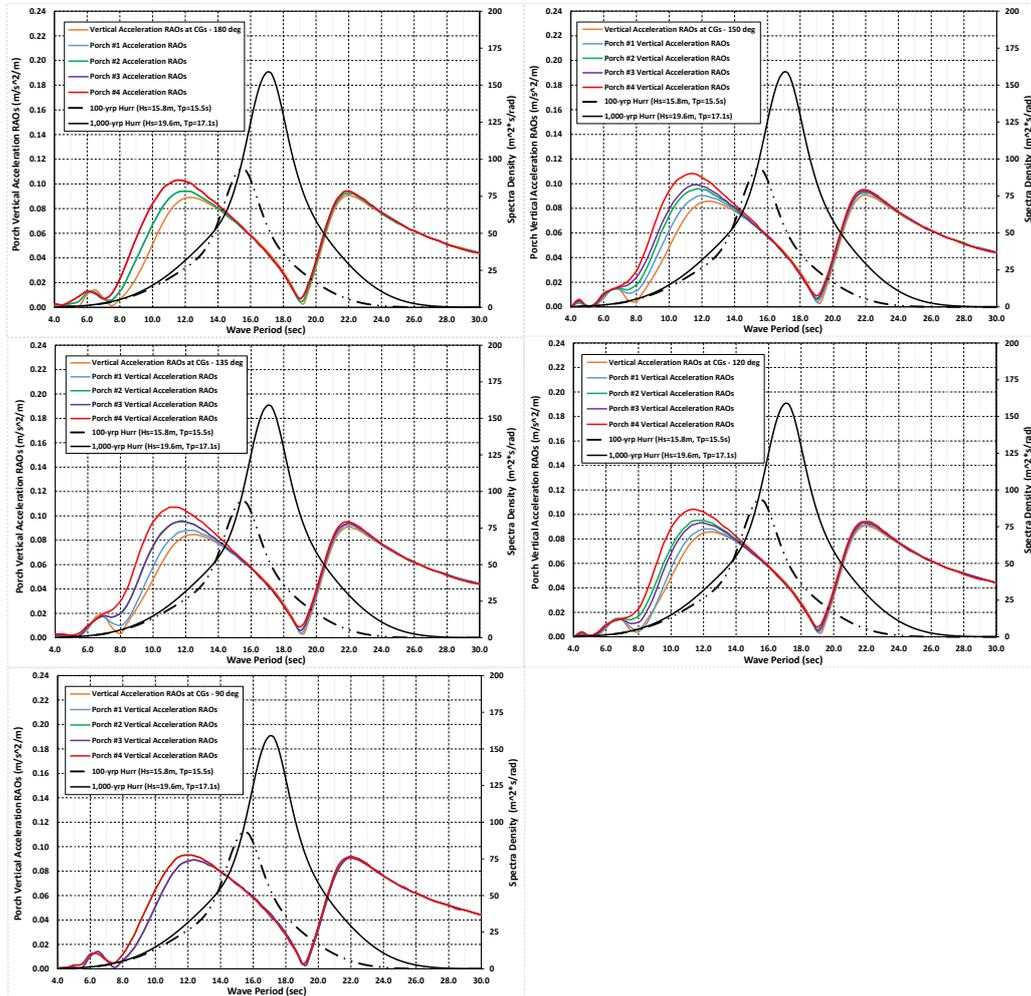
Fig. 15 Comparisons of PVA RAOs of the DD-Semi
