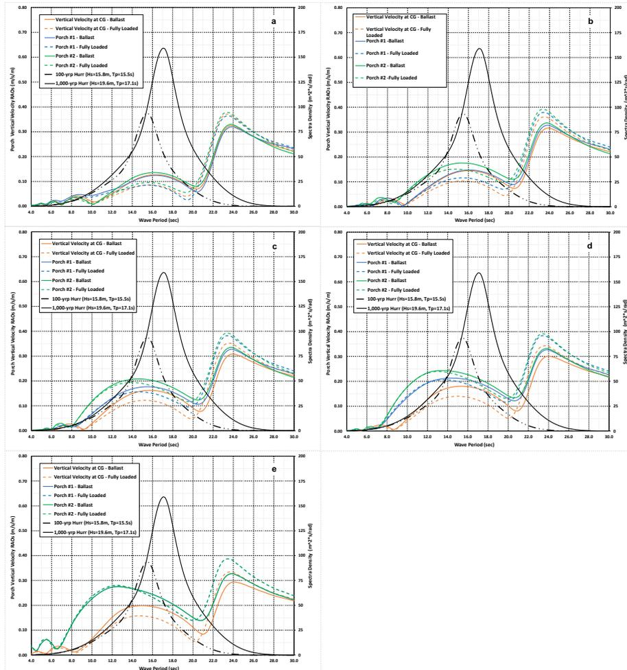
Fig. 17 Comparisons of the PVV RAOs of the eco-FPSO: (a) 180 deg, (b) 150 deg, (c) 135 deg, (d) 120 deg and (e) 90 deg headings
