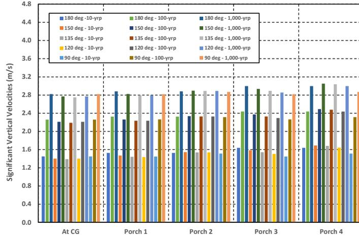
Fig. 35 Extreme WF PVVs and platform heave velocities in 10-yrp,100-yrp and 1,000-yrp hurricanes
