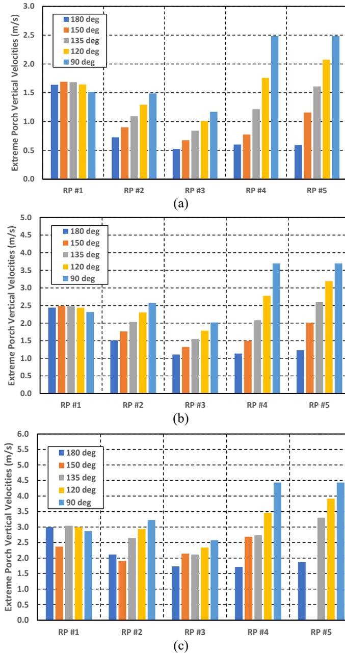
Fig. 41 (a) Extreme WF PVVs in 10-yrp hurricane, (b) Extreme WF PVVs in 100-yrp hurricane and (c) Extreme WF PVVs in 1,000-yrp hurricane
