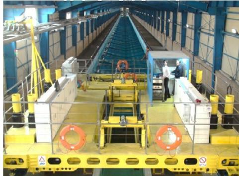
Fig. 1 Wave flume and manned chariot of NIMALA marine laboratory
