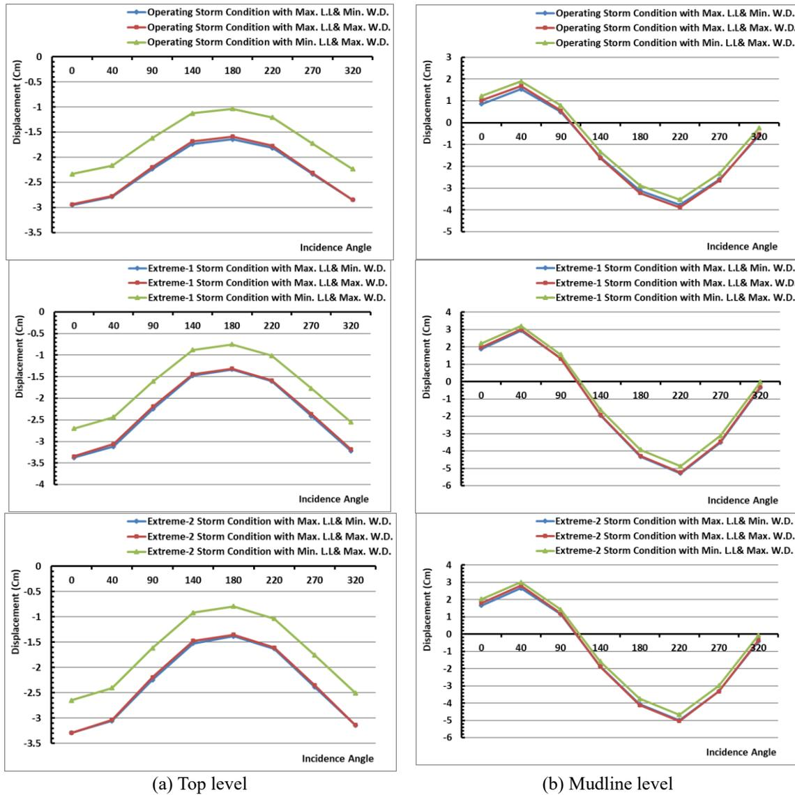
Fig. 11 Vertical displacement for top level (left) and mudline level (right) of (leg A-1) for three storm conditions according to the angles of the environmental loads' directions
