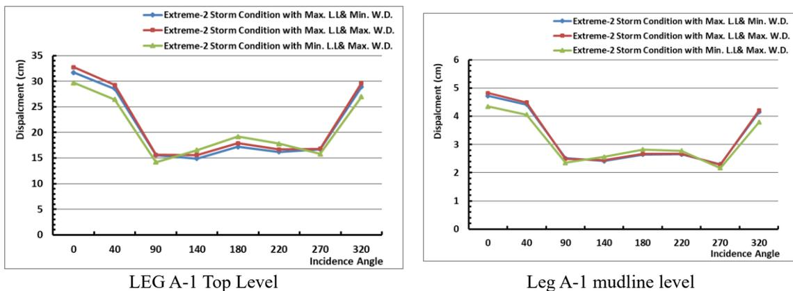
Fig. 10 Absolute horizontal displacement for extreme-2 storm condition
