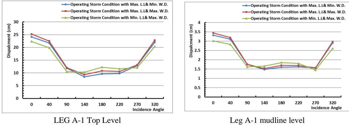
Fig. 8 Absolute horizontal displacement for operating storm condition
