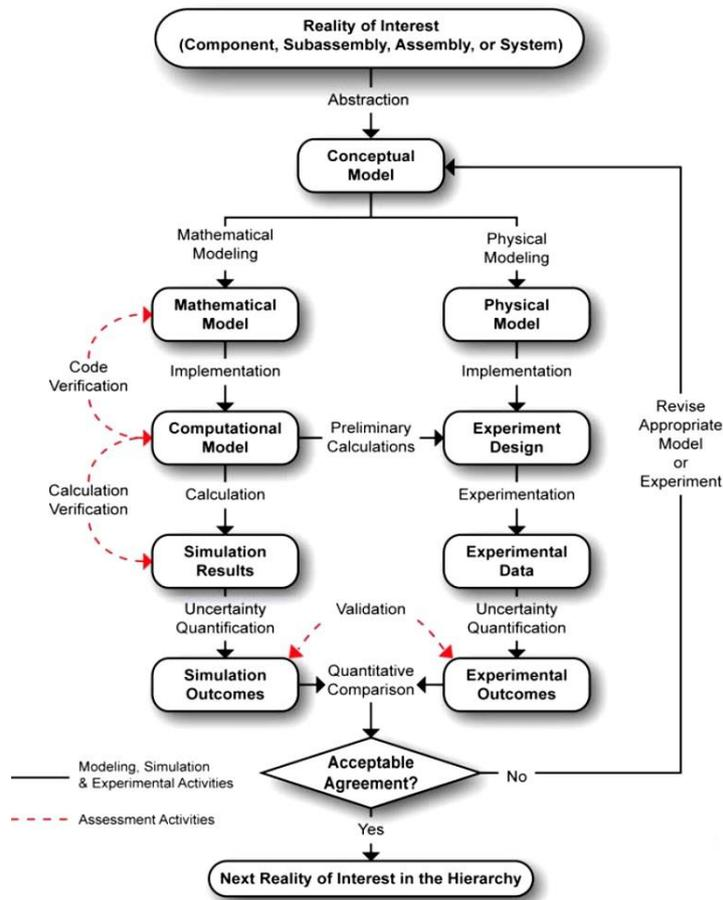
Fig. 5 Verification and Validation assessment through an entire analysis (ASME 2009, 2012)
