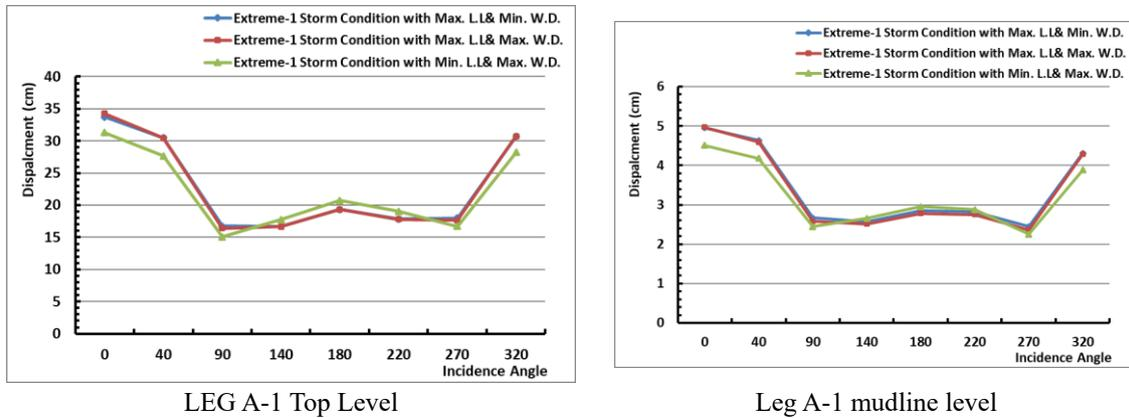
Fig. 9 Absolute horizontal displacement for extreme-1 storm condition
