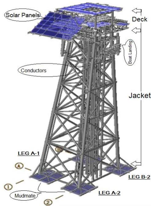
Fig. 4 3D finite element model
