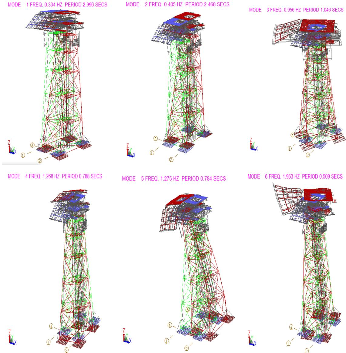
Fig. 6 First six mode shapes and natural frequencies of the platform at site
