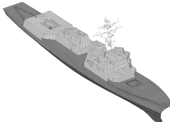
Fig. 2 DDG 81 finite element model (Harrington 2002)
