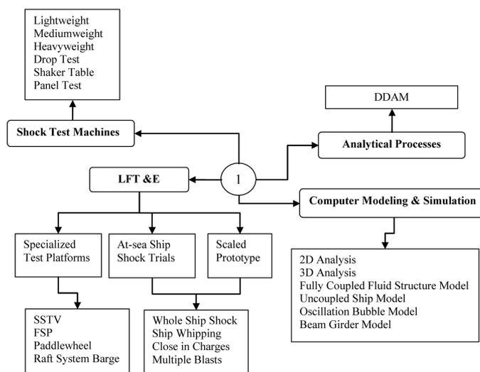
Fig. 7 UNDEX Shock testing toolkit
