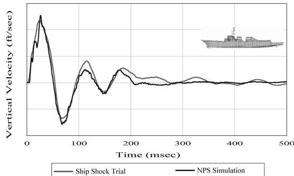
Fig. 5 Vertical velocity response of DDG-81 node/sensor Pair (Shin and Schneider 2003)
