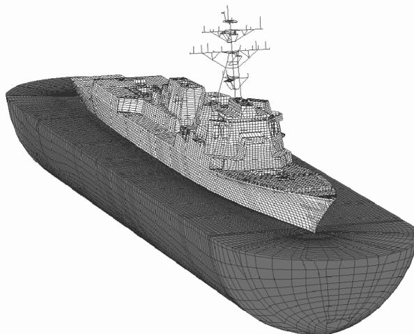
Fig. 4 USS WINSTON S. CHURCHILL Coupled fluid-structure model (Shin and Schneider 2003)
