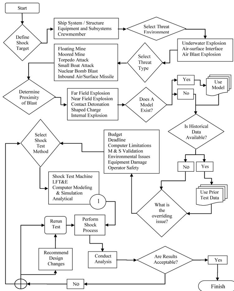
Fig. 6 Threat based surface ship shock analysis decision making tool
