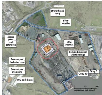
Fig. 2 Topside structures placement during onshore dismantling (Shell 2019)
