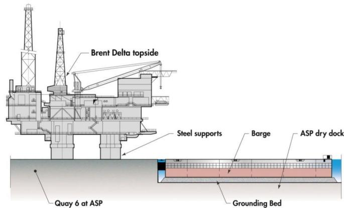
Fig. 3 Topside load-in operation (Shell 2019)
