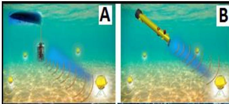
Fig. 1 Rendering showing OWC in data collection from an offshore node
