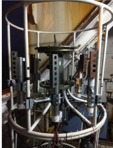
Fig. 2 Water sampler used for sample collection up to 195 m water depth
