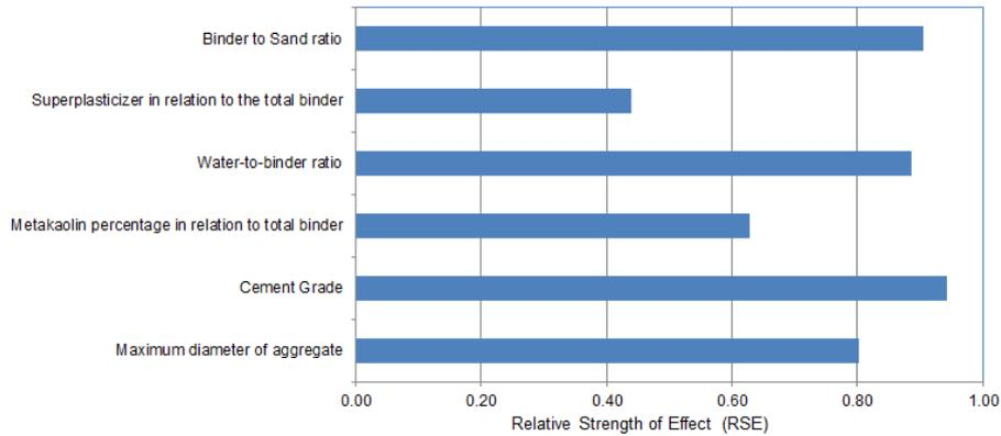
Fig. 4 Sensitivity analysis of cement-metakaolin mortars compressive strength
