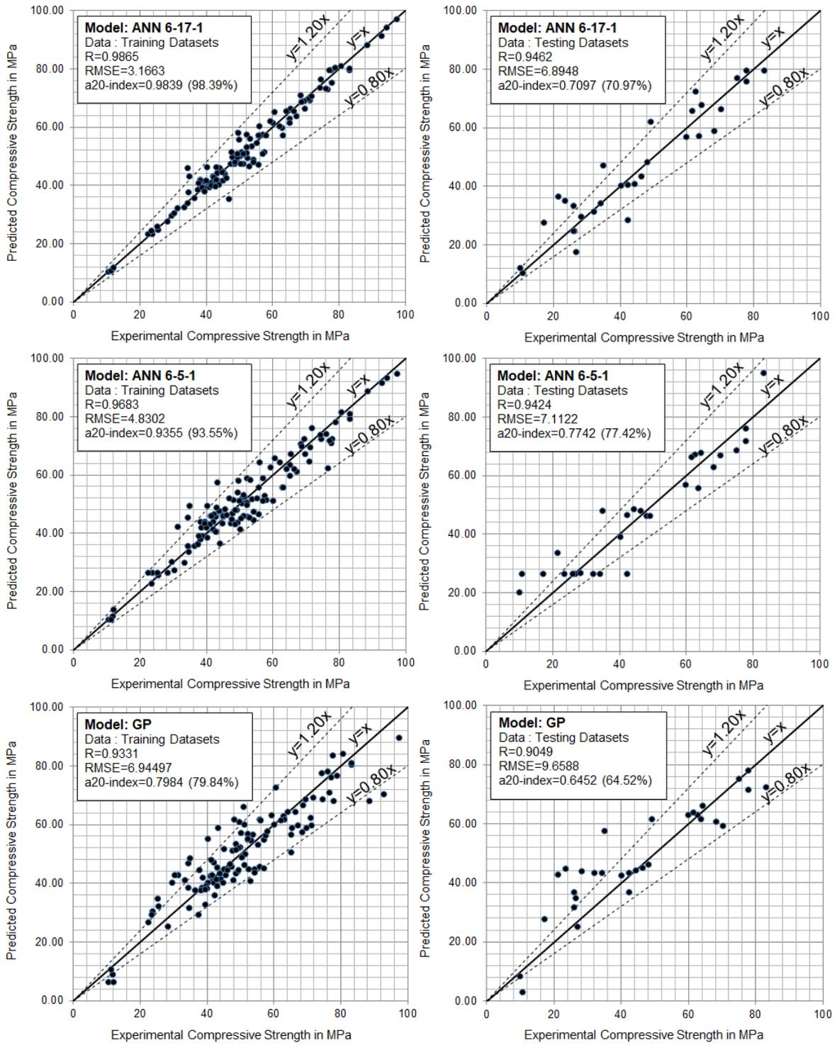
Fig. 9 Experimental vs Predicted values of compressive strength for the three developed models
