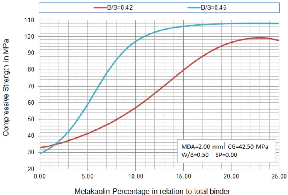
Fig. 13 Mortar Compressive Strength vs Metakaolin to total Binder (MK/B) ratio at various binder to sand ratio (MDA=2.00 mm, CG=42.50, W/B=0.50 and SP=0.00) based on the proposed 6-17-1 ANN model
