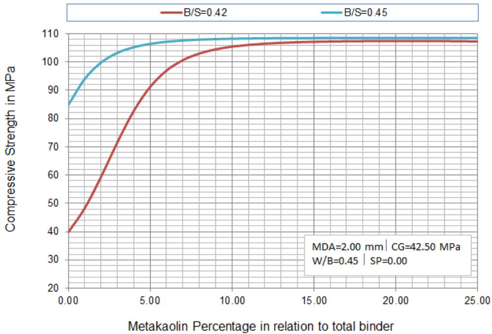
Fig. 12 Mortar Compressive Strength vs Metakaolin to total Binder (MK/B) ratio at various binder to sand ratio (MDA=2.00 mm, CG=42.50, W/B=0.45 and SP=0.00) based on the proposed 6-17-1 ANN model
