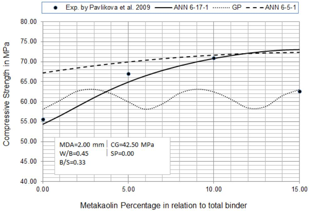
Fig. 10 Experimental verification of the developed models using experimental data by Pavlikova *et al.* 2009, for cement grade 42.5 MPa
