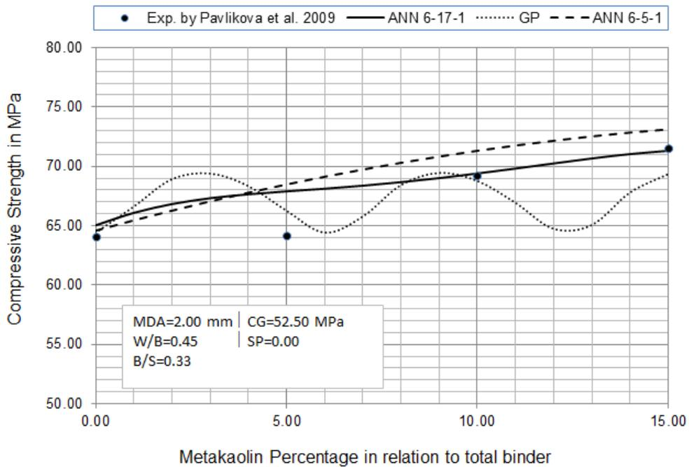
Fig. 11 Experimental verification of the developed models using experimental data by Pavlikova *et al.* 2009, for cement grade 52.5 MPa
