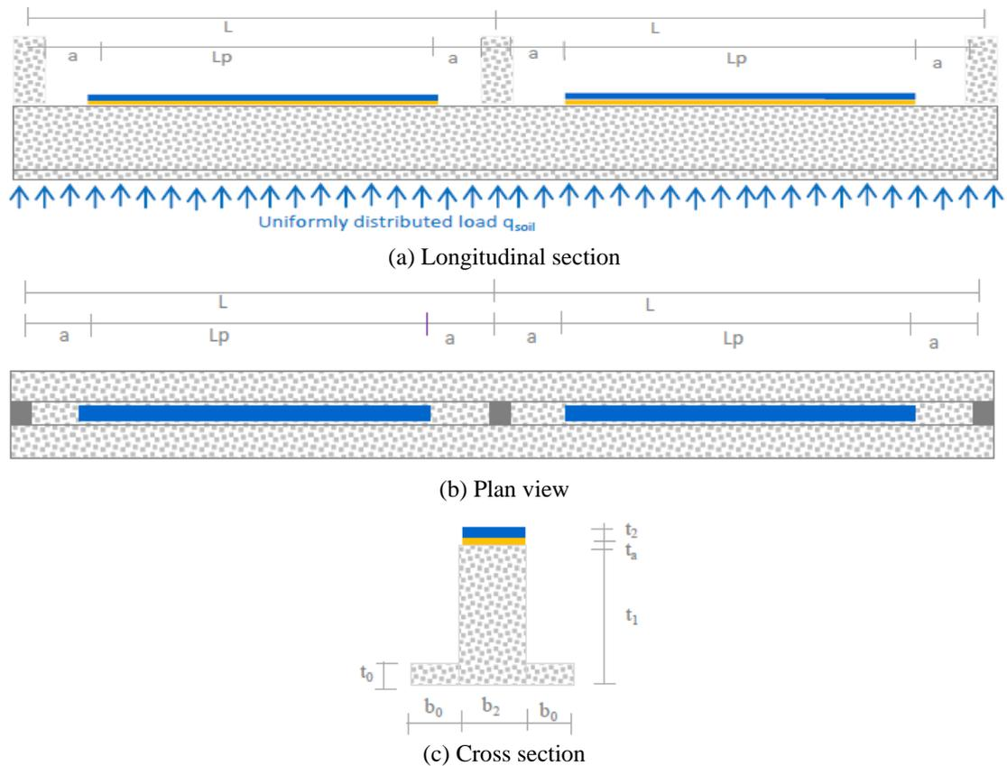
Fig. 1 Reinforced concrete foundation beam repairing with composite plate
