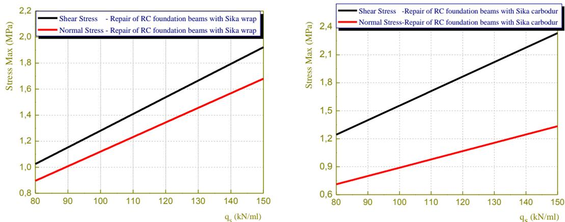
Fig. 11 Effect soil stress characteristics on interfacial stresses in reinforced concrete foundation beam repaired with composite plate
