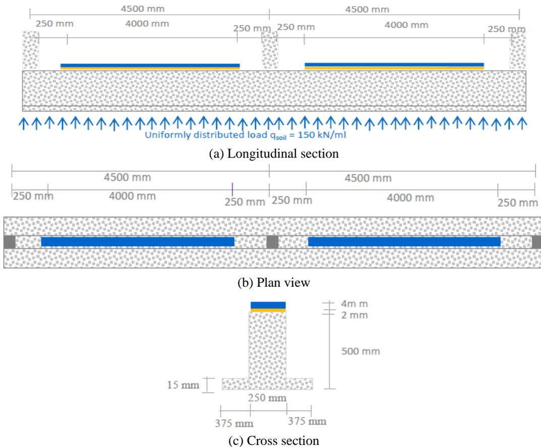
Fig. 3 Geometric characteristic of a reinforced concrete foundation beam repaired with composite plate
