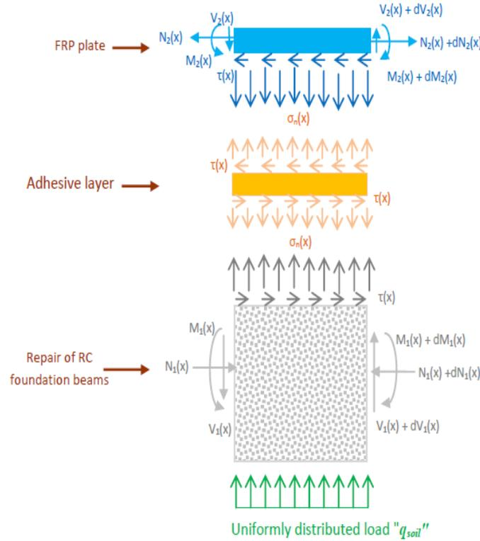
Fig. 2 Forces in an infinitesimal element of an FRP- repairing RC foundation beam
