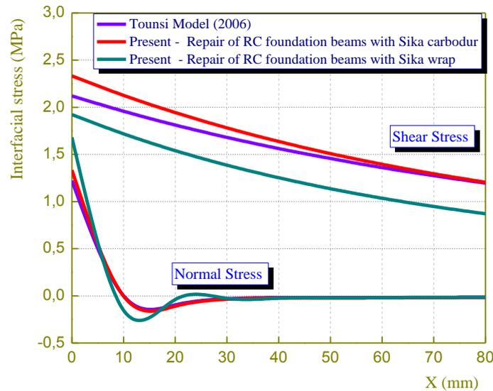
Fig 4 Comparison analytical results of interfacial stresses for composite plate repaired RC foundation beam
