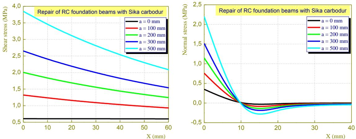
Fig. 13 Effect of the length of the repair plate  $L_p$  on interfacial stresses in reinforced concrete foundation beam repaired with Sika Carbodur composite plate
