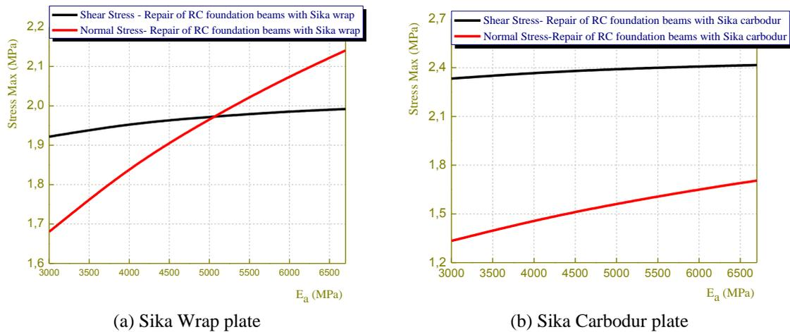
Fig. 17 Effect of elasticity modulus of adhesive layer on interfacial stresses in reinforced concrete foundation beam repaired with composite plate
