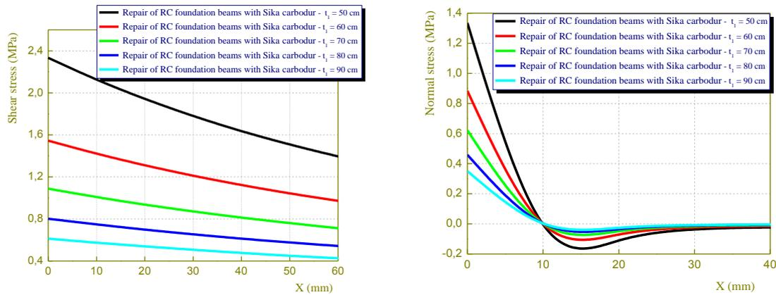
Fig. 7 Effect of rigidity of the RC beam on interfacial stresses in reinforced concrete foundation beam repaired with Sika Carbodur composite plate
