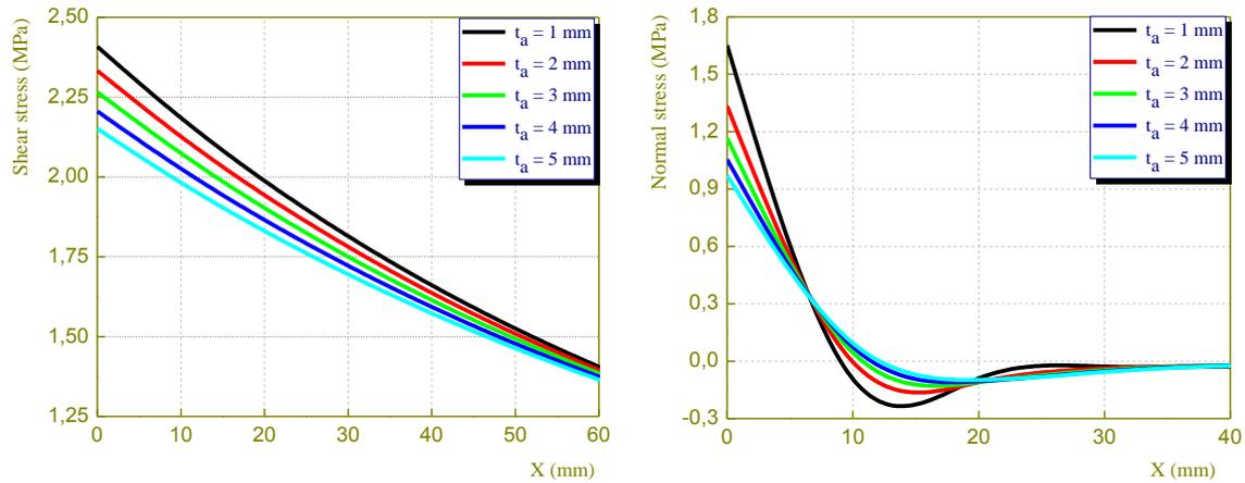
Fig. 19 Effect of adhesive layer thickness on interfacial stresses in reinforced concrete foundation beam repaired with Sika Carbodur composite plate
