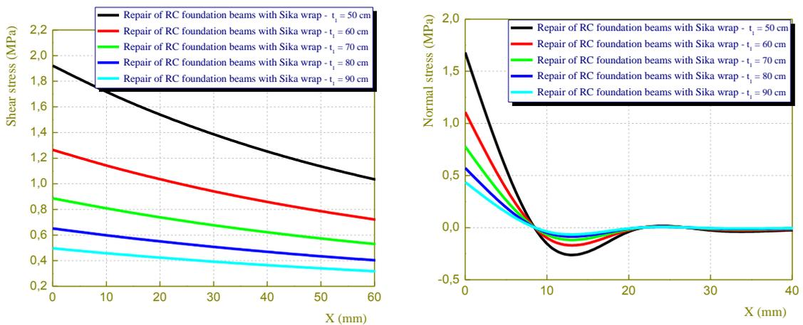
Fig. 6 Effect of rigidity of the RC beam on interfacial stresses in reinforced concrete foundation beam repaired with Sika Wrap composite plate
