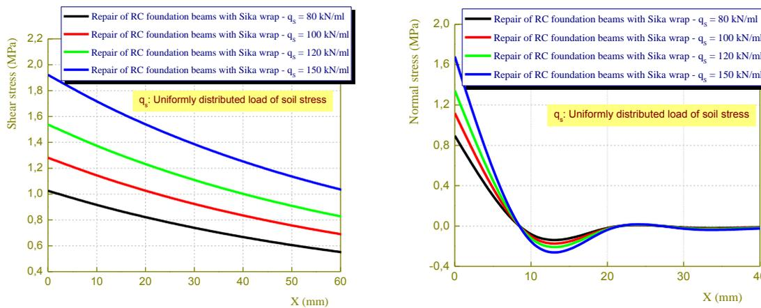
Fig. 9 Effect soil stress characteristics on interfacial stresses in reinforced concrete foundation beam repaired with Sika Wrap composite plate
