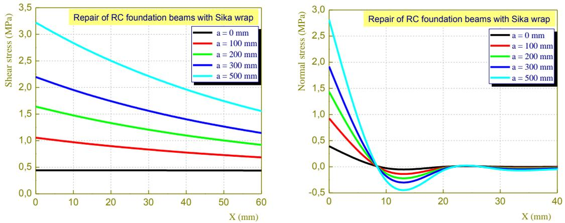
Fig. 12 Effect of the length of the repair plate  $L_p$  on interfacial stresses in reinforced concrete foundation beam repaired with Sika Wrap composite plate
