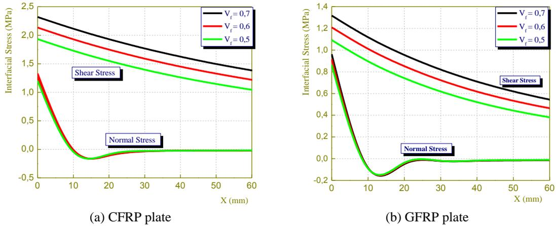
Fig. 14 Effect of fiber volume fraction on interfacial stresses in reinforced concrete foundation beam repaired with composite plate (a) CFRP plate and (b) GFRP plate
