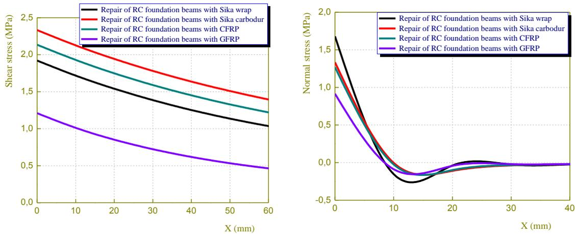
Fig. 5 Effect of plate stiffness on interfacial stresses in reinforced concrete foundation beam repaired with composite plate
