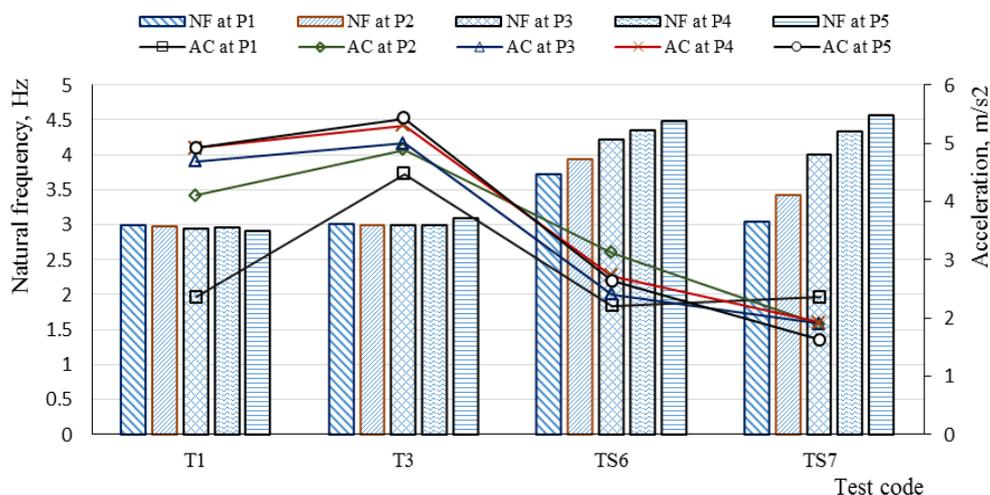
Fig. 20 Comparison of natural frequencies (NF) and acceleration (AC) between  $T_1$ ,  $T_3$ ,  $TS_4$  and  $TS_7$  test with different tire inflation pressure.  $P_1$ ,  $P_2$ ,  $P_3$ ,  $P_4$  and  $P_5$  are tire inflation pressure of 60, 90, 120, 150 and 180 kPa contributed for  $T_1$  and  $TS_4$ , and 120, 150, 180, 210, 240 kPa contributed for  $T_3$  and  $TS_7$  test, respectively. All values considering the first natural frequency
