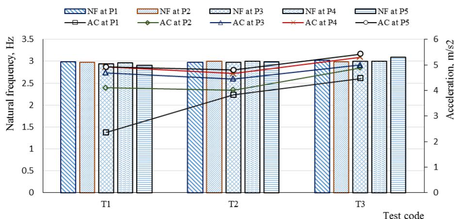
Fig. 17 Comparison of natural frequencies (NF) and acceleration (AC) between  $T_1$ ,  $T_2$  and  $T_3$  test with different tire inflation pressure.  $P_1$ ,  $P_2$ ,  $P_3$ ,  $P_4$  and  $P_5$  is tire inflation pressure of 60, 90, 120, 150 and 180 kPa contributed for  $T_1$  and  $T_2$ , and is 120, 150, 180, 210, 240 kPa contributed for  $T_3$  test, respectively. All values considering at the first natural frequency
