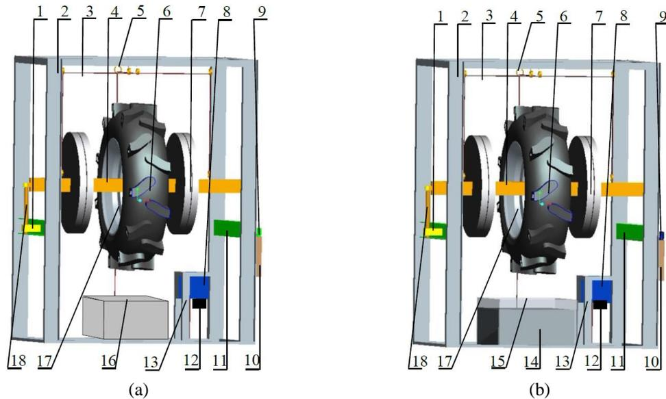
Fig. 2 The test rig (a) For measuring the acceleration of test tires dropping on rigid ground; (b) For measuring the acceleration of test tire dropping on soft soil
