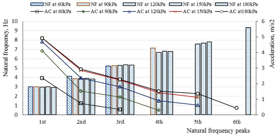
Fig. 4 Variation of vertically natural frequency and acceleration values of  $T_1$  test tire
