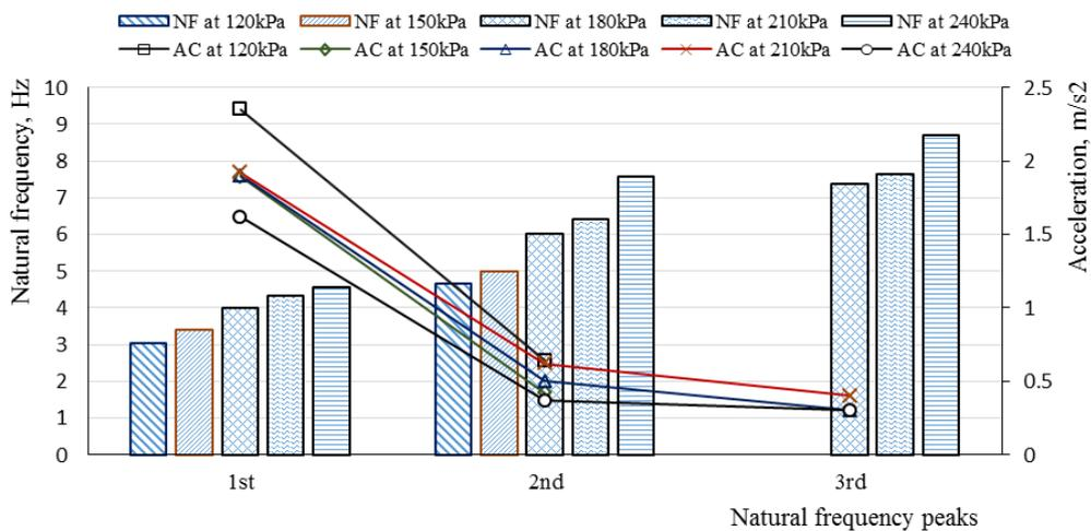
Fig. 16 Variation of vertically natural frequency and acceleration values of *TS*<sub>7</sub> test tire
