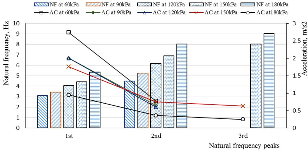
Fig. 12 Variation of vertically natural frequency and acceleration values of  $TS_5$  test tire
