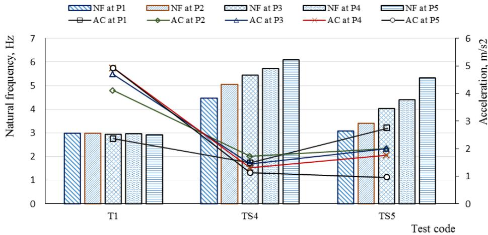
Fig. 18 Comparison of natural frequencies (NF) and acceleration (AC) between  $T_1$ ,  $TS_4$  and  $TS_5$  test with different tire inflation pressure.  $P_1$ ,  $P_2$ ,  $P_3$ ,  $P_4$  and  $P_5$  is tire inflation pressure of 60, 90, 120, 150 and 180 kPa, respectively. All values considering the first natural frequency
