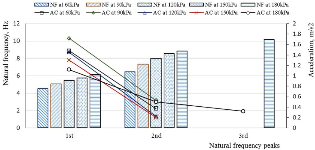
Fig. 10 Variation of vertically natural frequency and acceleration values of  $TS_4$  test tire
