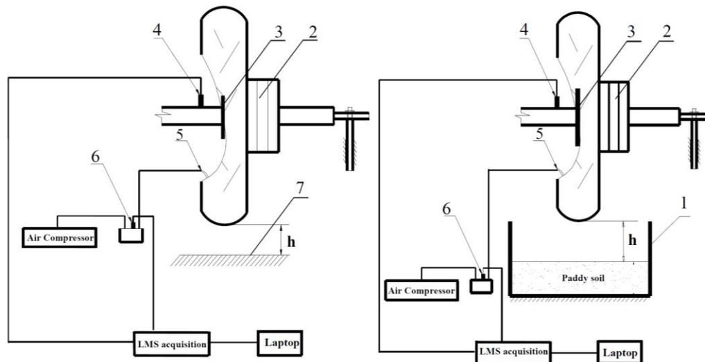
Fig. 1 Sketch of the measurement system. (a) Sketch for measurement of vertical acceleration of tractor tire dropping on the rigid ground; (b) Sketch for measurement of vertical acceleration of tractor tire dropping on soft soil: 1. Steel bin, 2. Load, 3. Plate to link tire rim, 4. Acceleration sensor, 5. Tire valve, 6. Air pressure sensor, 7. Rigid ground
