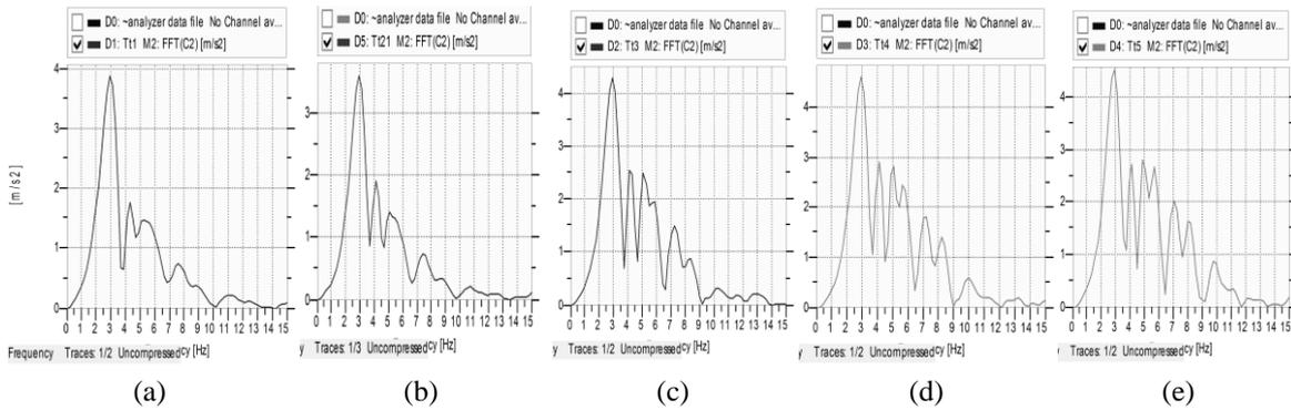
Fig. 5 The spectrum of vertical acceleration in frequency domain of tire  $T_2$ : Figs. 5(a), (b), (c), (d), (e) show acceleration spectrum of tire inflation pressure of 60, 90, 120, 150 and 180 kPa, respectively
