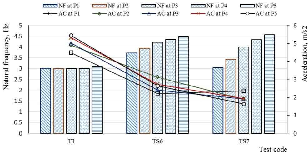
Fig. 19 Comparison of natural frequencies (NF) and acceleration (AC) between  $T_3$ ,  $TS_6$  and  $TS_7$  test with different tire inflation pressure.  $P_1$ ,  $P_2$ ,  $P_3$ ,  $P_4$  and  $P_5$  are tire inflation pressure of 120, 150, 180, 210, 240 kPa, respectively. All values considering the first natural frequency
