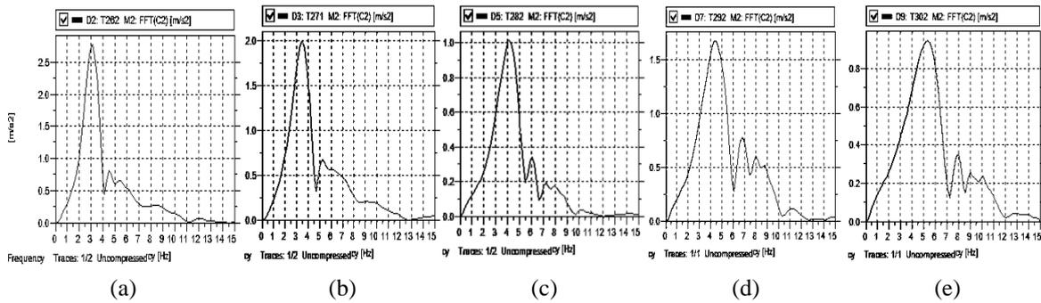
Fig. 11 The spectra of vertical acceleration in frequency domain of tire  $TS_5$  when tire inflation pressure increased: Figs. 11(a), (b), (c), (d) and Fig. 9(e) for tire inflation pressure change from 60 to 180 kPa, increment of 30 kPa, respectively
