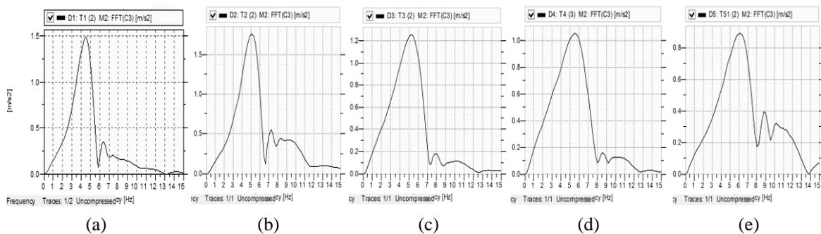
Fig. 9 The spectra of vertical acceleration in frequency domain of  $TS_4$  test when tire inflation pressure increased: Figs. 9(a), (b), (c), (d) & (e) for tire inflation pressure change from 60 to 180 kPa, with increment of 30 kPa, respectively
