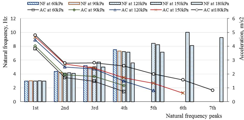
Fig. 6 Variation of vertically natural frequency and acceleration values of  $T_2$  test tire
