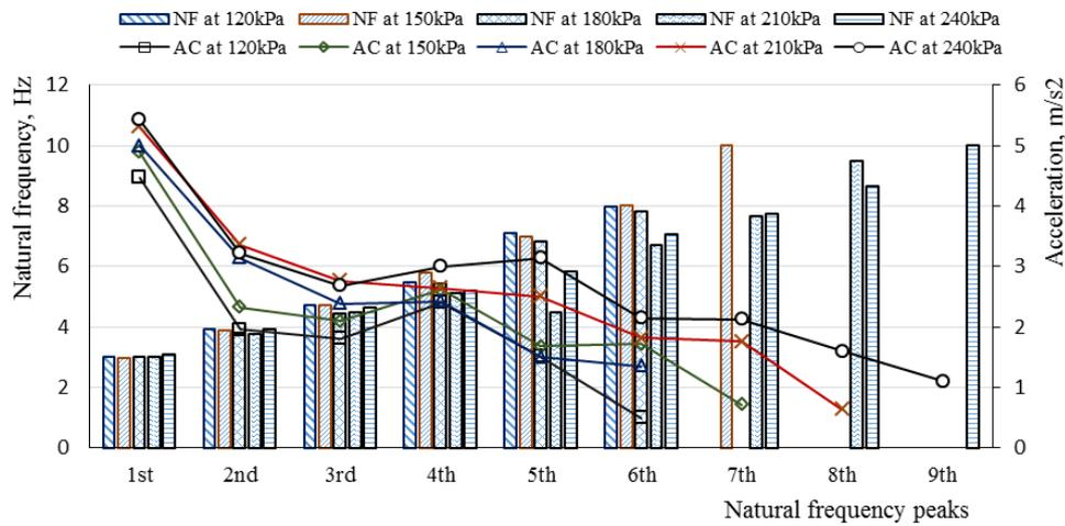
Fig. 8 Variation of vertically natural frequency and acceleration values of  $T_3$  test tire
