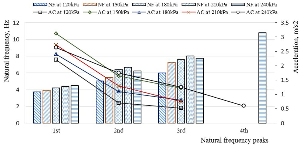
Fig. 14 Variation of vertically natural frequency and acceleration values of *TS*<sub>6</sub> test tire
