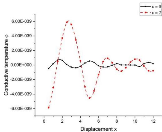
Fig. 12 Variation of conductive temperature  $\phi$  with displacement  $x$  (thermal source)
