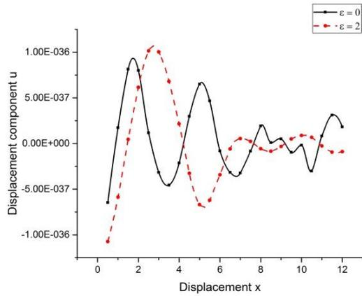
Fig. 7 Variation of displacement component  $u$  with displacement  $x$  (thermal source)
