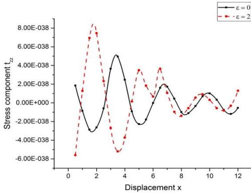
Fig. 3 Variation of stress component  $t_{zz}$  with displacement  $x$  (mechanical force)
