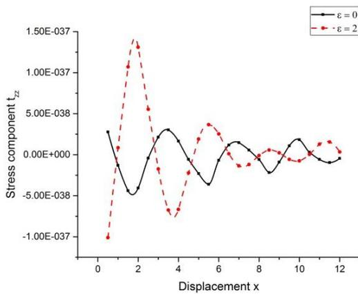
Fig. 9 Variation of stress component  $t_{zz}$  with displacement  $x$  (thermal source)
