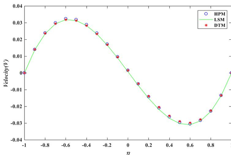
Fig. 3(b) Velocity profile for Cu-SA nanofluid when  $r=0$ ,  $\beta=0.05$ ,  $\delta=Ec=Pr=1$
