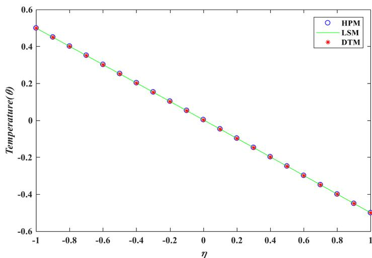
Fig. 3(a) Temperature profile for Cu-SA nanofluid when  $r=0$ ,  $\beta=0.05$ ,  $\delta=Ec=Pr=1$
