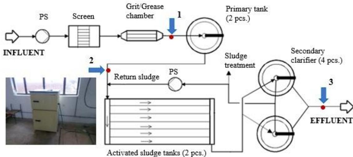
Fig. 3 Scheme of the WWTP Butile/Sarajevo with location of the automatic samplers; 1 - downstream of aerated Grid/Grease Chamber, 2 - inlet to biology and 3 - effluent
