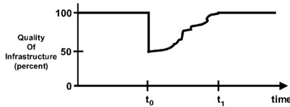
Fig. 4 Schematic representation of seismic resilience concept (Bruneau *et al.* 2003)
