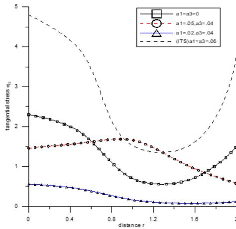
Fig. 6 Variation of tangential stress  $\sigma_{zr}$  with the distance  $r$ (normal force over the circular region)
