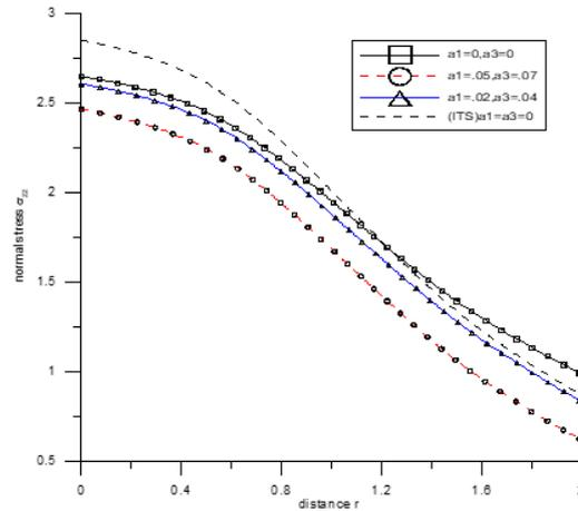
Fig. 7 Variation of normal stress  $\sigma_{zz}$  with the distance  $r$  (normal force over the circular region)
