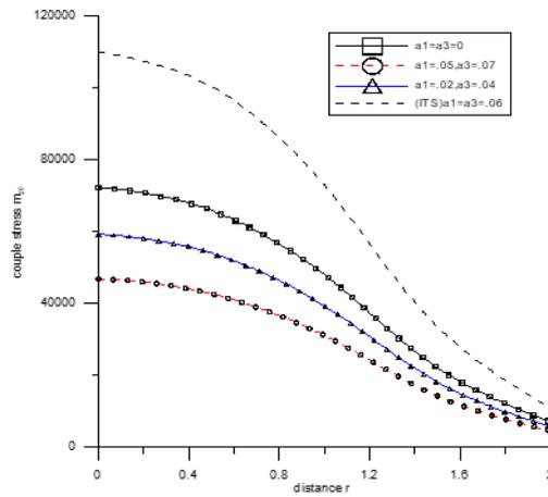
Fig. 12 Variation of couple stress  $m_{z\theta}$  with the distance  $r$ (thermal point source)
