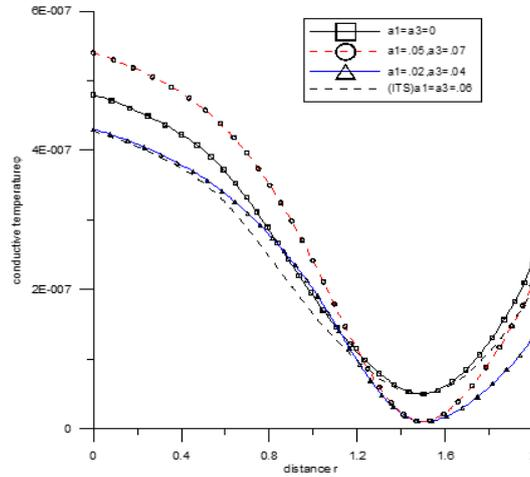
Fig. 1 Variation of conductive temperature  $\varphi$  with the distance  $r$ (concentrated normal force)
