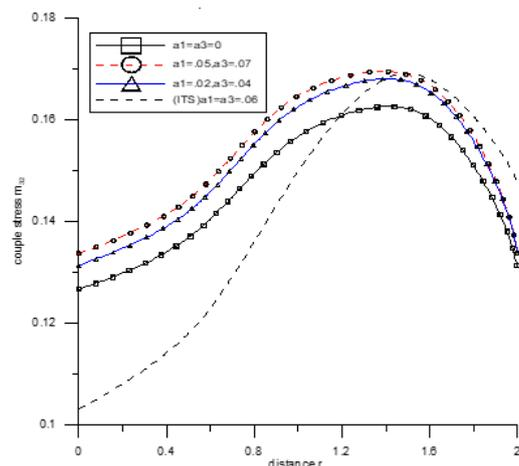
Fig. 8 Variation of couple stress  $m_{z\theta}$  with the distance  $r$  (normal force over the circular region)
