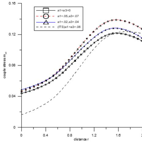
Fig. 4 Variation of couple stress  $m_{z\theta}$  with the distance  $r$ (concentrated normal force)
