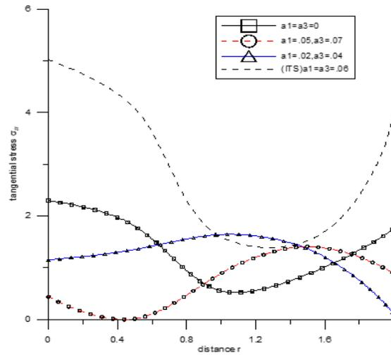
Fig. 2 variation of tangential stress  $\sigma_{zr}$  with the distance  $r$ (concentrated normal force)
