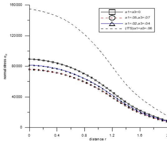
Fig. 11 Variation of normal stress  $\sigma_{zz}$  with the distance  $r$ (thermal point source)
