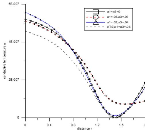
Fig. 5 Variation of conductive temperature  $\phi$  with the distance  $r$ (normal force over the circular region)
