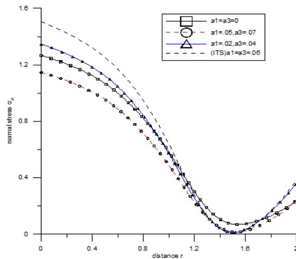
Fig. 3 Variation of normal stress  $\sigma_{zz}$  with the distance  $r$ (concentrated normal force)
