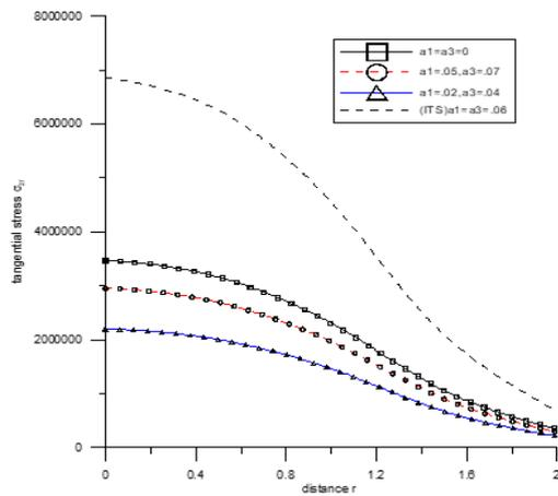
Fig. 10 Variation of tangential stress  $\sigma_{zr}$  with the distance  $r$ (thermal point source)
