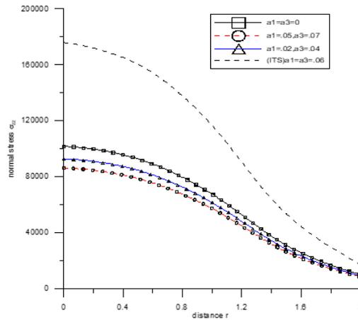
Fig. 15 Variation of normal stress  $\sigma_{zz}$  with the distance  $r$ (thermal source over the circular region)
