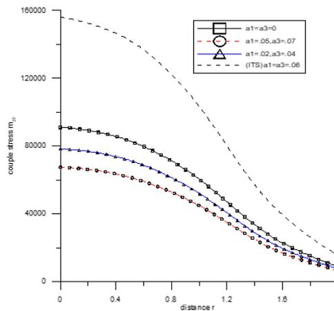
Fig. 16 Variation of couple stress  $m_{z\theta}$  with the distance  $r$ (thermal source over the circular region)
