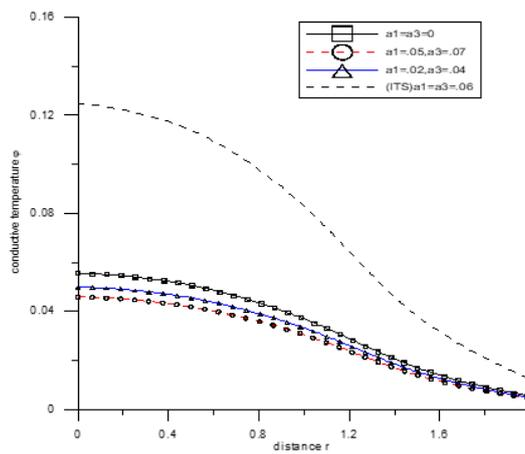
Fig. 13 Variation of conductive temperature  $\phi$  with the distance  $r$  (thermal source over the circular region)
