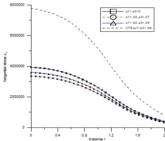
Fig. 14 Variation of tangential stress  $\sigma_{zr}$  with the distance  $r$ (thermal source over the circular region)
