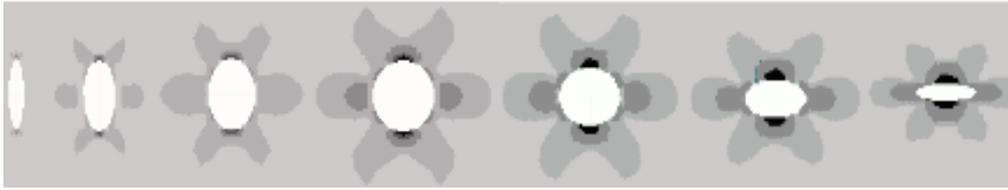
Fig. 3 Patterns of the distribution of strain intensity  $p_u$  in the  $Oxz$  section
