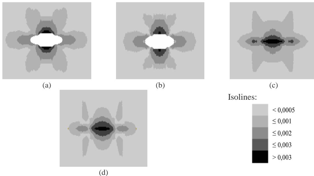
Fig. 9 Distribution of strain intensity  $p_u$  in a plate with an elliptical hole (a, b) and a crack (c, d) in an elastic (a, c) and elastoplastic (b, d) cases
