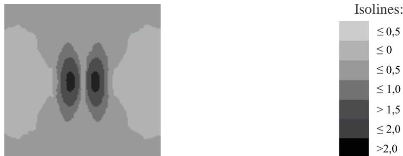
Fig. 8 Distribution of values of tangential stresses  $\tau_{zx}$  [MPa] in case of crack
