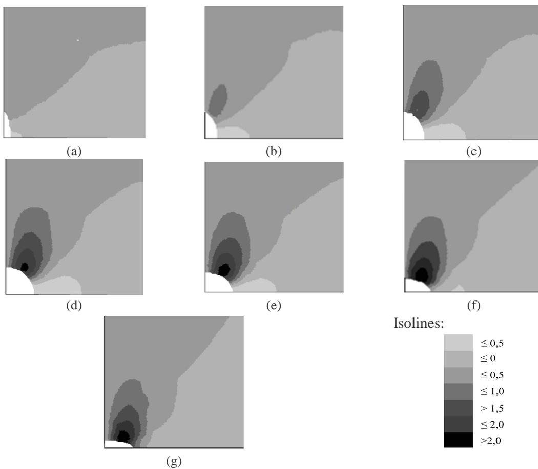
Fig. 7 Distribution of tangential stresses  $\tau_{zx}$  [MPa] in 1/4 of the plate
