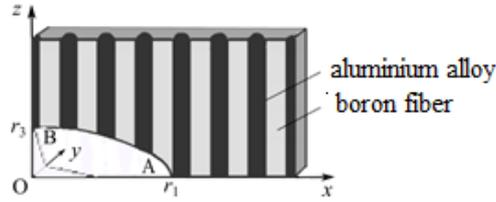
Fig. 1 The fourth part of the plate section on plane *Oxz*
