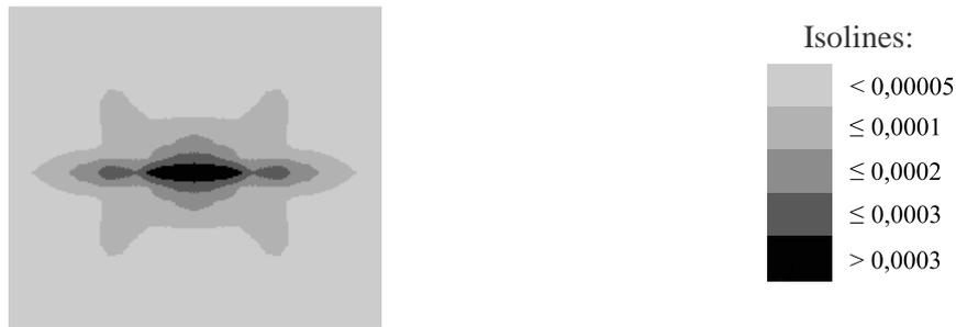
Fig. 4 Distribution of strain intensity values  $-p_u$  in case of crack
