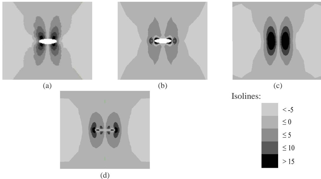
Fig. 10 Distribution of tangential stresses  $\tau_{zx}$  [MPa] in a plate with an elliptical hole (a, b) and a crack (c, d) in an elastic (a, c) and elastoplastic (b, d) cases
