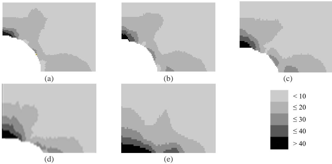
Fig. 5 The stress intensity distribution  $P_u$  [MPa] (1/4 of the plate)
