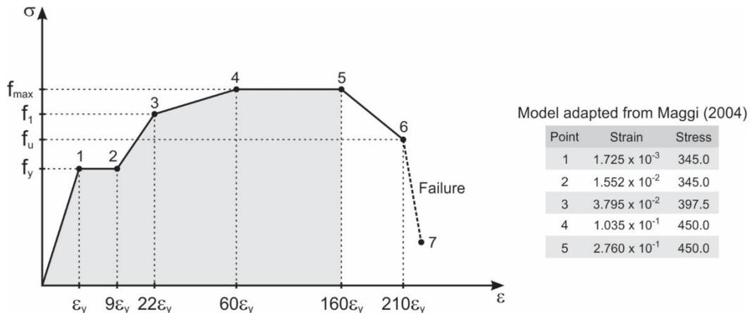
Fig. 6 Multilinear diagram of the steel behavior (adapted from Maggi 2004)
