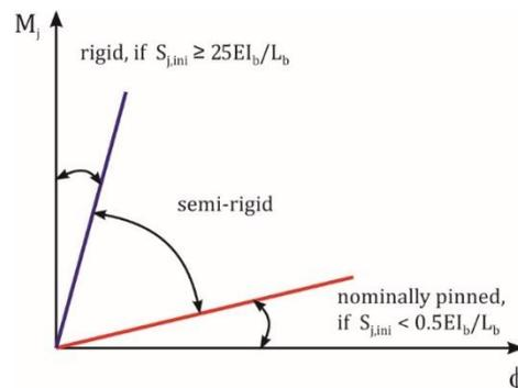
Fig. 2 Limits for stiffness classification of beam-to-column joints for unbraced frames (adapted from Eurocode 3-EN 1993-1-8 2005)
