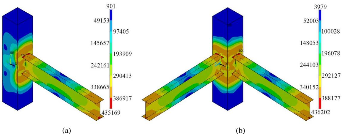
Fig. 11 von Miss stresses for (a) M5-U; (b) M5-M
