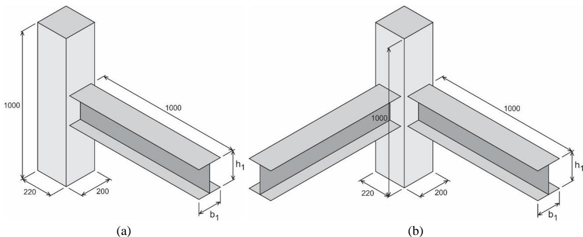
Fig. 4 Geometry and sizes of (a) uniplanar model; (b) multiplanar model. Units in mm
