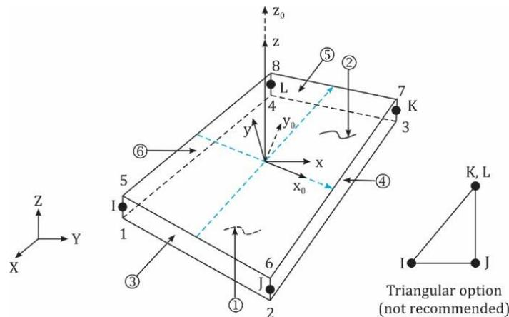
Fig. 5 SHELL181 element (adapted of ANSYS 16.0 2015)
