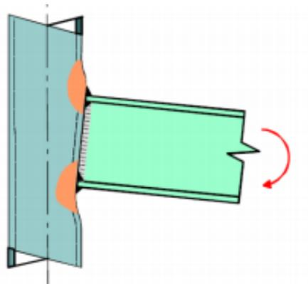
Fig. 3 Column wall plastification (adapted from CIDECT 2010)
