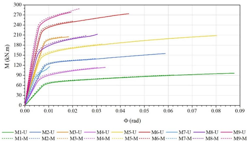
Fig. 9 Bending moment-rotation curves
