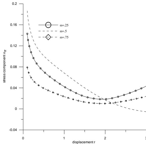
Fig. 6 Variations of radial stress component  $\sigma_{rr}$  with displacement  $r$
