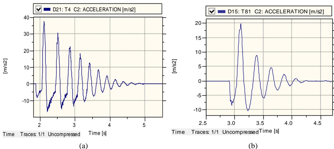
Fig. 4 The sampling signal of acceleration decay curve of tire T2 and TS5 at 150 kPa pressure and 120 mm soil depth (a) For tire; (b) For tire-soil system
