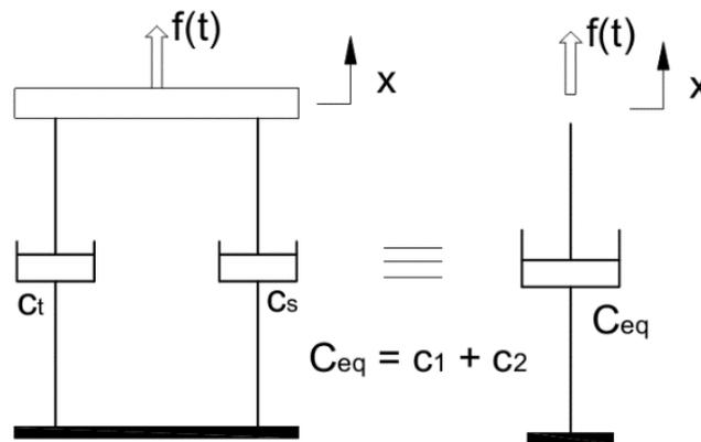
Fig. 10 New damping model of tire-soil system  $c_{eq}$  - equivalent damping coefficient of tire-soil system;  $c_t$  - damping coefficient of tire;  $c_s$  - damping coefficient of paddy soil
