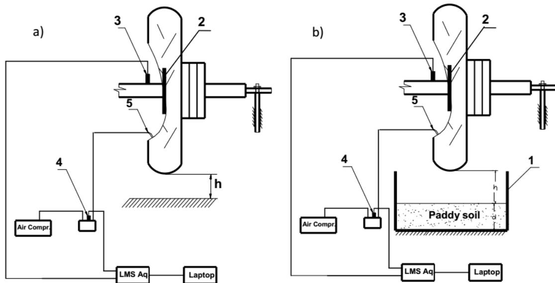
Fig. 1 Sketch of the damping ratio measurement system. (a) Sketch for measurement of vertical damping ratio of tractor tire; (b) Sketch for measurement of damping ratio of tire-soil system. 1. Steel tank; 2. Plate of link tire; 3. Acceleration sensor; 4. Air pressure sensor; 5. Tire valve
