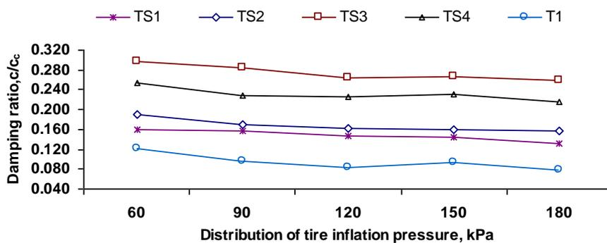
Fig. 7 The vertical equivalent damping ratios of T1, TS1, TS2, TS3 and TS4 tests in soil depth of 120 mm
