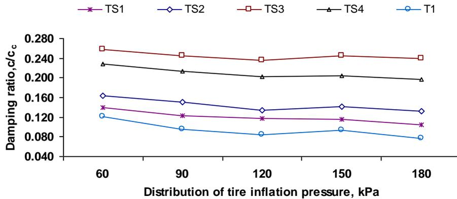
Fig. 6 The vertical equivalent damping ratios of T1, TS1, TS2, TS3 and TS4 test in soil depth of 80 mm
