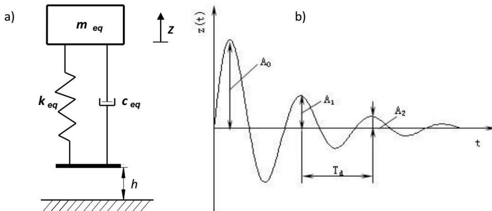
Fig. 2(a) Single degree of freedom system for measuring the vertical equivalent damping ratio of tire and tire-soil system; (b) The decay curve of the free vibration with damping
