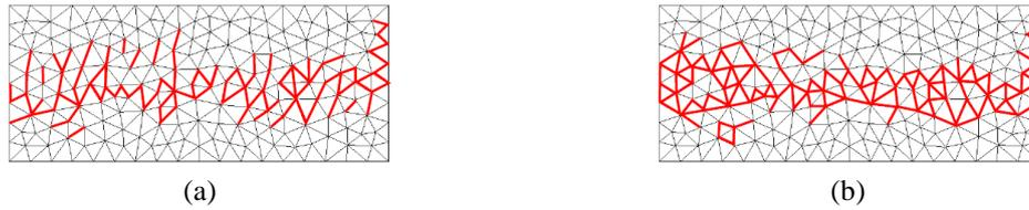
Fig. 5 Elements with increasing damage (a) mode I (b) mode II (note that we mark the cohesive links that are activated by cracks)
