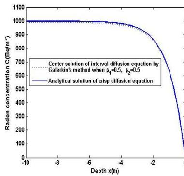
Fig. 2 Comparison of center solution of interval diffusion equation obtained by Galerkins Method when  $\beta_1 = 0.5, \beta_2 = 0.5$  with analytical solution of crisp diffusion equation
