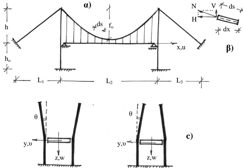
Fig. 3 Schematic of the studied bridge and cable-systems
