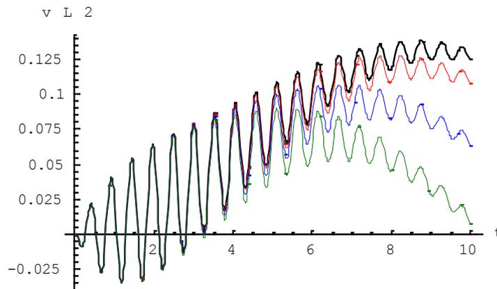
Fig. 8 The influence of angle  $\theta$  on the lateral deflections (m) of the middle of the bridge for  $\theta=0^\circ$ (black),  $\theta=2^\circ$ (red),  $\theta=4^\circ$  (blue) and  $\theta=6^\circ$  (green)
