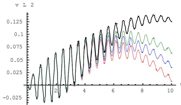
Fig. 9 The influence of sag  $f_0$  on the lateral deflections (m) of the middle of the bridge for  $f_0=120$  m and  $\theta=0^\circ$ (black),  $f_0=120$  m and  $\theta=6^\circ$  (red),  $f_0=100$  m and  $\theta=6^\circ$  (blue) and,  $f_0=80$  m and  $\theta=6^\circ$  (green)
