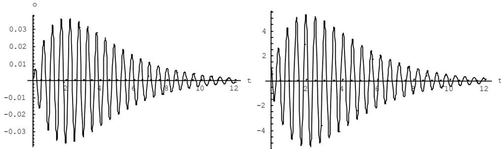
Fig. 7 Soil motion (m) and acceleration (m/s<sup>2</sup>) with respect to time t (s) caused by a distant earthquake
