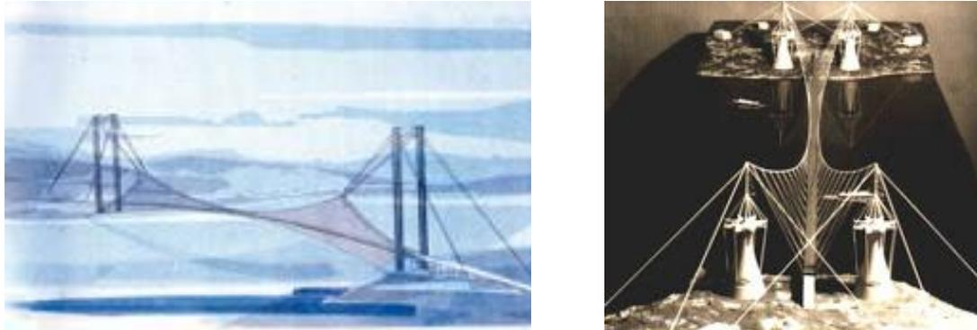
Fig. 1 Nervi's solution with inclined cables
