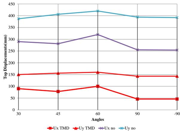
Fig. 11 Lateral displacements of the model with different earthquake exposure angles
