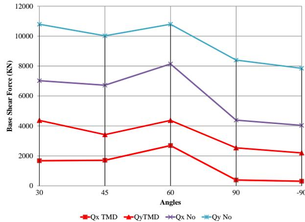
Fig. 12 Base shear in x and y directions of the model with different earthquake exposure angles
