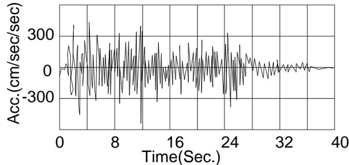
Fig. 2 Accelerograms used for the analyses El Centro
