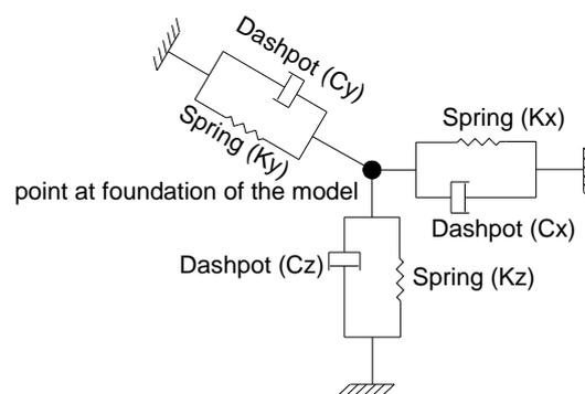
Fig. 4 3D SSI element connected to raft foundation (damper and spring in x, y and z directions)
