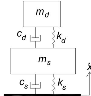
Fig. 5 SDOF system with TMD
