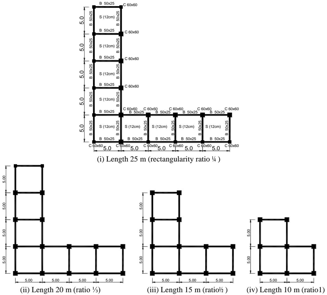
Fig. 1 L-shape in plan HRB with different ratios (rectangularity ratios)
