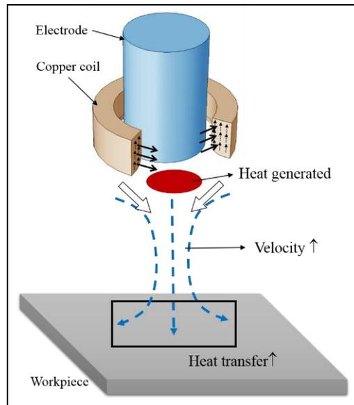
Fig. 8 The diagram of the coil added welding system
