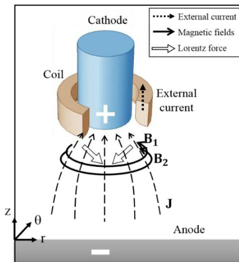
Fig. 7 Conceptual diagram of electromagnetic viewpoint of the coil added welding system
