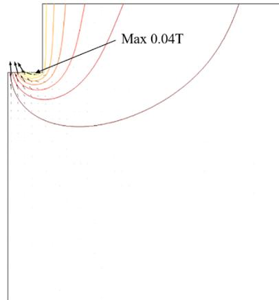
Fig. 3 The azimuthal direction of magnetic flux density (contours, interval: 0.005T) and The current density (arrow line)
