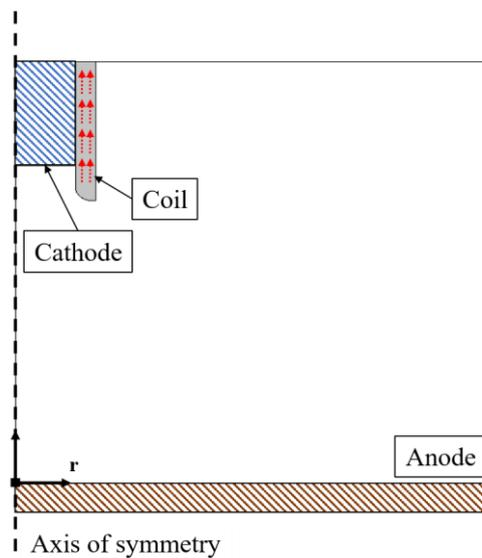
Fig. 9 Computational domain of the coil added system
