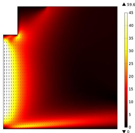
Fig. 4 The velocity fields surface and contours (max: 60, min: 15, interval: 9 m/s)
