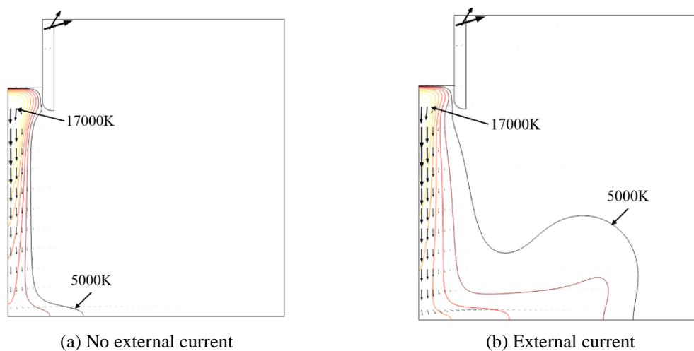
Fig. 13 The isothermal contours (interval: 1500 K) and total heat flux (arrow line)
