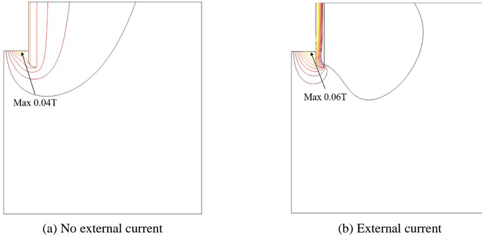
Fig. 10 The azimuthal component of magnetic flux density contours (interval: 0.005 T)
