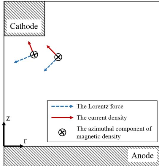
Fig. 6 Schematic figure of interaction between the current density, magnetic density and Lorentz force
