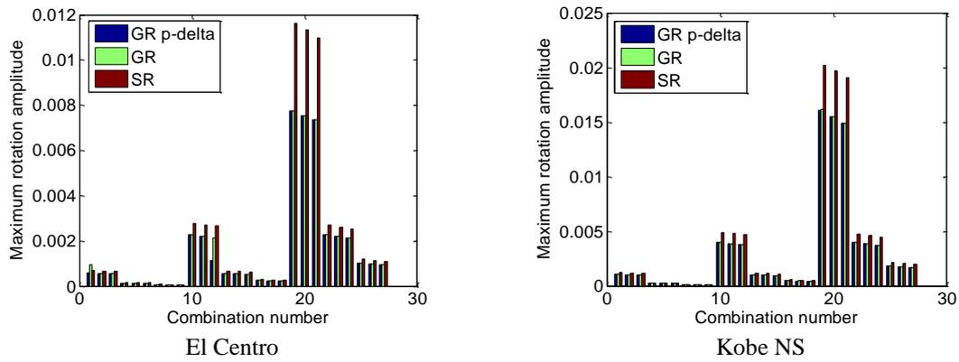
Fig. 7 Variation of maximum rotation as function of the combination number in the case of flexible foundation-mat on Winkler foundation type; (GR p-delta) designates great rotation with p-delta effect; (GR) great rotation without p-delta effect and (SR) small rotation
