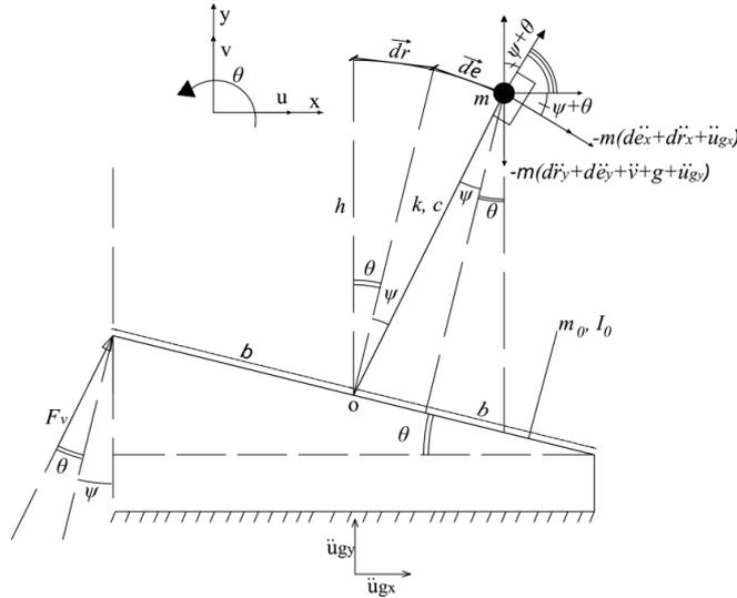
Fig. 5 Free body diagram of the system with uplift showing the considered dependent and independent degrees of freedom
