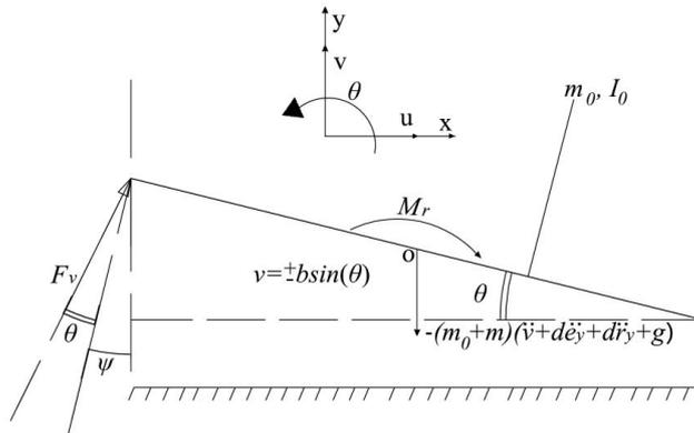
Fig. 6 Free body diagram of the system with uplift showing the considered dependent and independent degrees of freedom
