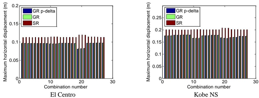
Fig. 8 Variation of maximum horizontal displacement as function of the combination number in the case of flexible foundation-mat on Winkler foundation type; (GR p-delta) designates great rotation with p-delta effect; (GR) great rotation without p-delta effect and (SR) small rotation
