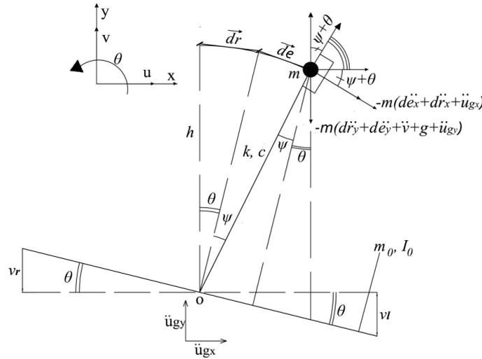
Fig. 2 Free body diagram of the system with uplift showing the considered dependent and independent degrees of freedom
