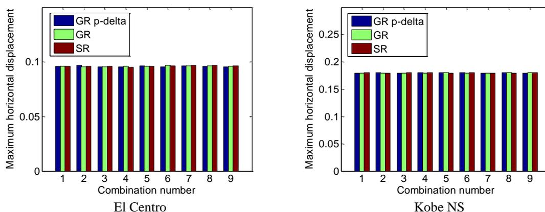
Fig. 10 Variation of maximum horizontal displacement as function of the combination number in the case of flexible foundation-mat on rigid soil; (GR p-delta) designates great rotation with p-delta effect; (GR) great rotation without p-delta effect and (SR) small rotation
