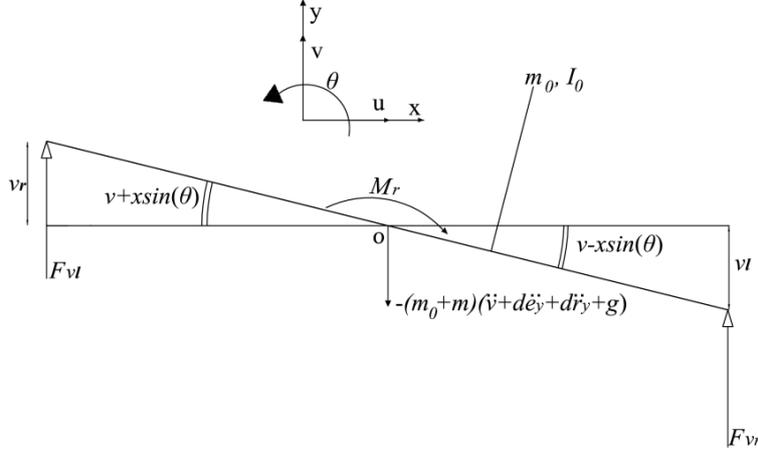
Fig. 3 Free body diagram for the base
