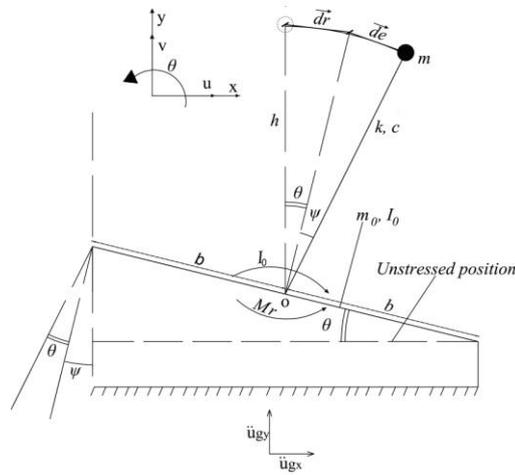
Fig. 4 Flexible structure on rigid soil
