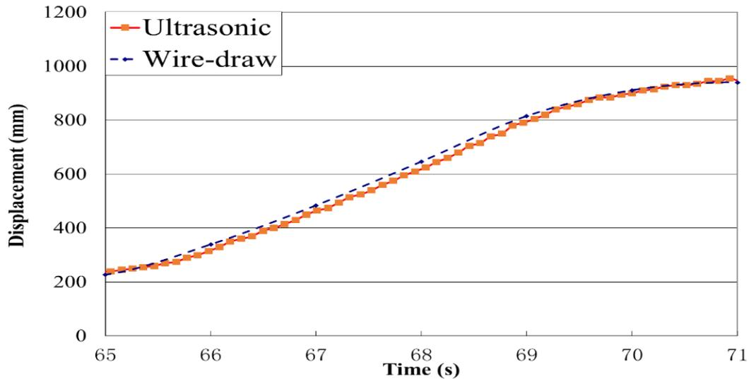
Fig. 12 Displacement measured by the ultrasonic and the wire draw sensing systems (65s to 71s)
