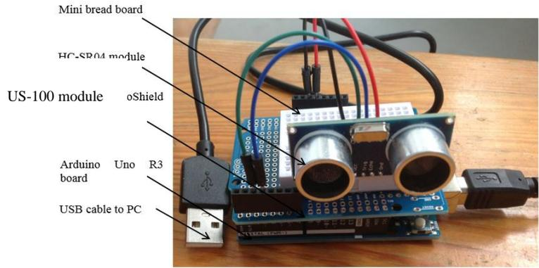
Fig. 1 An Ultrasonic sensing system with US-100 module
