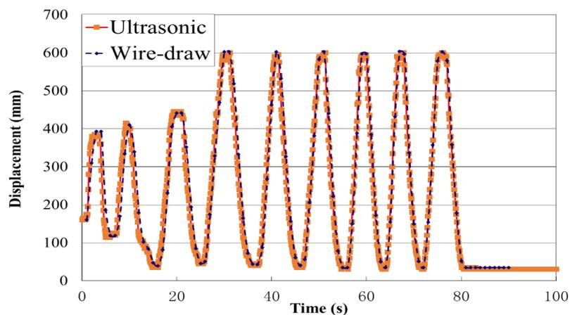
Fig. 6 Displacement measured by the ultrasonic and the wire draw sensing systems
