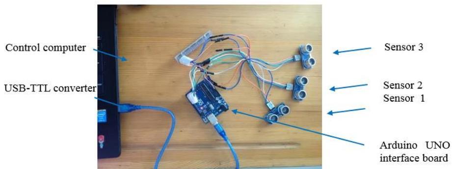
Fig. 2 Ultrasonic distance sensing system with three distance sensors
