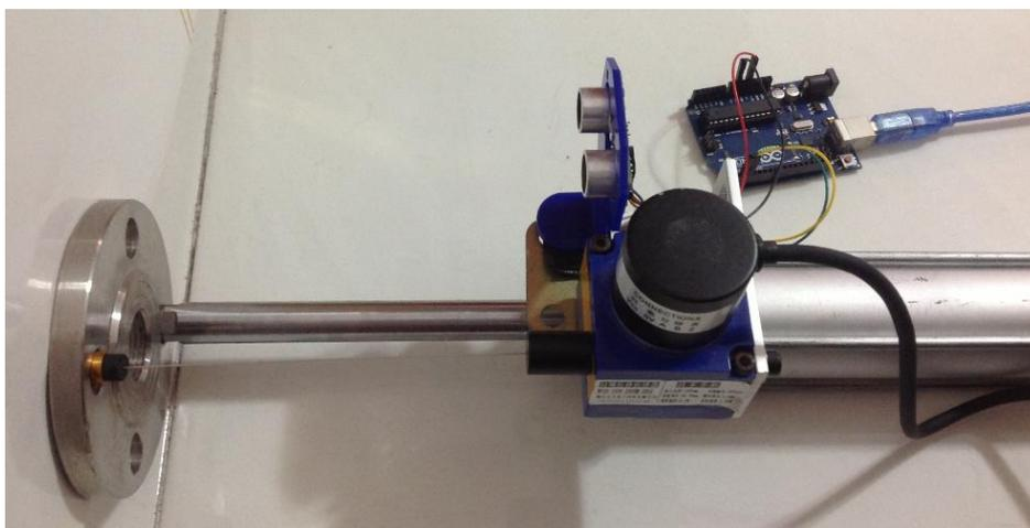
Fig. 5 Experimental setup of ultrasonic and wire draw sensing systems
