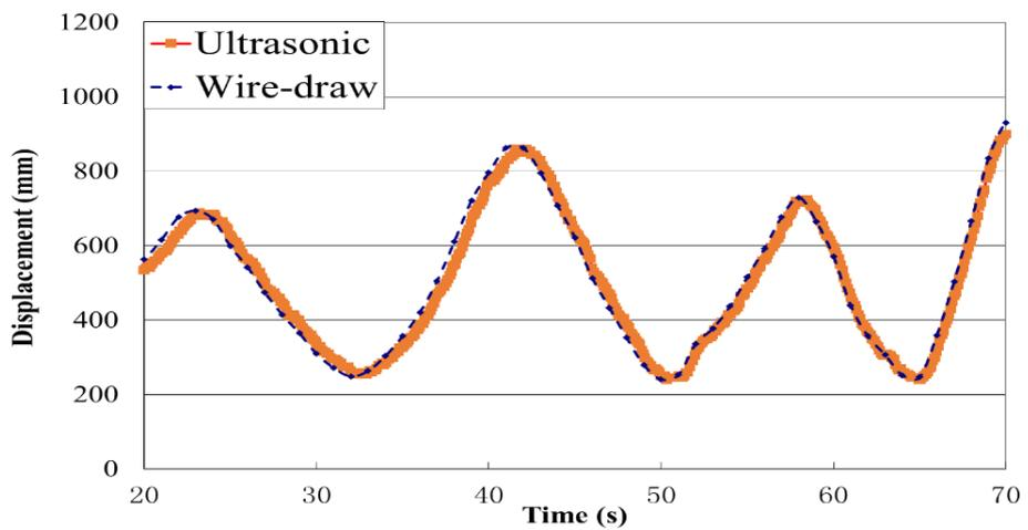
Fig. 11 Displacement measured by the ultrasonic and the wire draw sensing systems (20s to 70s)
