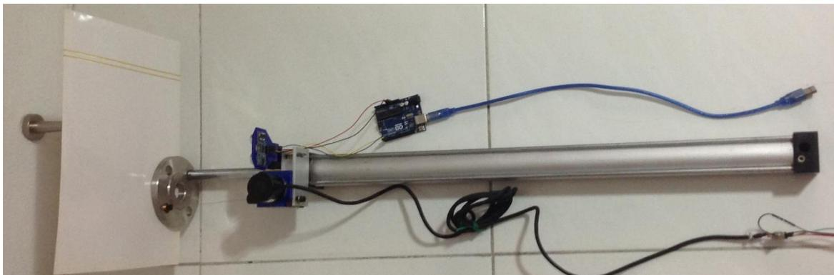
Fig. 4 Experimental setup to measure the translational motion of a cylinder using ultrasonic and wire draw sensing systems
