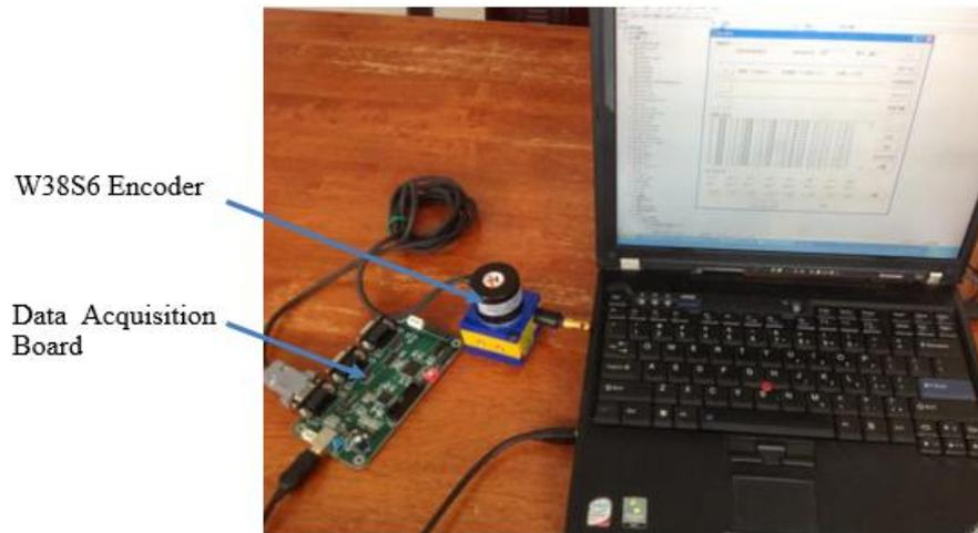
Fig. 3 W38S6 Wire draw Encoder system
