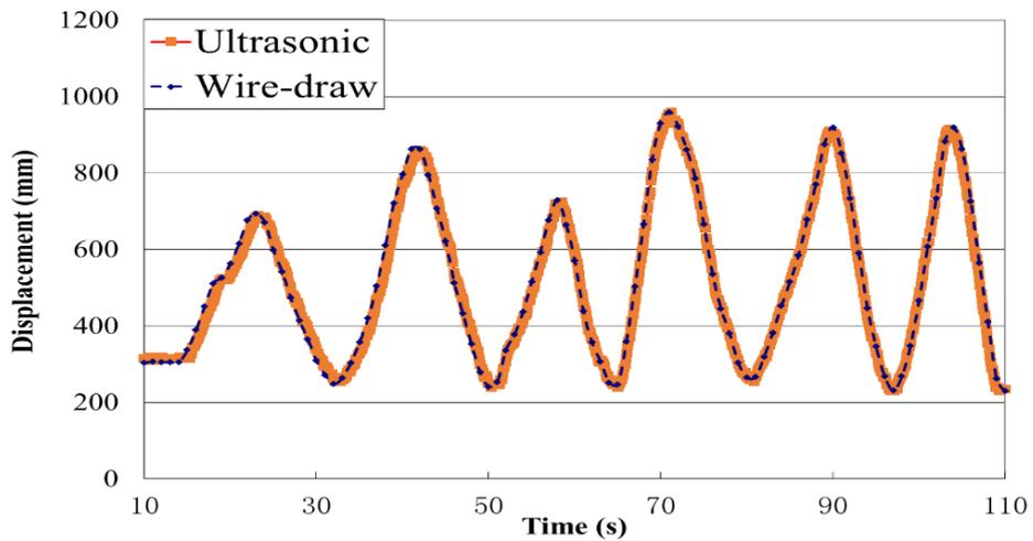
Fig. 10 Displacement measured by the ultrasonic and the wire draw sensing systems (mini-car)
