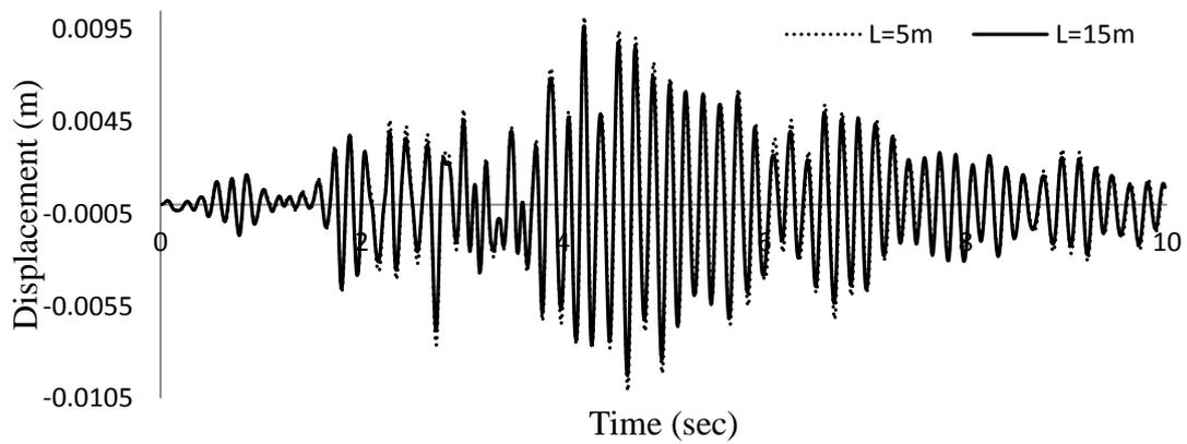
Fig. 7 Tip displacement of separator wall due to Koyna earthquake
