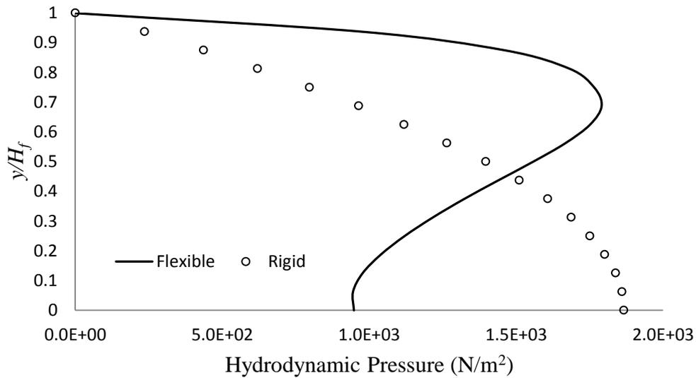
Fig. 11 Hydrodynamic pressure along the separator wall at  $t = 4.20$  sec for  $L = 15$  m
