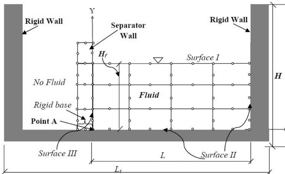
Fig. 1 A typical finite element discretization of tank-water system
