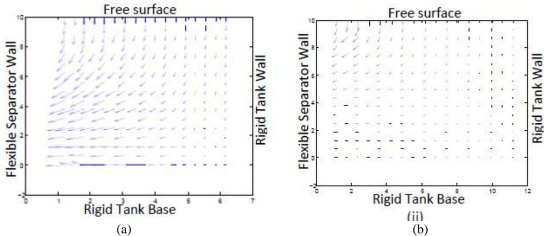
Fig. 13 Velocity vectors at  $t = 4.20$  sec in fluid for (a)  $L = 5$  m and (b)  $L = 15$  m
