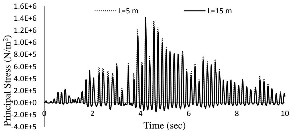
Fig. 8 Major Principal stress at the base of the separator wall due to Koyna earthquake
