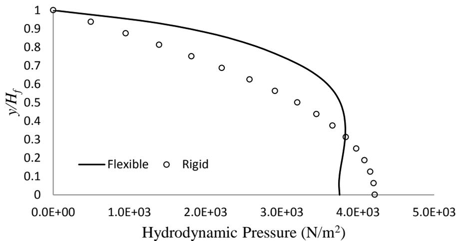
Fig. 10 Hydrodynamic pressure along the separator wall at  $t = 4.20$  sec for  $L = 5$  m
