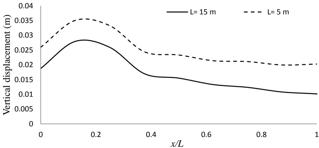
Fig. 12 Sloshed displacement for different length of tank at  $t = 4.20$  sec
