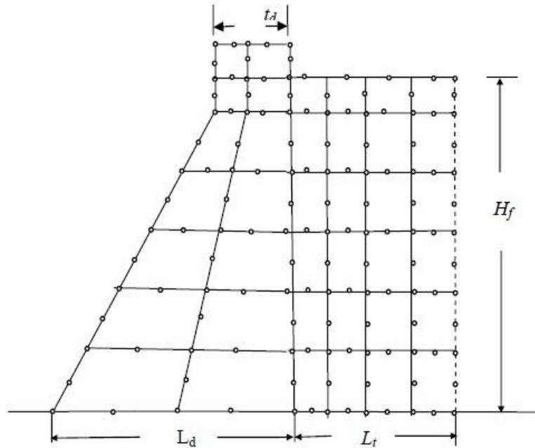
Fig. 3 Finite element mesh of dam-reservoir system
