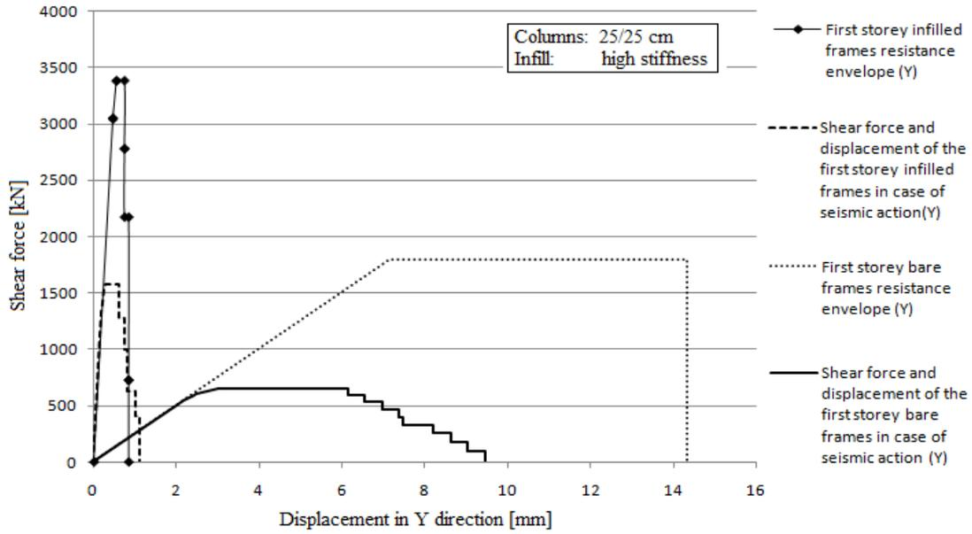
Fig. 13 Comparison of the resistance envelope and required resistance in case of seismic action with PGA = 0,1 g of the first storey frames in Y direction with and without the infill
