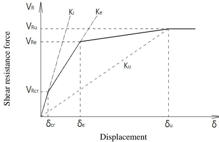
Fig. 9 Trilinear idealisation of an infilled frame behavior by Žarnić (1994)
