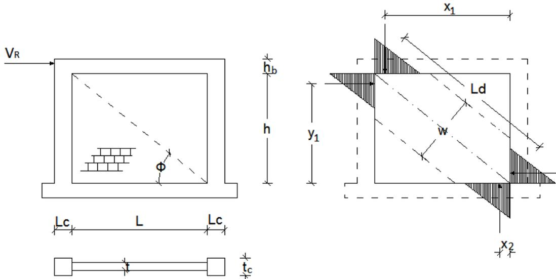
Fig. 10 model of masonry infilled frame and idealized stresses in the corners of compression strut
