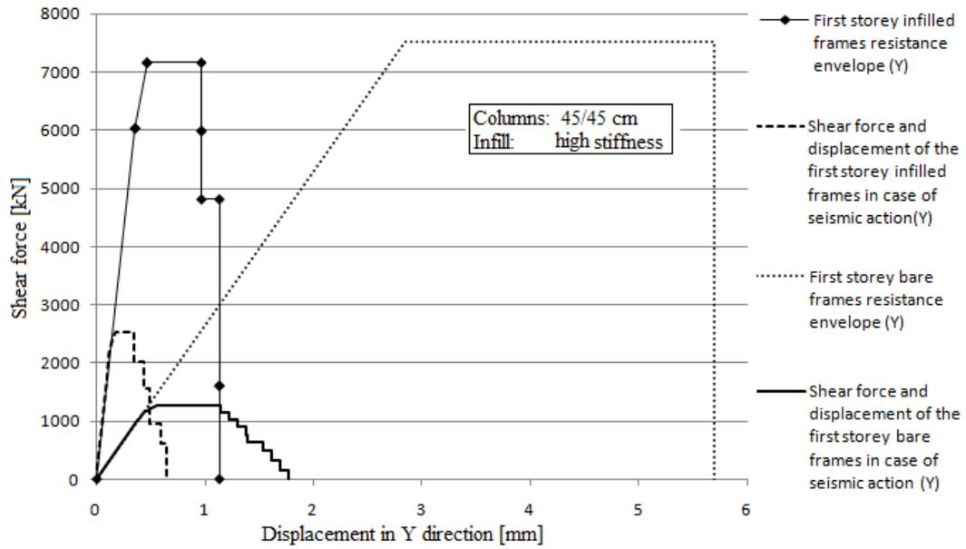
Fig. 15 Comparison of the resistance envelope and required resistance in case of seismic action with PGA = 0,1 g of the first storey frames in Y direction with and without the infill
