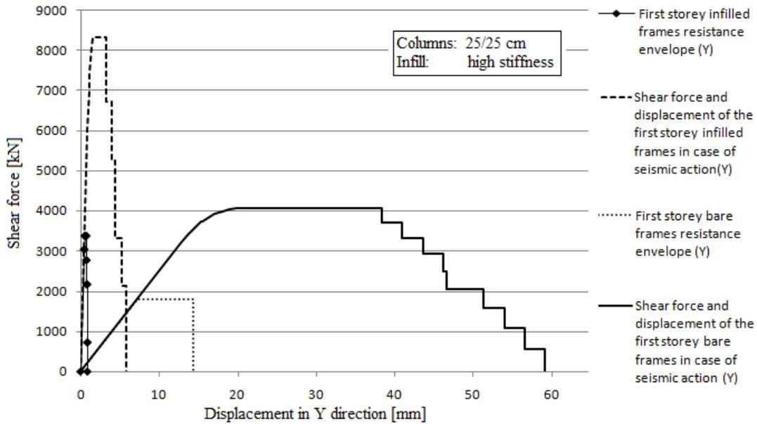
Fig. 17 Comparison of the resistance envelope and required resistance in case of seismic action with PGA = 0,4 g of the first storey frames in Y direction with and without the infill
