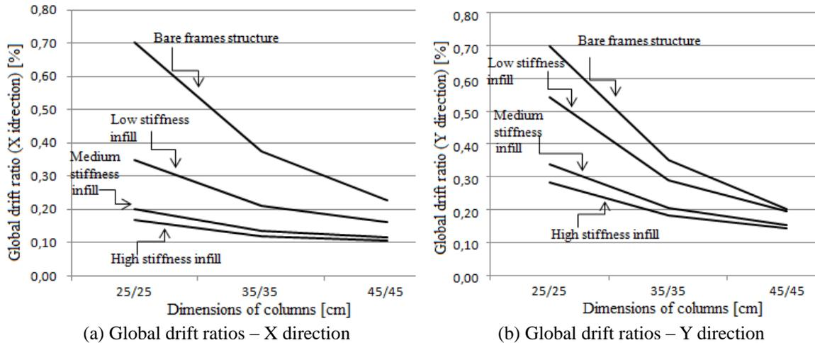
Fig. 8 Comparison of the global drift ratios of frame structure with different column dimensions without infill and with different stiffness infills
