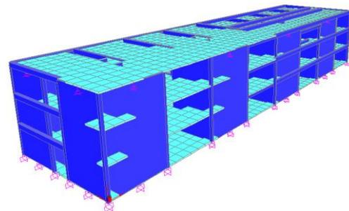
(b) Masonry infilled r.c. frames structure
