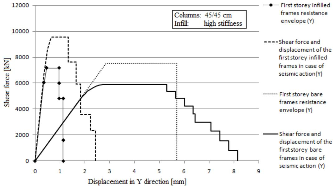
Fig. 19 Comparison of the resistance envelope and required resistance in case of seismic action with PGA = 0,4 g of the first storey frames in Y direction with and without the infill
