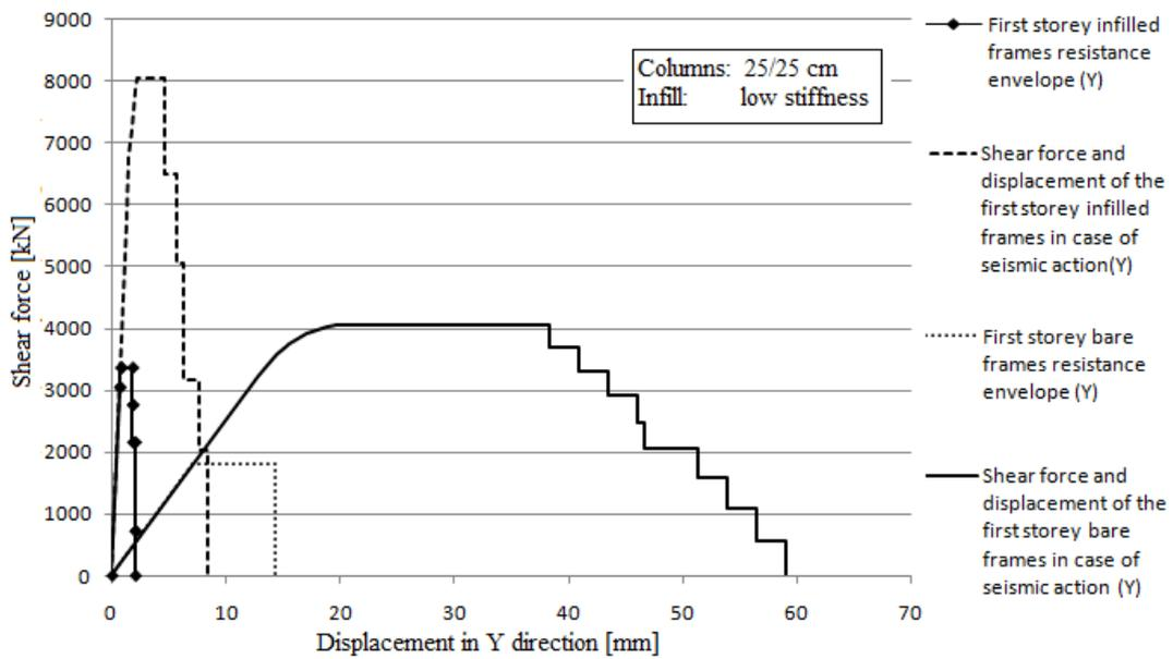
Fig. 16 Comparison of the resistance envelope and required resistance in case of seismic action with PGA = 0,4 g of the first storey frames in Y direction with and without the infill
