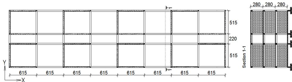
Fig. 5 Building layout and disposition of the masonry infill walls
