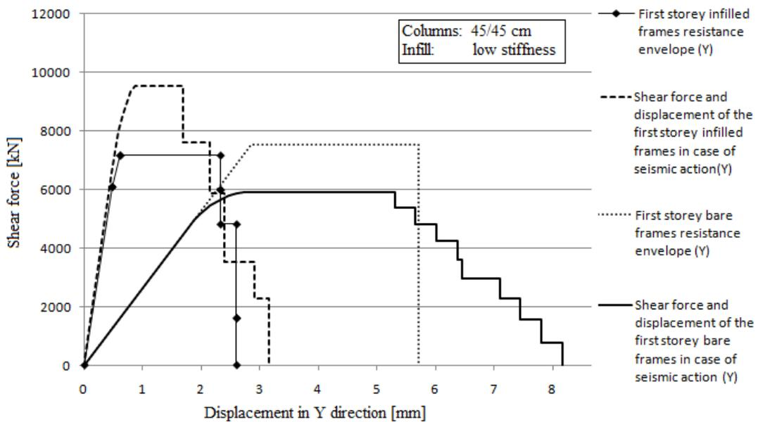
Fig. 18 Comparison of the resistance envelope and required resistance in case of seismic action with PGA = 0,4 g of the first storey frames in Y direction with and without the infill
