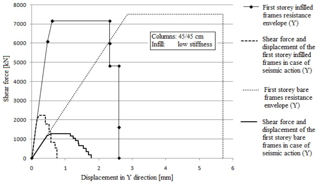
Fig. 14 Comparison of the resistance envelope and required resistance in case of seismic action with PGA = 0,1 g of the first storey frames in Y direction with and without the infill
