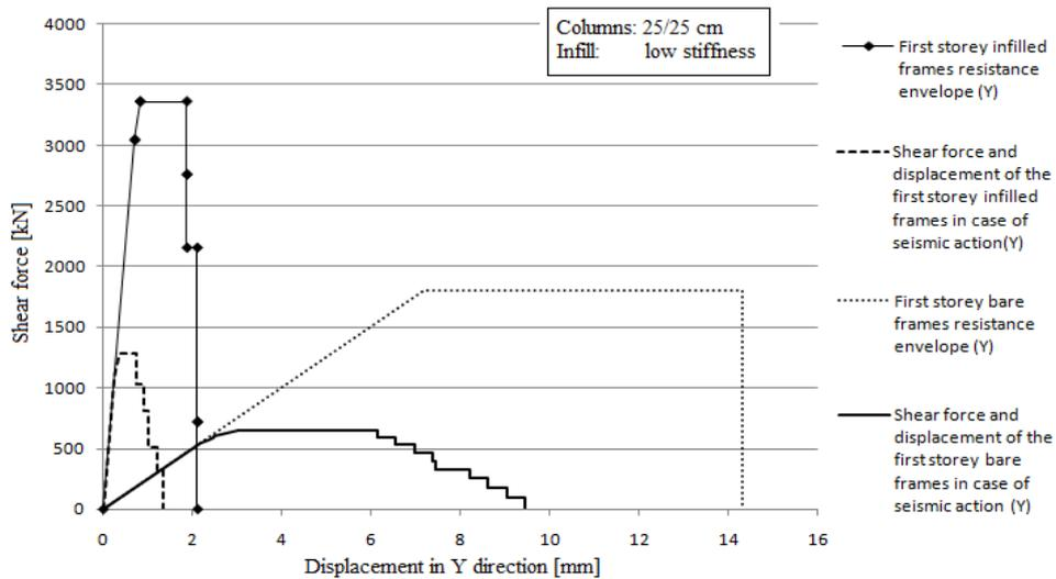
Fig. 12 Comparison of the resistance envelope and required resistance in case of seismic action with  $PGA = 0,1\text{ g}$  of the first storey frames in Y direction with and without the infill
