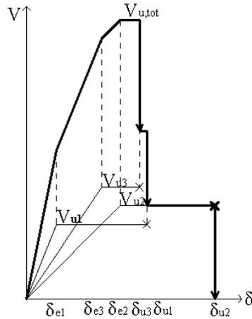
Fig. 11 Construction of the storey resistance envelope by Tomažević (1999)
