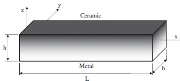
Fig. 1 Geometry and coordinate of a FG beam
