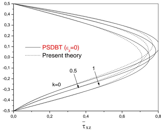
Fig. 4 The variation of the transverse shear stress  $\bar{\tau}_{xz}$  through-the-thickness of a FG beam ( $L = 2h$ )
