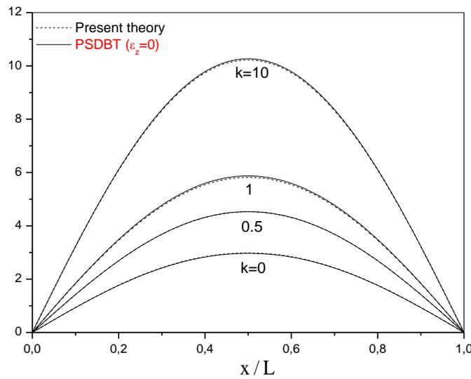
Fig. 5 Variation of the transverse displacement  $\bar{w}$  versus non-dimensional length of a FG beam ( $L = 5h$ )
