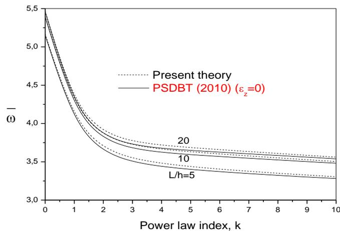
Fig. 6 Variation of the nondimensional fundamental frequency  $\bar{\omega}$  of FG beam with power law index  $k$  and span-to-depth ratio  $L/h$
