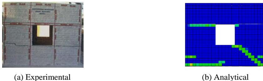
Fig. 18 Comparison of damage on south side wall after sixth shock (Horizontal cracks originating from the window opening appeared on the southern shear walls)
