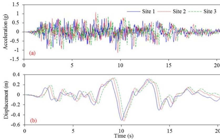
Fig. 2 Simulated ground motions: (a) Accelerations and (b) displacements for highly correlated excitations under soft soil conditions
