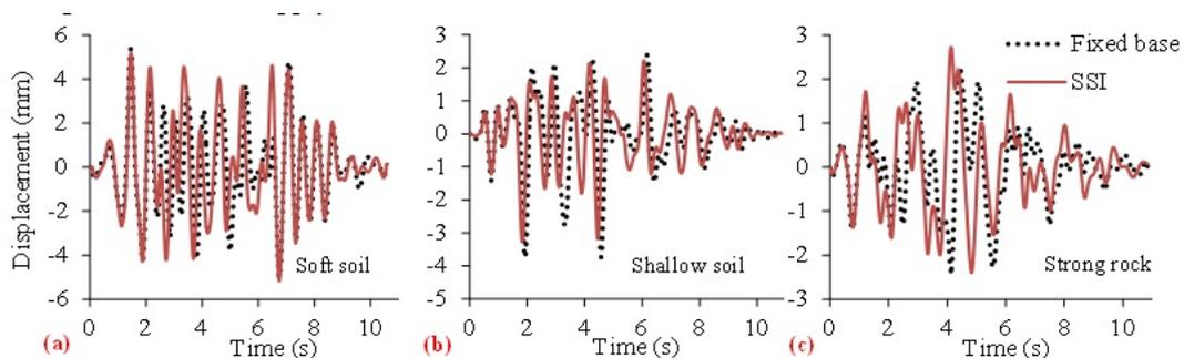
Fig. 6 Absolute displacements of segment 1, with and without SSI, for ground motions of (a) soft soil, (b) shallow soil, and (c) strong rock conditions
