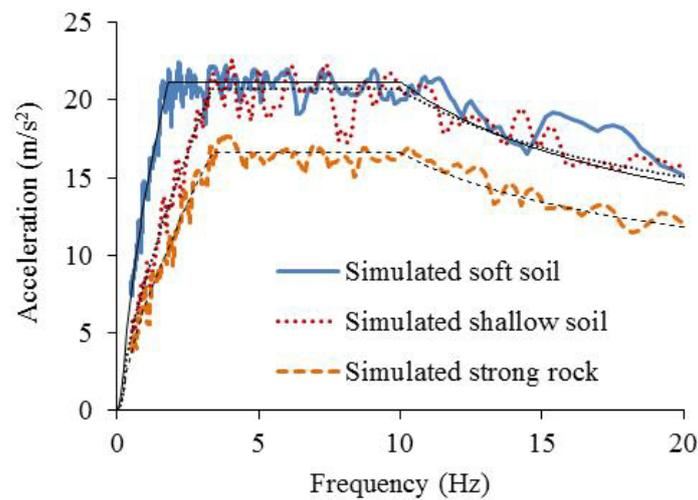
Fig. 3 The response spectra of the simulated ground motions (thick lines) and the target design spectra (thin lines)
