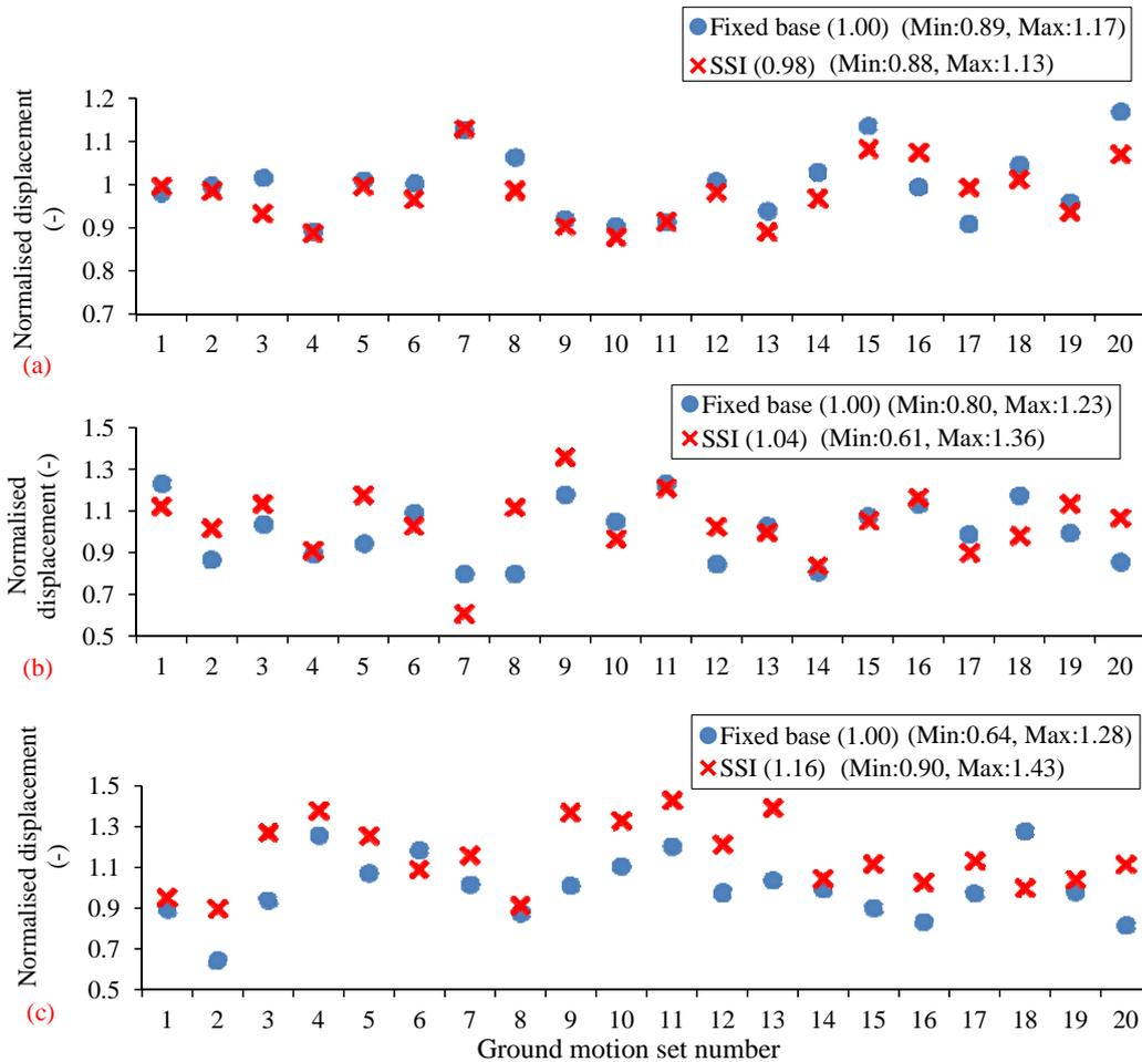
Fig. 7 Consequences of SSI for the normalised maximum absolute displacements of segment 1, without pounding, due to the ground motions of (a) soft soil, (b) shallow soil, and (c) strong rock conditions
