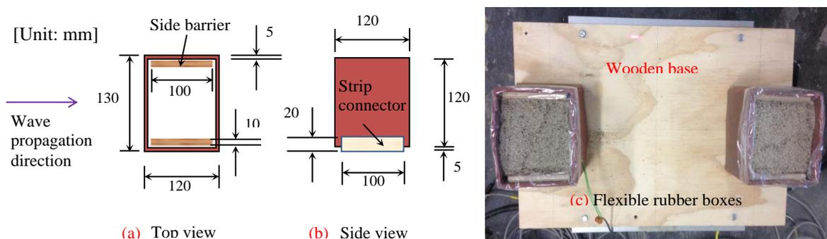
Fig. 4 Flexible rubber boxes: (a) Top view, (b) side view, and (c) top view of boxes filled with sand
