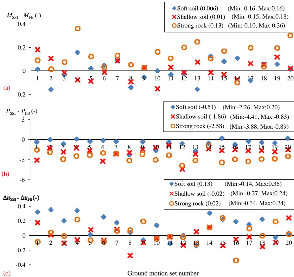
Fig. 11 Consequence of SSI and excitation soil conditions for the maximum values of the normalised (a) bending moment of pier 2A, (b) pounding force, and (c) relative opening displacement between segments 2 and 3
