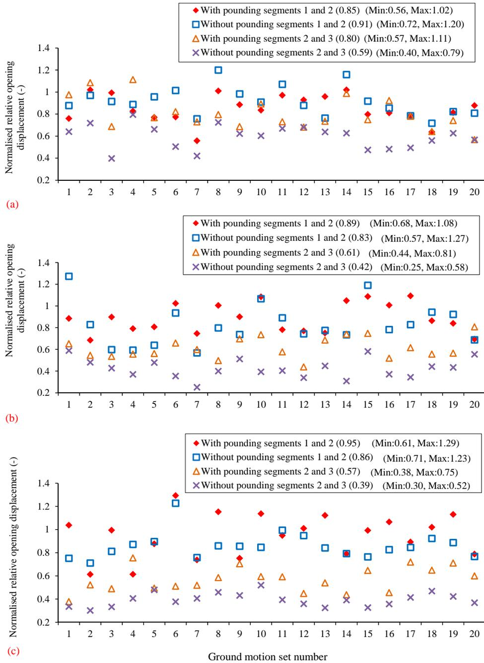
Fig. 13 Consequence of pounding and SSI for the normalised relative opening displacements between different segments, for(a) soft soil, (b) shallow soil and (c) strong rock conditions
