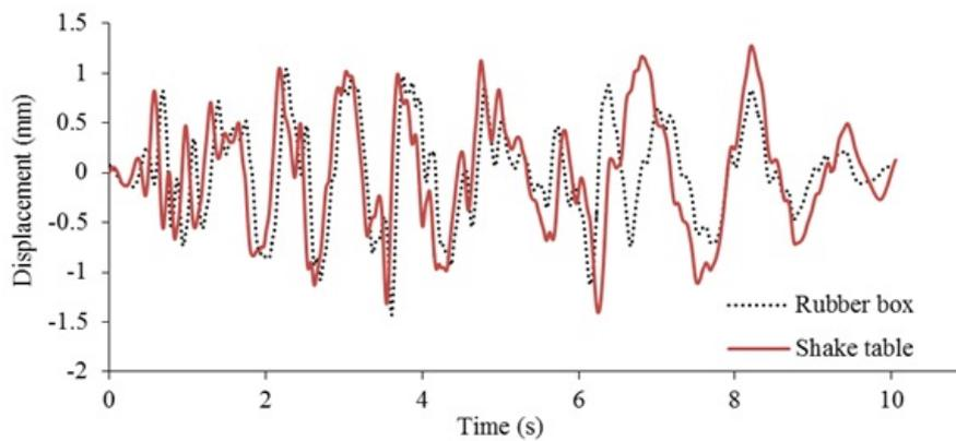
Fig. 5 Comparison of displacements of the rubber box (box 1A, see Fig. 1) and the shake table, subjected to the same highly correlated ground motion associated with the strong rock condition
