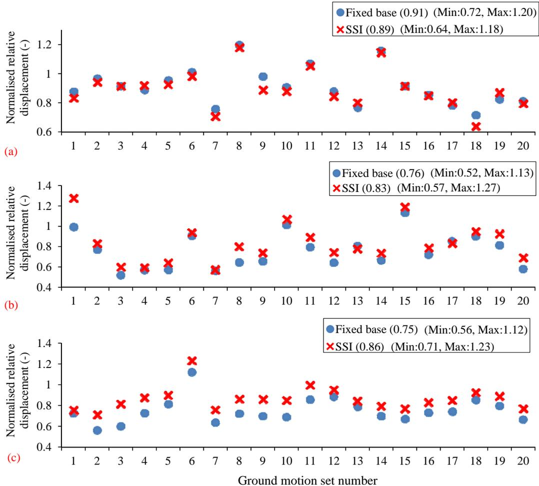
Fig. 8 Consequences of SSI for the normalised maximum relative opening displacements between segments 1 and 2, without pounding effects. Results for highly correlated ground motions of (a) soft soil, (b) shallow soil, and (c) strong rock conditions
