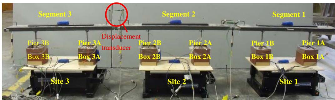
Fig. 1 Setup of the test system with rubber sandboxes
