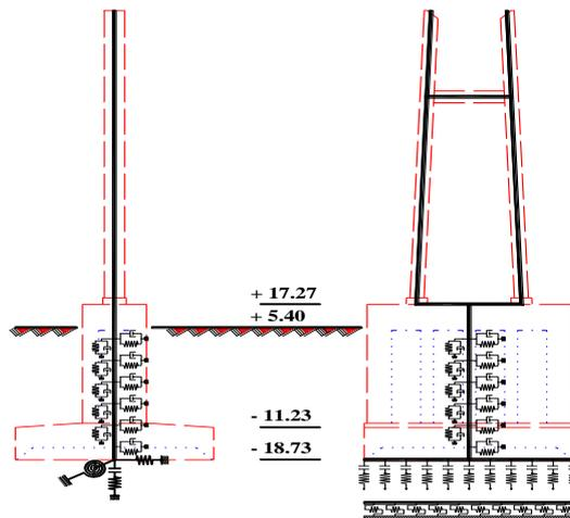
Fig. 9 Hybrid tower model
