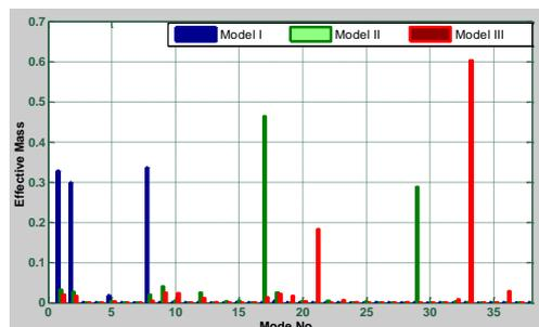
Fig. 11 Modal effective mass ratio for the first 50 Eigen modes of the different tower models.
