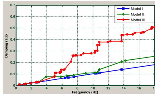
Fig. 12 Modal damping ratio for different tower models
