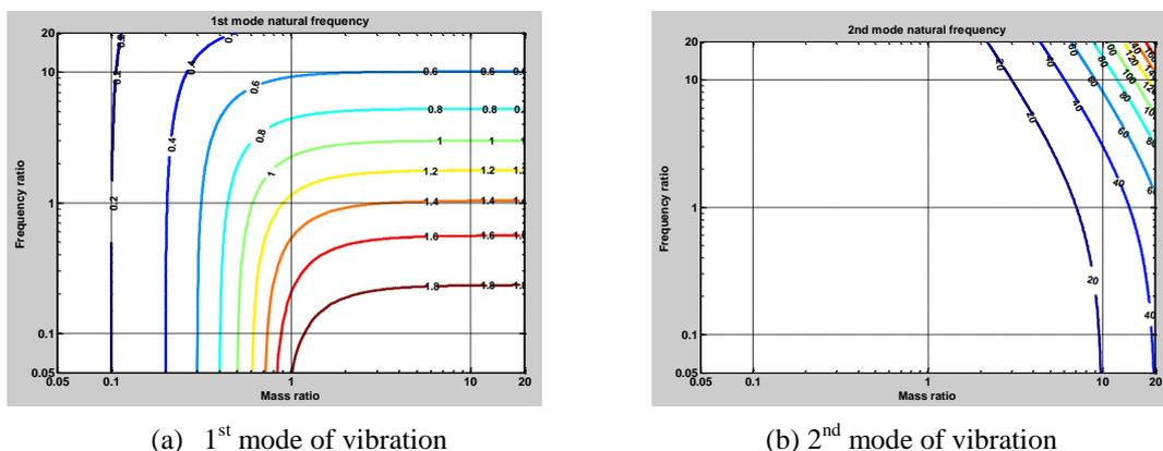
Fig. 7 Natural frequency variation with mass/frequency ratio ( $\zeta_1 = 0.02/0.20$ ,  $\zeta_2 = 0.02$ )
