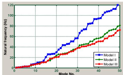
Fig. 10 Natural frequencies for the first 50 Eigen modes of the different tower models
