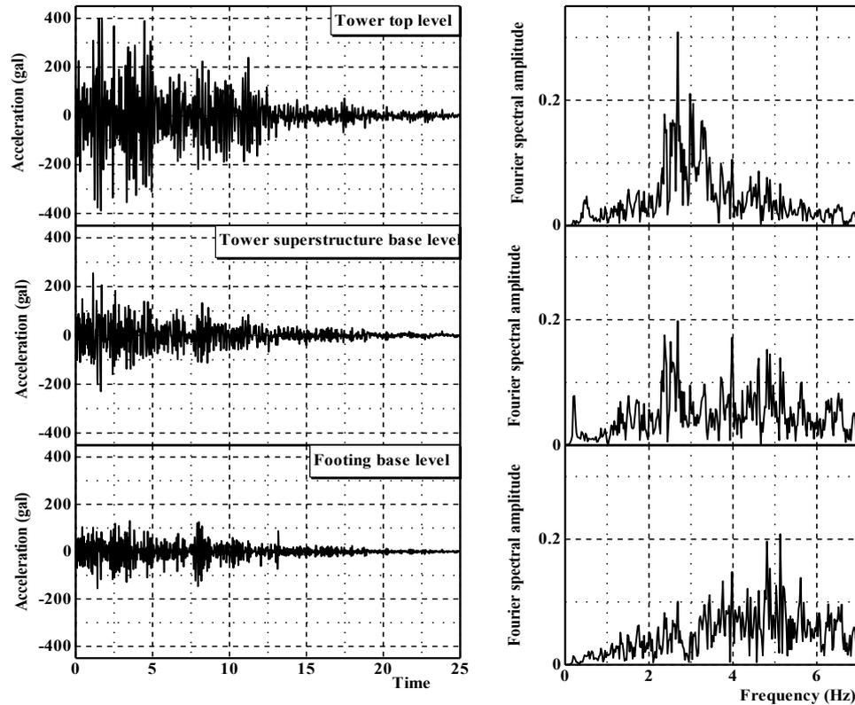
Fig. 14 Vertical acceleration time history and response spectra
