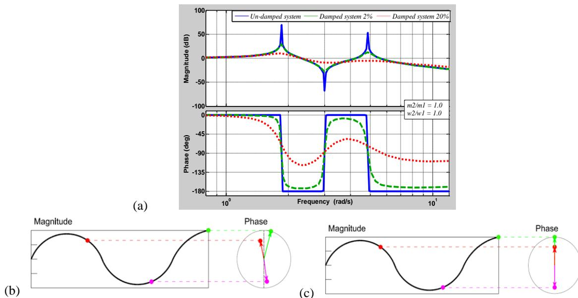
Fig. 2 Frequency response function: (a) damping effect on vibration modes; (b) Classical (real normal) mode schematic and (c) Non-classical (complex) mode schematic
