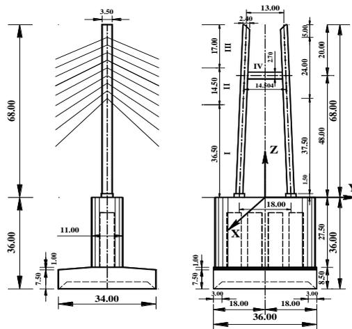
Fig. 8 Tower structure of cable-stayed bridge (m)
