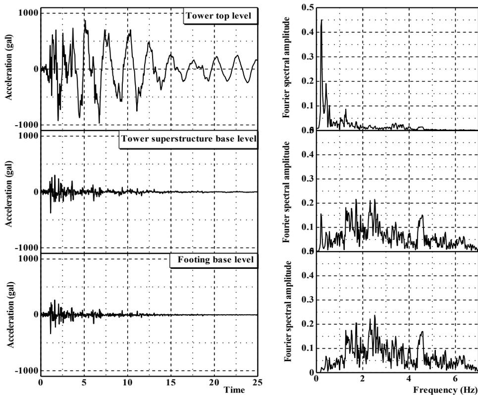
Fig. 13 In-plane acceleration time history and response spectra
