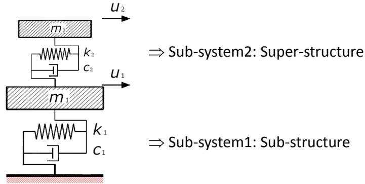
Fig. 1 2-DOF simplified tower model
