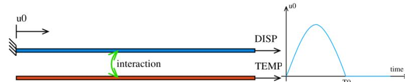
Fig. 4 One-dimensional thermomechanical test
