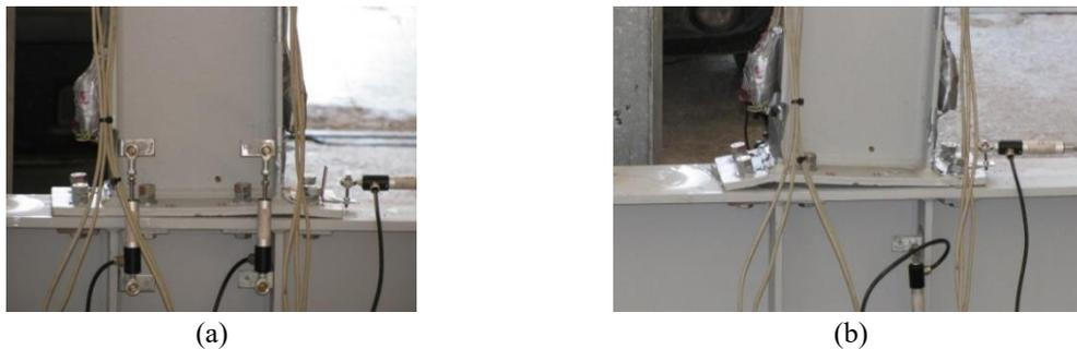
Fig. 1 Deformation of the connection during a cyclic loading
