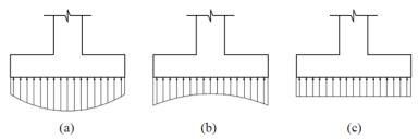
Fig. 1 Pressure distribution diagram; (a) Sandy soils (granular soils); (b) Clayey soils (cohesive soils); (c) Distribution simplified
