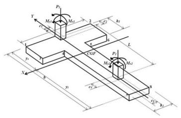
Fig. 6 T-shaped combined footing
