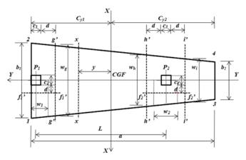
Fig. 4 Critical sections for bending shear
