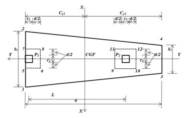
Fig. 5 Critical sections for punching shear
