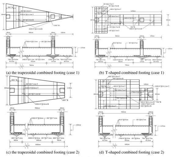
Fig. 10 Final design for the four footings
