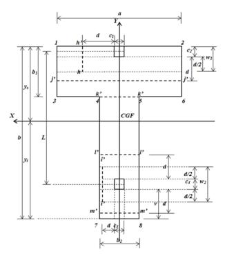
Fig. 8 Critical sections for bending shear
