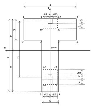
Fig. 9 Critical sections for punching shear
