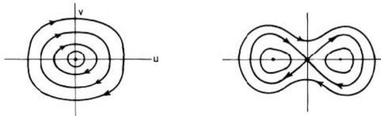
Fig. 6 Phase space representation of Duffing oscillator for non-damped case ( $\delta = 0$ ) in free vibrations ( $\gamma = 0$ ) with  $\beta \geq 0$  (left) and  $\beta < 0$  (right)
