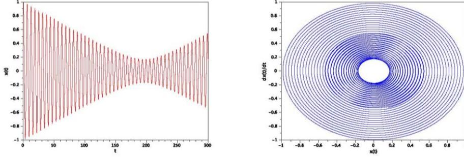
Fig. 9 Computed solution (left) and phase space (right) for Duffing oscillator with numerical values of parameters in (6) chosen as:  $\omega_0=\delta=\alpha=1$  and  $\varepsilon=0.01$
