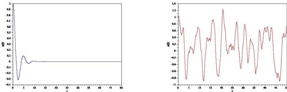
Fig. 10 Response of Duffing oscillator under deterministic load (left) and white noise (right)
