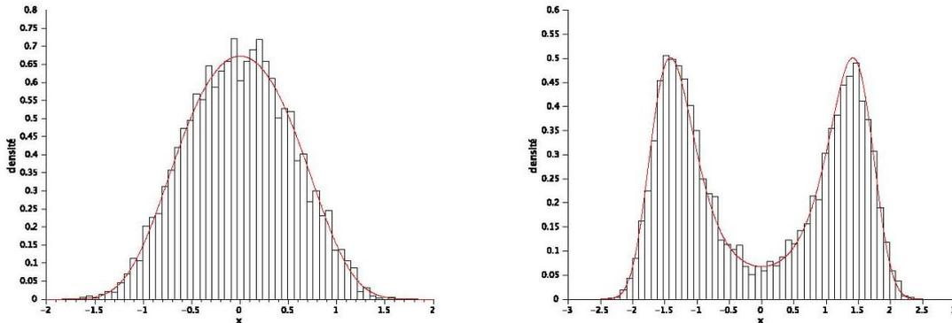
Fig. 11 Stationary solution for system in (14), with exact (red line) and numerical (histogram) with parameters values  $\delta=\alpha=\beta=\eta=1$  (left) vs.  $\delta=\alpha=\eta=1$  and  $\beta=-2$  (right)
