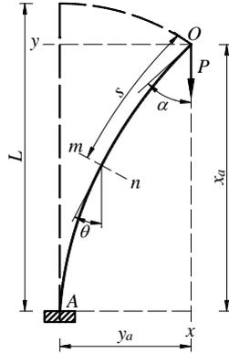
Fig. 3(a) Geometrically exact Euler beam under compressive fixed load-geometry and load
