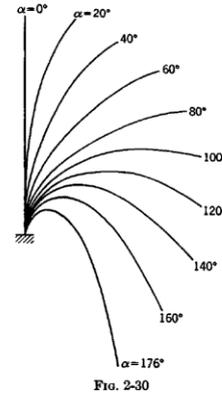
Fig. 3(b) Geometrically exact Euler beam under compressive fixed load-deformed shapes
