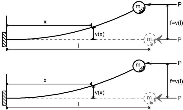
Fig. 5 Euler-Bernoulli cantilever beam vibrations under fixed load ( $v(x,t)$   $P_x=P$ ,  $P_y=0$ )
