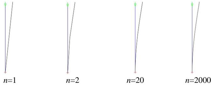
Fig. 4 The first buckling mode for different meshes
