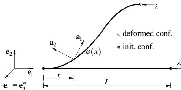
Fig. 2 Nonlinear instability of geometrically exact Euler cantilever beam
