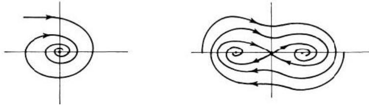
Fig. 7 Phase space representation of Duffing oscillator for damped case ( $\delta > 0$ ) in free vibrations ( $\gamma = 0$ ) with  $\beta \geq 0$  (left) and  $\beta < 0$  (right)
