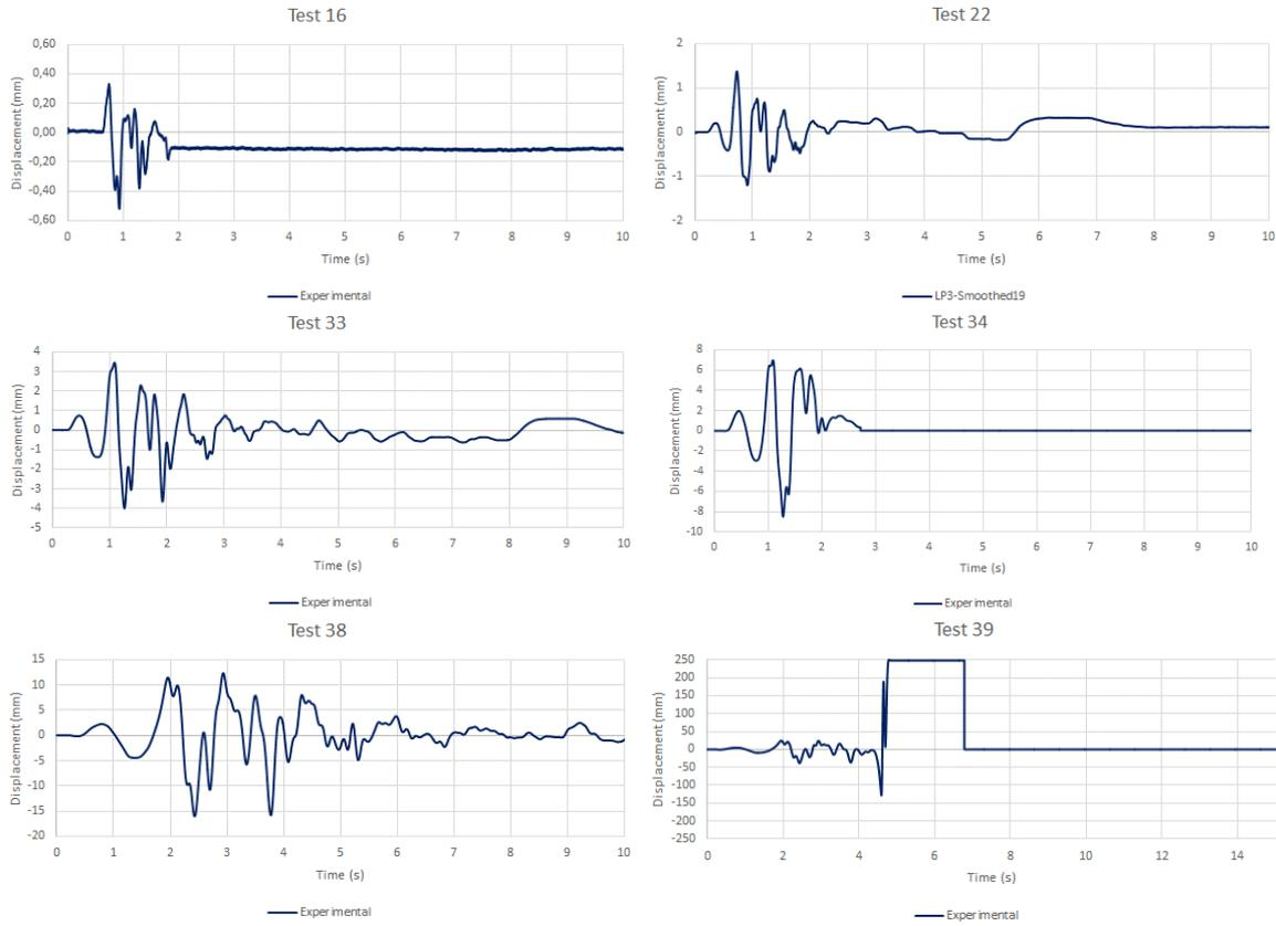
Fig. 14 Time histories for the horizontal displacements at the top of the arch
