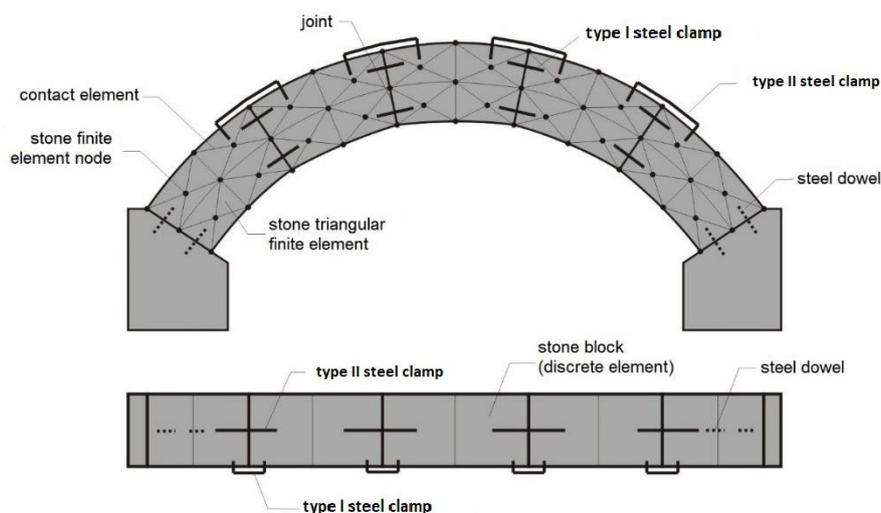
Fig. 15 Discretisation of a stone arch with installed clamps and dowels [11]
