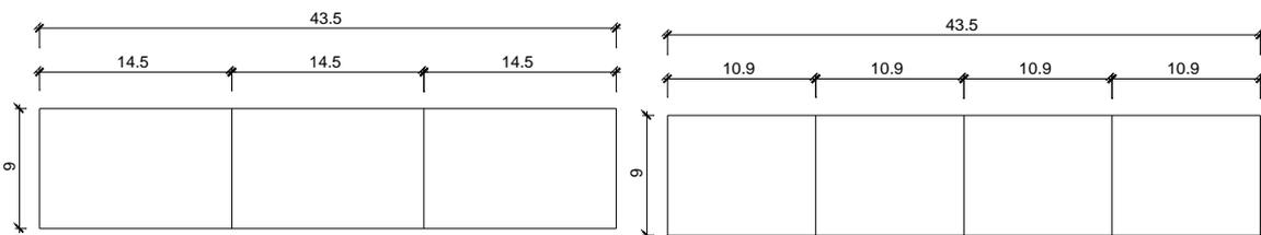
Fig. 8 The arrangement of the vault (cm)
