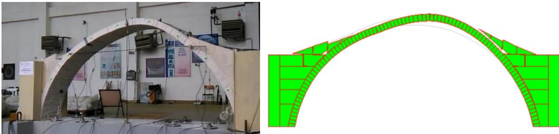
Fig. 20 Mode shapes and failure mechanism for Test\_39—initial cracks
