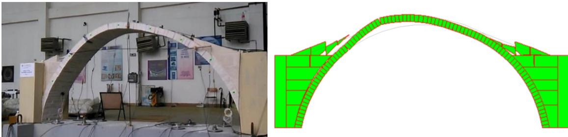
Fig. 21 Mode shapes and failure mechanism for Test\_39—crack development
