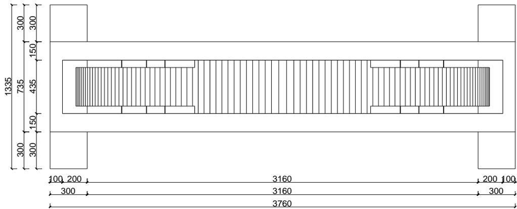
Fig. 6 Geometry of the model of the Old Bridge – top view (cm)
