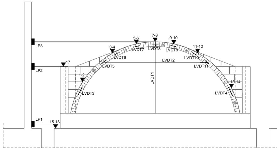
Fig. 12 Position of LPs (1-3), position of LVDT (1-11), position of accelerometers (1-17)
