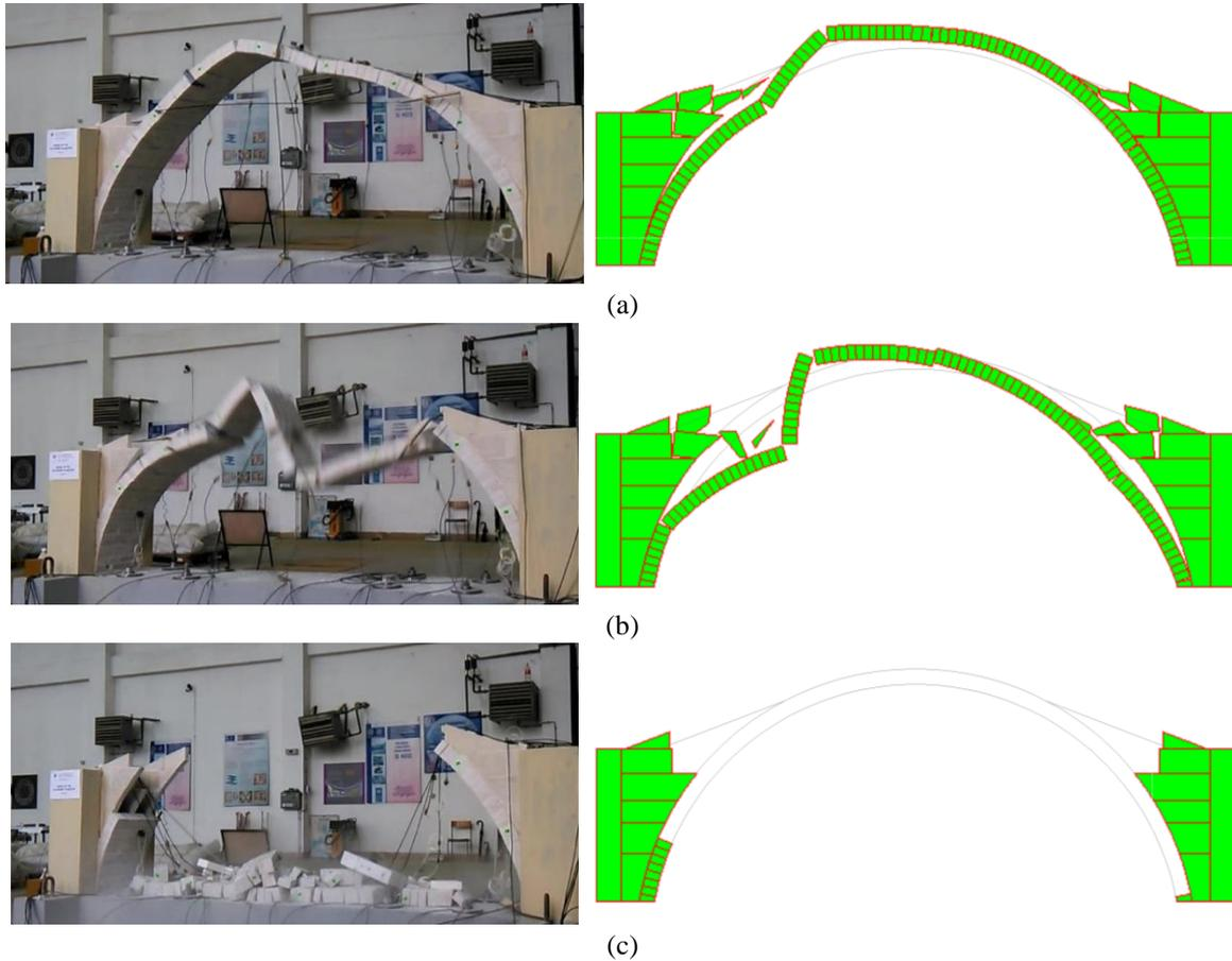
Fig. 22 Mode shapes and failure mechanism for Test\_39—collapse of the model
