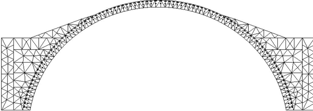
Fig. 16 Discretisation of the Old Bridge model
