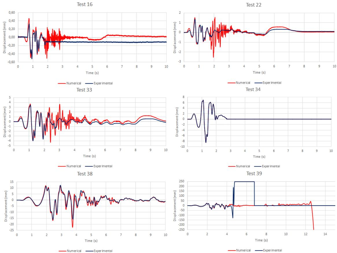
Fig. 18 Comparison of the time histories of the horizontal displacements at the top of the arch
