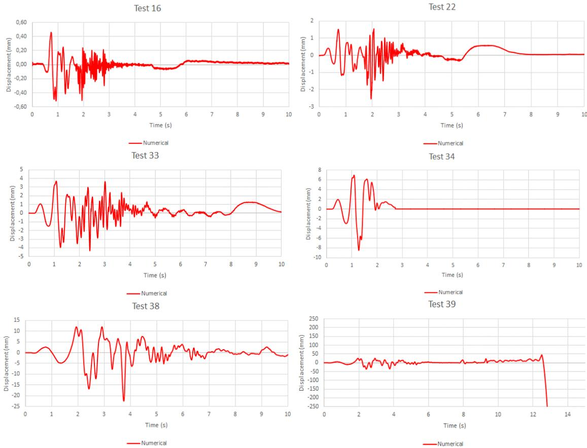
Fig. 17 Time histories of the horizontal displacements at the top of the arch
