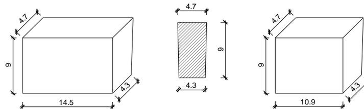
Fig. 7 Dimensions of the stone elements (cm)
