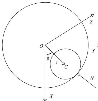
Fig. 1 Schematic view of buckled pipe
