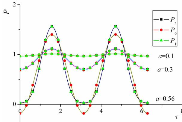
Fig. 3 Variations of the “reference” and approximate force  $P$  with  $a$
