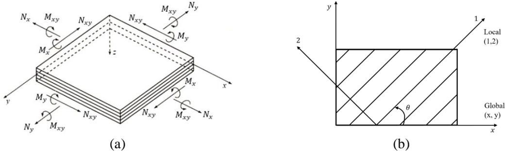
Fig. 1 Scheme of the laminate with loads and the lamina: (a) Laminate with forces and moments, (b) Unidirectional lamina and its axes: material/local (1, 2) and global (x, y)
