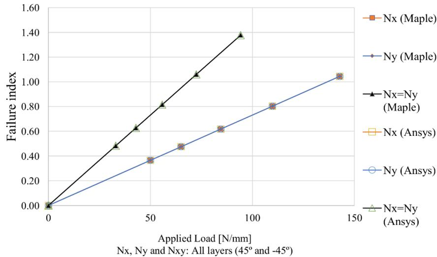
Fig. 9 Comparison of the evolution of (Maximum Stress criterion failure index between analytical (MAPLE®) and numerical (ANSYS® APDL) for laminate E3 ( $[45^\circ/-45^\circ]_S$ , Glass/epoxy)
