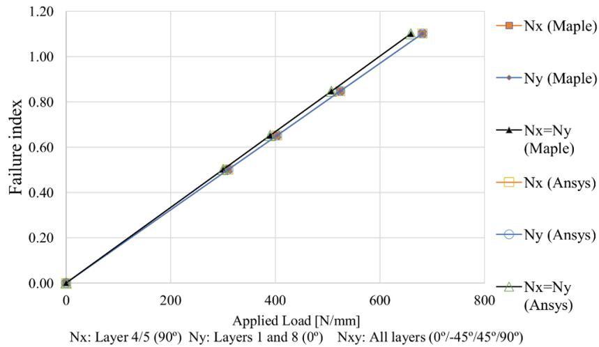
Fig. 13 Comparison of the evolution of Maximum Stress criterion failure index between analytical (MAPLE®) and numerical (ANSYS® APDL) for laminate E5 ( $[0^\circ/-45^\circ/45^\circ/90^\circ]_s$ , G4-800/5260)
