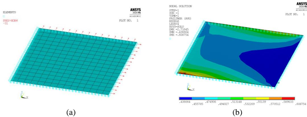
Fig. 6 (a) Representation of the mesh, supports and loads generated in 2D, for biaxial loading  $N_x = N_y$ , (b) Illustration of the index failure obtained in the worst ply of the composite for a load of 31 N/mm, for biaxial loading  $N_x = N_y$ , case E2, layer 4 ( $30^\circ$ ), using Tsai-Wu failure criterion
