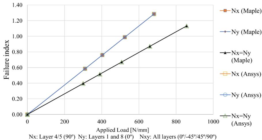
Fig. 12 Comparison of the evolution of Tsai-Wu criterion failure index between analytical (MAPLE®) and numerical (ANSYS® APDL) for laminate E5 ( $[0^\circ/-45^\circ/45^\circ/90^\circ]_s$ , G4-800/5260)
