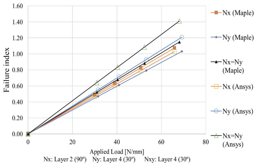
Fig. 7 Comparison of the evolution of Maximum Stress criterion failure index between analytical (MAPLE®) and numerical (ANSYS® APDL) for laminate E2 ( $[30^\circ / 90^\circ / -30^\circ / 30^\circ]$ , Glass/epoxy)
