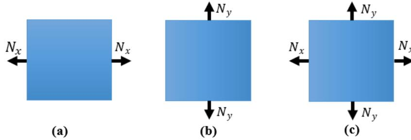
Fig. 2 Plates' loads considered. (a) Uniaxial tension along  $x$ ,  $N_x$ , (b) Uniaxial tension along  $y$ ,  $N_y$  and (c) Biaxial tension  $N_x$  and  $N_y$
