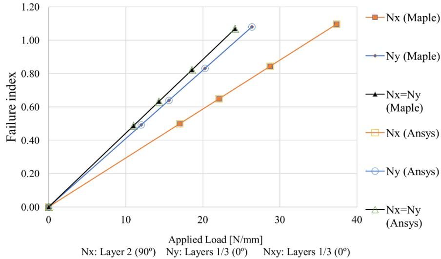
Fig. 11 Comparison of the evolution of Maximum Stress criterion failure index between analytical (MAPLE®) and numerical (ANSYS® APDL) for laminate E4 ( $[0^\circ/90^\circ/0^\circ]$ , Glass/epoxy)
