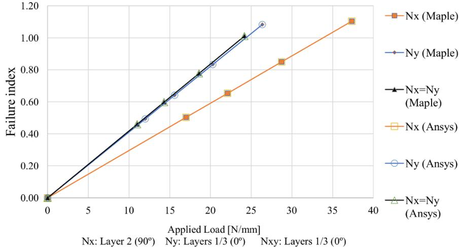
Fig. 10 Comparison of the evolution of Tsai-Wu criterion failure index between analytical (MAPLE®) and numerical (ANSYS® APDL) for laminate E4 ( $[0^\circ/90^\circ/0^\circ]$ , Glass/epoxy)
