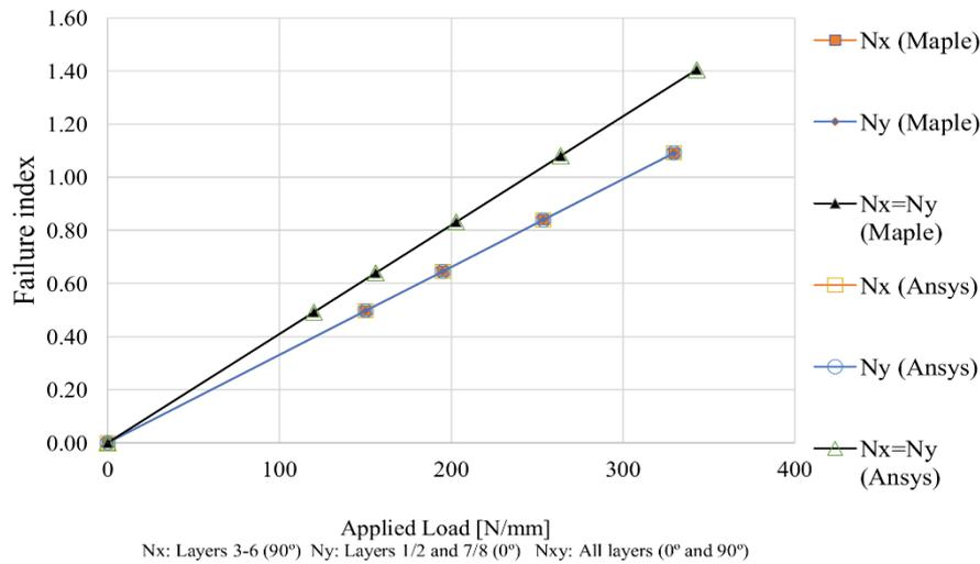
Fig. 4 Comparison of the evolution of Maximum Stress criterion failure index between analytical (MAPLE®) and numerical (ANSYS® APDL) for laminate E1 ( $[0^{\circ}_2/90^{\circ}_2]_S$ , AS4/3501-6)
