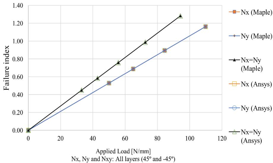
Fig. 8 Comparison of the evolution of Tsai-Wu criterion failure index between analytical (MAPLE®) and numerical (ANSYS® APDL) for laminate E3 ( $[45^\circ/-45^\circ]_S$ , Glass/epoxy)
