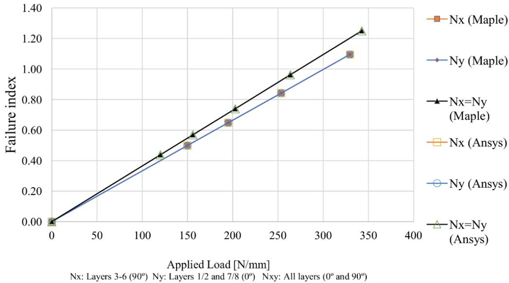
Fig. 3 Comparison of the evolution of Tsai-Wu criterion failure index between analytical (MAPLE®) and numerical (ANSYS® APDL) for laminate E1 ( $[0^{\circ}_2/90^{\circ}_2]_S$ , AS4/3501-6)
