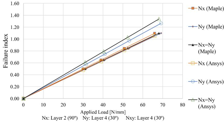
Fig. 5 Comparison of the evolution of Tsai-Wu criterion failure index between analytical (MAPLE®) and numerical (ANSYS® APDL) for laminate E1 ( $[30^\circ/90^\circ/-30^\circ/30^\circ]$ , Glass/epoxy)
