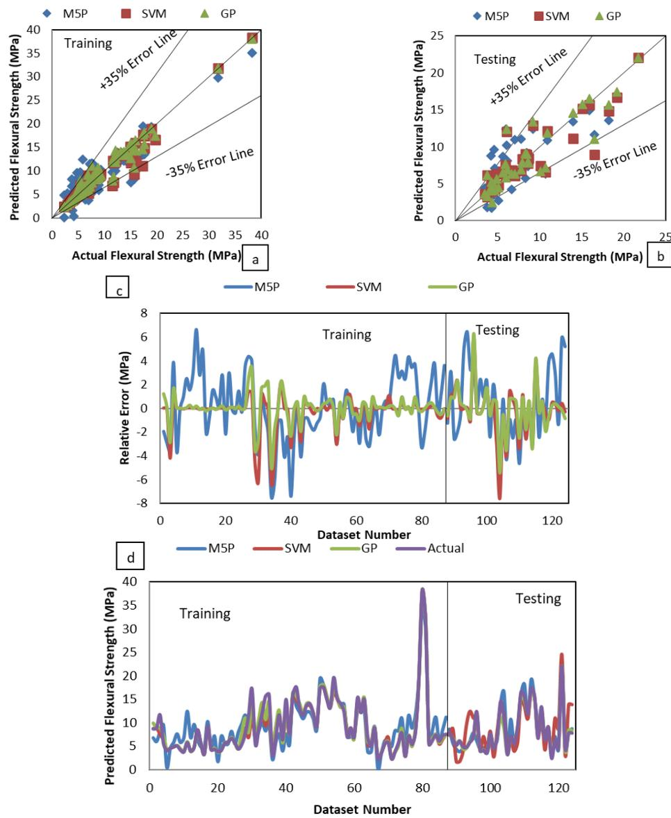
Fig. 4 Comparison between M5P, SVM and GP, predicted and actual values for Flexural Strength
