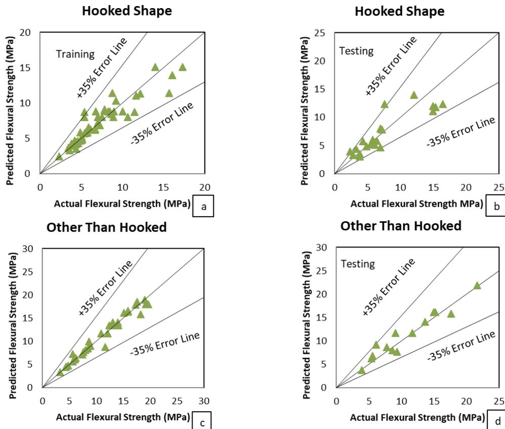
Fig. 5 Comparison between predicted and actual values for Flexural Strength on the Basis of Shape by GP technique
