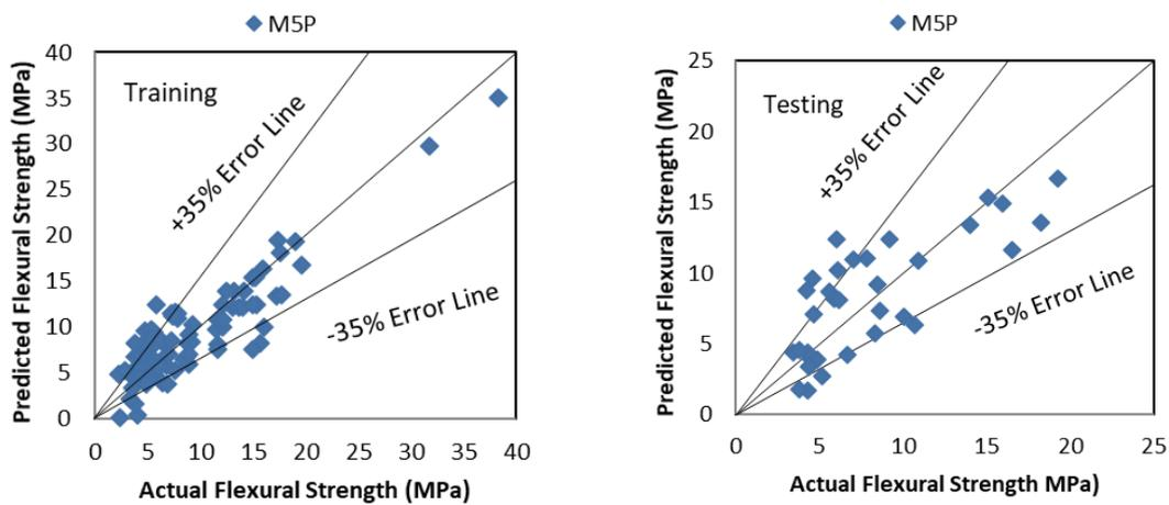
Fig. 1 Agreement plot between observed and predicted flexural strength of training and testing dataset by M5P technique
