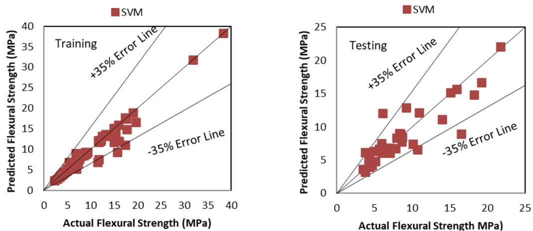
Fig. 2 Agreement plot between observed and predicted flexural strength of training and testing dataset by SVM technique
