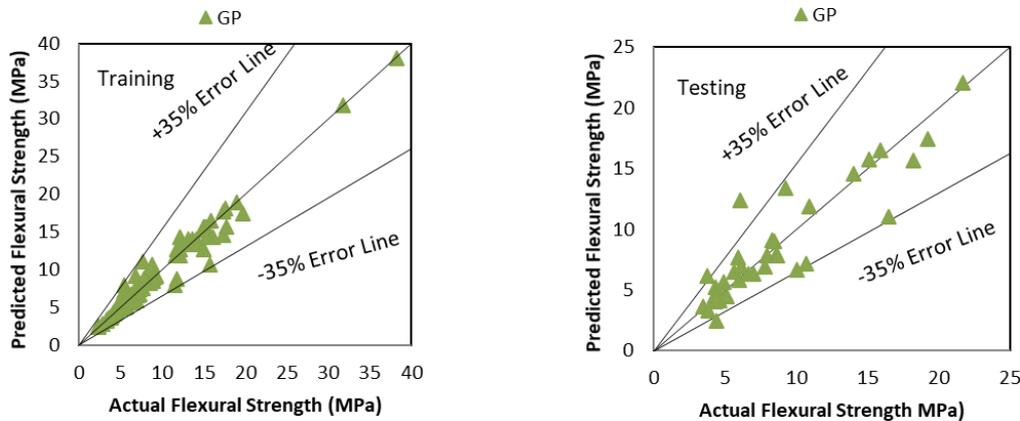
Fig. 3 Agreement plot between observed and predicted flexural strength of training and testing dataset by GP technique
